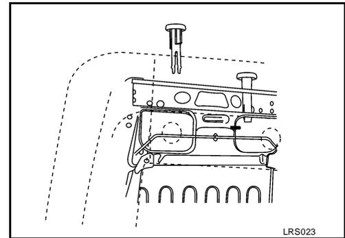
5. Remove the snap ring and the lumbar support lever knob.
