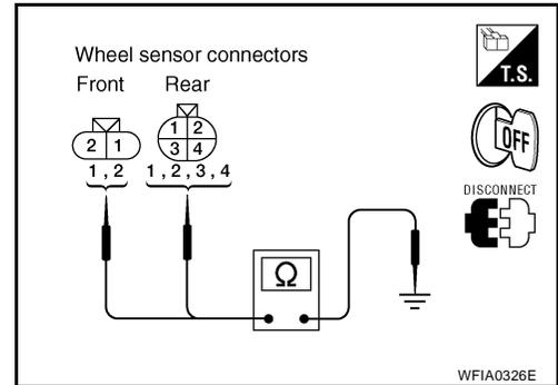
**6. CHECK WIRING HARNESS FOR OPEN CIRCUIT**
