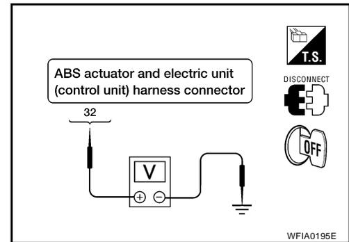
2. Check resistance between ABS actuator and electric unit (control unit) harness connector E125 and body ground.
