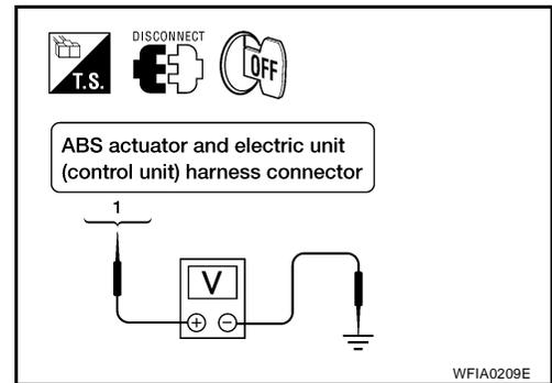
2. Check resistance between ABS actuator and electric unit (control unit) connector E125 and body ground.
