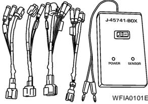
Checking operation of ABS active wheel sensors                                          |
