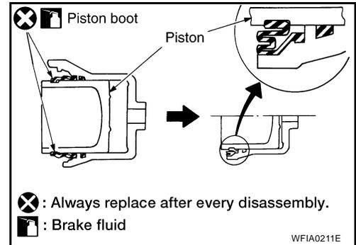
4. Insert into cylinder body by hand and insert piston boot piston-side lip into piston groove.
