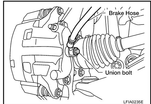
6. Refill new brake fluid and bleed air. Refer to [BR-12, "Bleeding Brake System"](#) .
