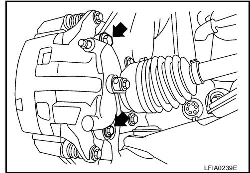
5. Install brake hose to cylinder body, if removed, then tighten union bolt to the specified torque. Refer to [BR-24, "Components"](#) .
