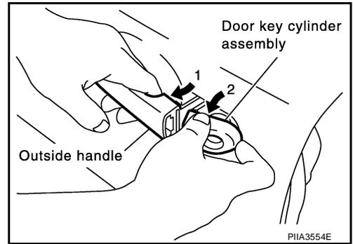
5. While pulling outside handle, slide toward rear of vehicle to remove outside handle.
