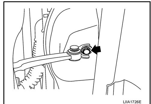
4. Remove the door-side hinge nuts, and the door assembly.
