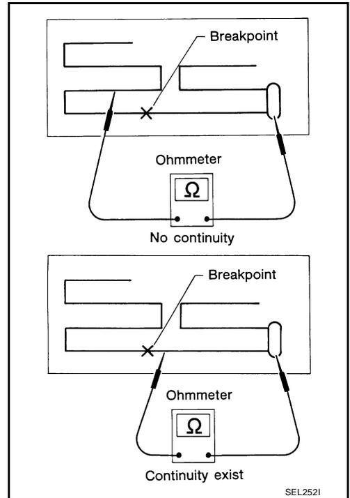
3. To locate a break, move probe along element. Tester indication will change abruptly when probe passes the broken point.
