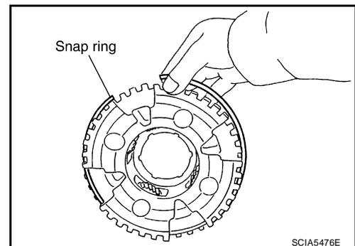
4. Disassemble input clutch assembly.
