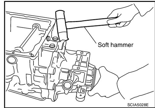
iii. Remove rear extension assembly from transmission case. (With needle bearing.)
