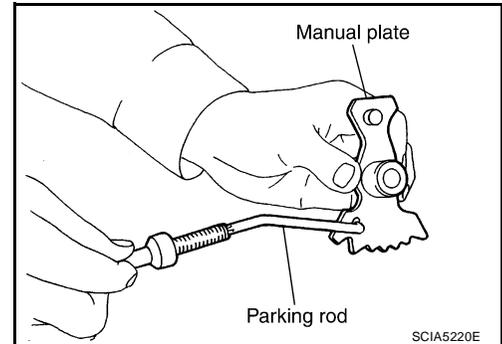
64. Remove manual shaft from transmission case.
