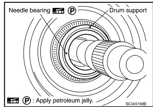
36. Install high and low reverse clutch assembly in direct clutch.
