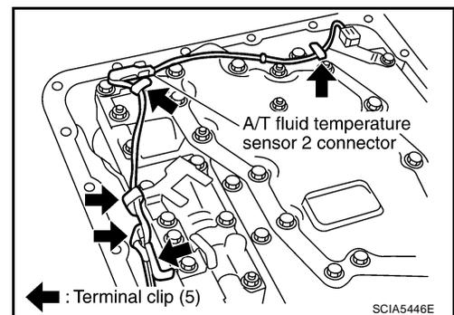
33. Straighten terminal clips to free revolution sensor harness.
