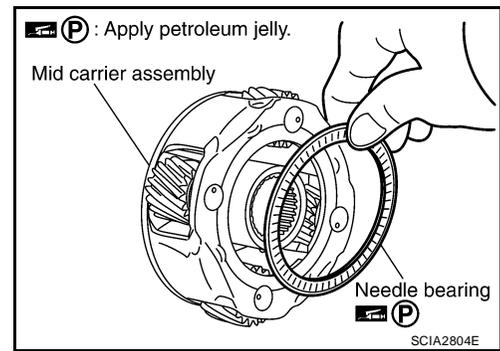
43. Install needle bearing (front side) to mid carrier assembly.
