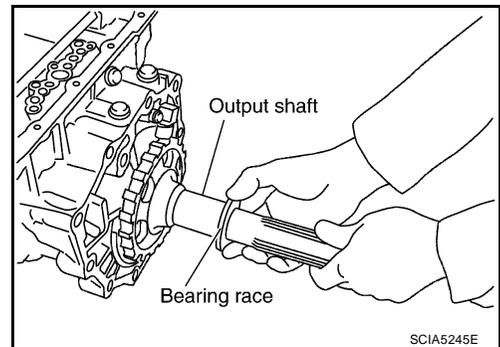
45. Remove output shaft from transmission case by rotating left/right.
