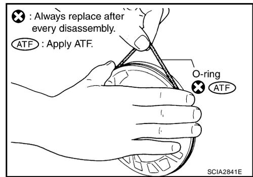
4. Remove O-ring from oil pump cover.
