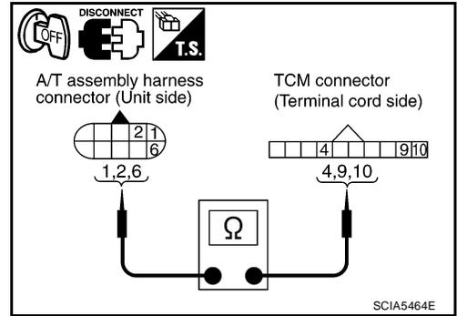
4. Check continuity between A/T assembly harness connector terminals and TCM connector terminals.
