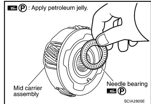
44. Install mid carrier assembly in rear carrier assembly.
