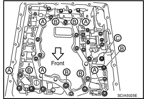
36. Remove control valve with TCM from transmission case.
