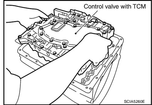
37. Remove A/T fluid temperature sensor 2 with bracket from control valve with TCM.
