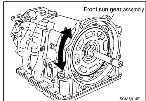
50. Install needle bearing to front sun gear.
