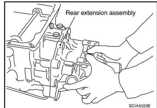
iii. Tighten rear extension assembly mounting bolts to specified torque.
