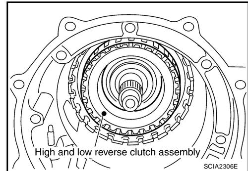
37. Using a flat-bladed screwdriver, align the drive plate.
