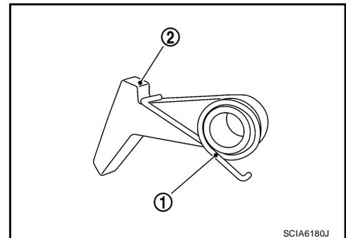
26. Install parking pawl (with return spring) and pawl shaft to rear extension (2WD models) or adapter case (4WD models).
