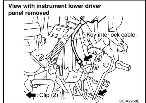
4. Insert interlock rod into adjuster holder.
