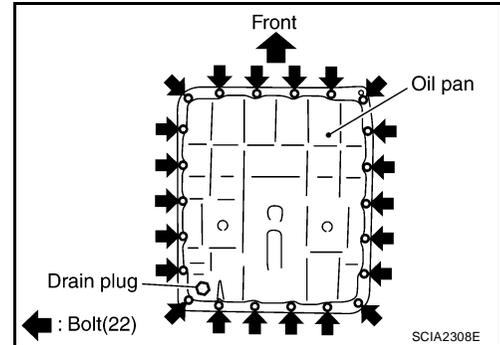
3. Check for foreign materials in oil pan to help determine cause of malfunction. If the A/T fluid is very dark, has some burned smell, or contains foreign particles then friction material (clutches, band) may need replacement. A tacky film that will not wipe clean indicates varnish build up. Varnish can cause valves, servo, and clutches to stick and can inhibit pump pressure.
