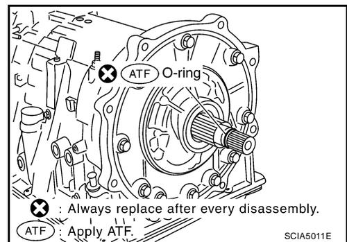
7. Install converter housing to transmission case.
