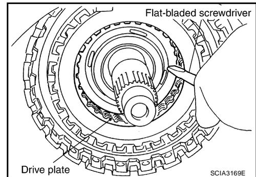
38. Install high and low reverse clutch hub, mid sun gear assembly and rear sun gear assembly as a unit.
