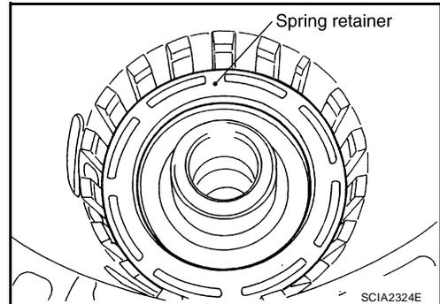
17. Set the SST on spring retainer and install snap ring (fixing spring retainer) in transmission case while compressing return spring.
