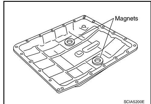
17. Install oil pan to transmission case.
