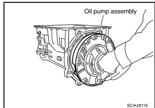
4. Apply recommended sealant (Genuine RTV Silicone Sealant or equivalent. Refer to [GI-45, "Recommended Chemical Products and Sealants"](#) .) to oil pump assembly as shown in the figure.
