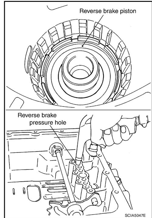
59. Remove D-rings from reverse brake piston.
