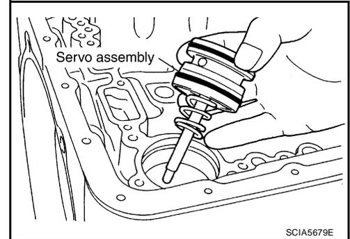
69. Remove return spring from servo assembly.
