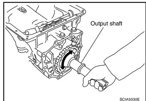
46. Remove parking gear from output shaft.
