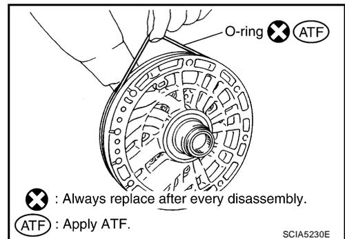
2. Install O-ring to oil pump housing.
