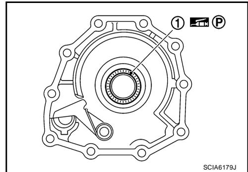
29. Install seal rings to output shaft.
