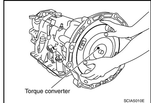
3. Check torque converter one-way clutch using a check tool as shown at figure.
