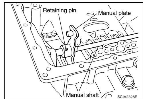
61. Remove manual shaft retaining pin with a pair of nippers.
