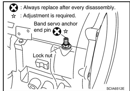
48. Install brake band in transmission case.
