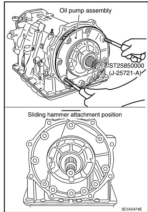
8. Remove O-ring from oil pump assembly.
