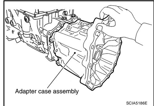
iii. Tighten adapter case assembly mounting bolts (1) to specified torque. (With terminal bracket (2).)
