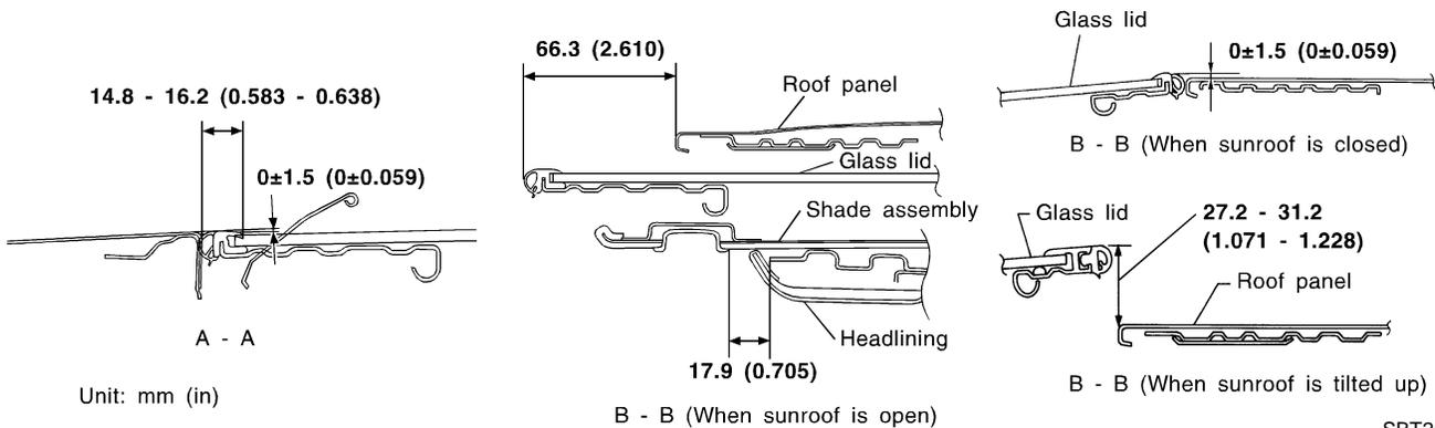
If any gap or height difference between glass lid and roof is found, check glass lid fit and adjust as follows:
