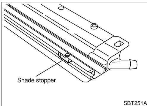
**D** Remove shade stoppers (2 points) from rear end of sunroof frame assembly. Remove sun shade from rear end of sunroof frame assembly.
