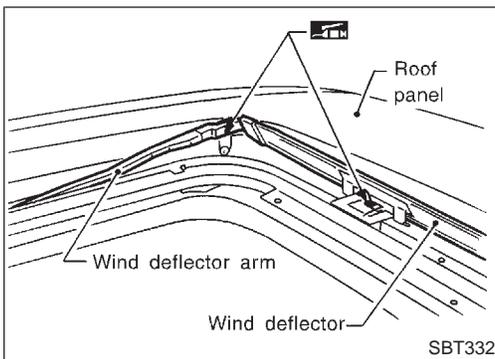
4. Check that wind deflector is properly retracted by hand. If it is not, remove and visually check condition. (Refer to removal procedures, BT-52.) If wind deflector is damaged, replace with new one. If wind deflector is not damaged, re-install properly.
