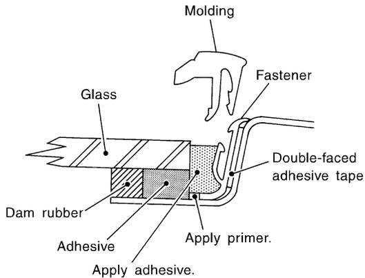
4. Install molding by aligning the molding mark located on center with vehicle center. Be sure to install tightly so that there is no gap around the corner.
