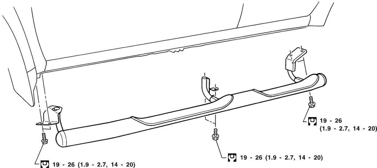
• Pipe type and board type outer steps are only different in shape. Removal and installation method for both types is the same.
