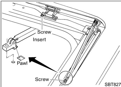
**B** Remove screws from left and right sides of each wind deflector holder. Extract pawls through rail holes, then remove left and right sides of wind deflector holder. Remove screws from front end of sunroof unit. Extract pawls through frame holes, then remove wind deflector from frame assembly.
