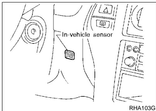
In-vehicle Sensor Circuit
