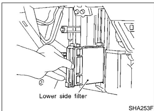
4. Take out the lower side In-cabin microfilter from cooling unit.
