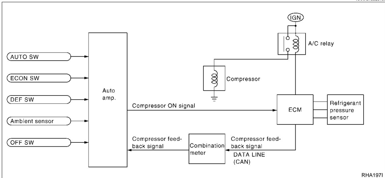
The ECM controls compressor operation using input signals from the throttle position sensor, refrigerant pressure sensor and auto amplifier.
