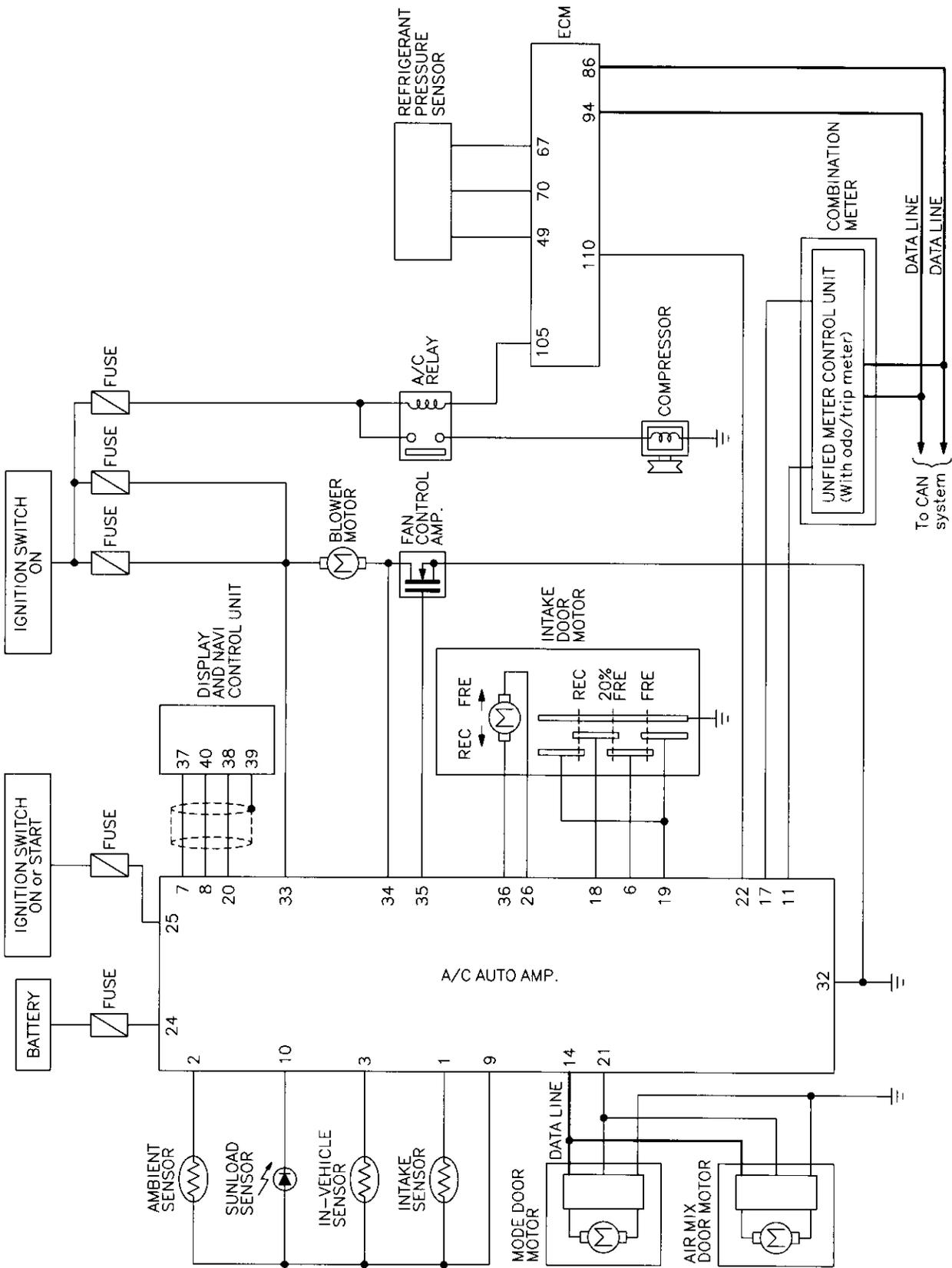
Wiring Diagram — A/C, A — (With Navigation System)
