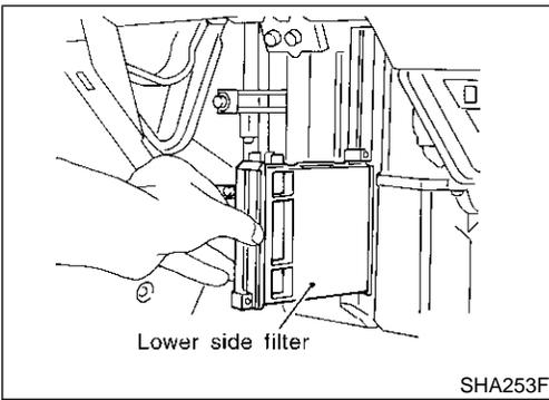
4. Take out the lower side In-cabin microfilter from cooling unit.
