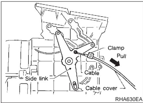
**CONTROL LINKAGE ADJUSTMENT****Mode Control Cable**
