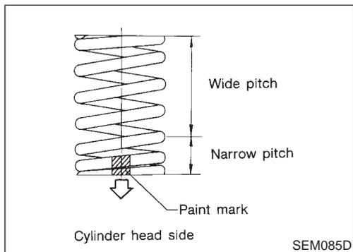
2. Install valve component parts.
