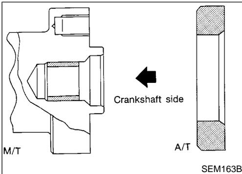
2. Install pilot bushing or pilot converter as shown.
