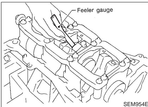
7. Measure connecting rod side clearance.
