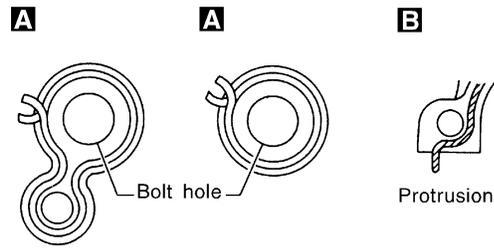
Sealant protrusion away from bolt hole
