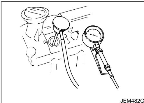
11. Attach a compression tester to No. 1 cylinder.
