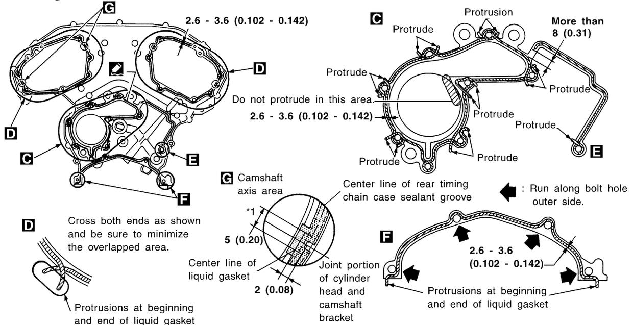
\*1: Apply liquid gasket to the chamfered surface between camshaft bracket and cylinder head.
