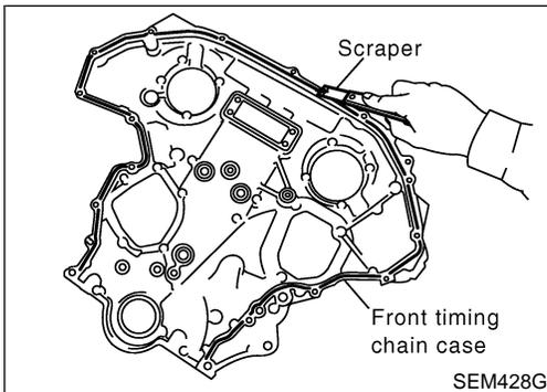
42. Use a scraper to remove all traces of liquid gasket from front and rear timing chain case, and opposite mating surfaces.
