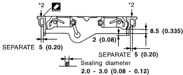
\*2: Remove the protruding sealant from front face.
