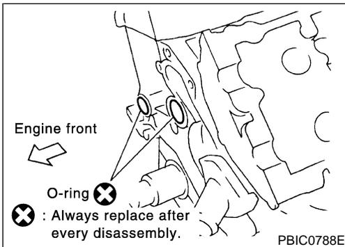
2. Install new O-rings to cylinder block if rear timing chain case is removed.
