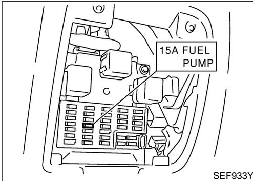
4. Disconnect fuel pump fuse to avoid injection during measurement.
