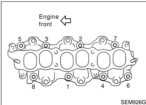
8. Remove intake manifold in reverse order of illustration.
