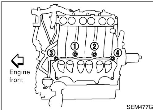
16. Remove lower intake manifold collector in reverse order of illustration.
