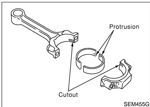
5. Install connecting rod bearings in connecting rods and connecting rod caps.
