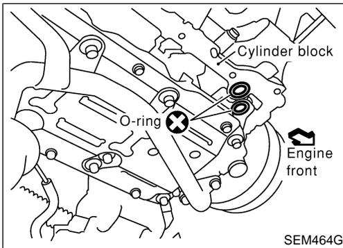
6. Install O-rings, cylinder block and oil pump body.
