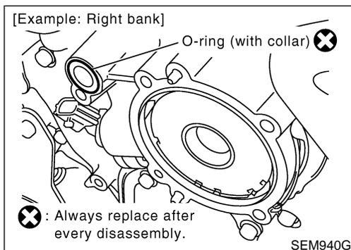
17. Install the water pump cover and the chain tensioner cover to front timing chain case if removed.
