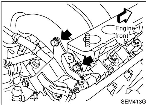
15. Remove intake manifold collector support bolts.
