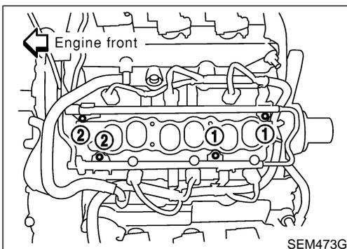
17. Disconnect injector harness connectors.
