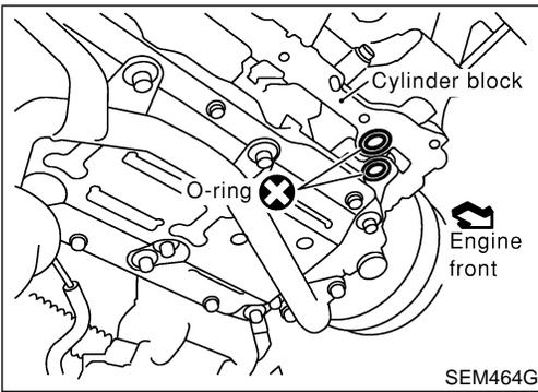
33. Remove O-rings from cylinder block and oil pump body.
