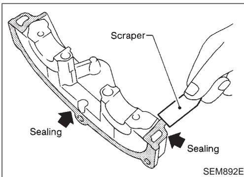
2. Before installing camshaft bracket, remove old liquid gasket from mating surface using a scraper.
