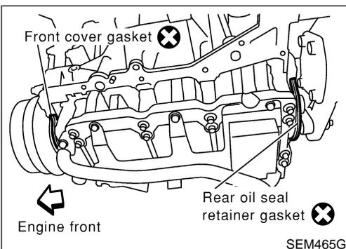
3. Install front cover gasket and rear oil seal retainer gasket.
