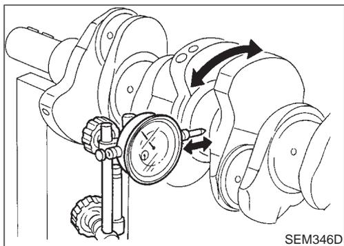
3. Measure crankshaft runout.
