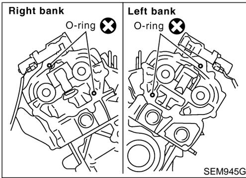
39. Remove O-rings from cylinder head.
