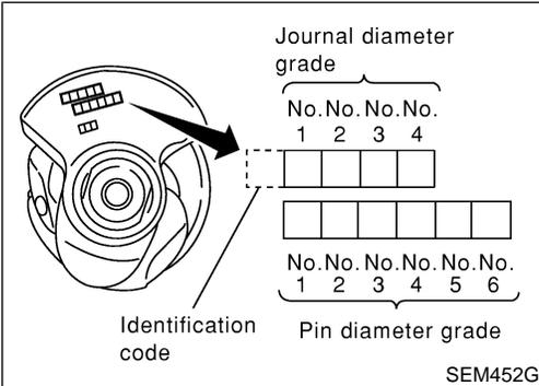
8. If crankshaft is replaced with a new one, select connecting rod bearing according to the following table.
