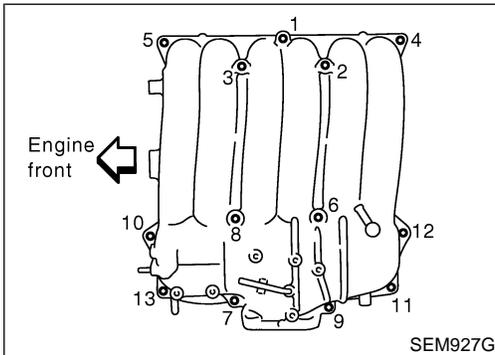
14. Remove upper intake manifold collector in reverse order of illustration.
