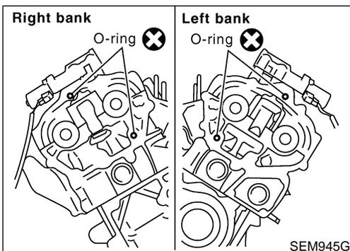
3. Install new O-rings to cylinder head if rear timing chain case is removed.
