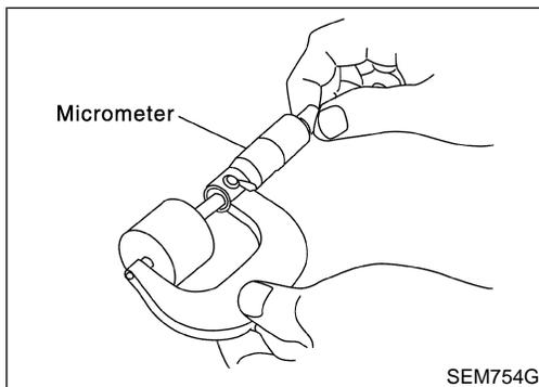
3. Measure center thickness of removed valve lifter with micrometer.
