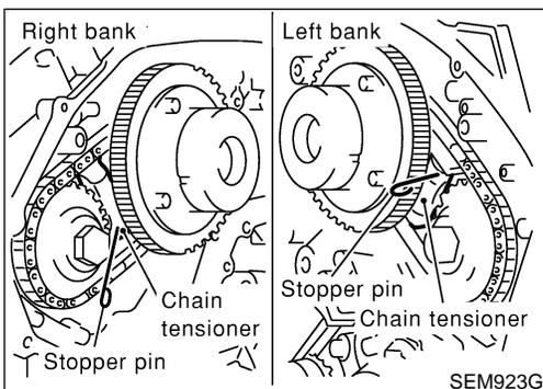
35. Attach a suitable stopper pin to RH and LH camshaft chain tensioners.
