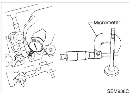
2. If it exceeds the limit, check valve to valve guide clearance.
