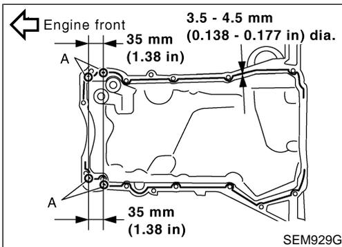
5. Apply liquid gasket to inner sealing surface as shown in figure.
