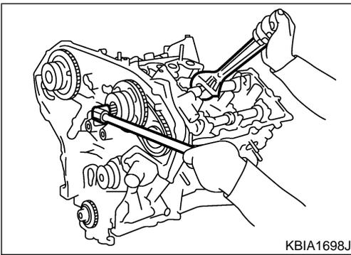
36. Remove intake and exhaust camshaft sprocket bolts.
