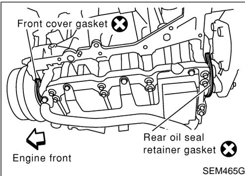
34. Remove front cover gasket and rear oil seal retainer gasket.
