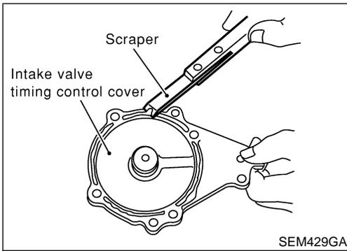
45. Use a scraper to remove all traces of liquid gasket from intake valve timing control cover, water pump cover and chain tensioner cover.
