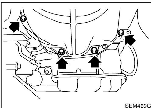
9. Install the four engine-to-transmission bolts. For tightening torque, refer to AT-277 or MT-8, "Installation".
