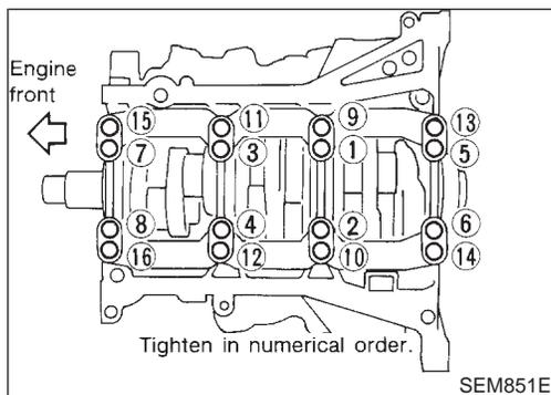
3. After installing crankshaft, main bearing cap, main bearing beam and bearing cap bolts, tighten bearing cap bolts in numerical order as shown.
