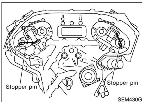
5. Align rear timing chain case, if removed, with dowel pins (RH and LH) on cylinder block. Then install it.
