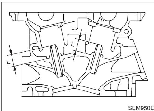
4. Heat cylinder head to 110 to 130°C (230 to 266°F) and press service valve guide onto cylinder head.
