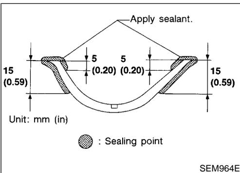
2. Apply sealant to front cover gasket and rear oil seal retainer gasket.
