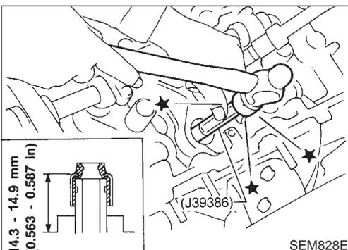
6. Apply engine oil to new valve oil seal and install it with Tool.
