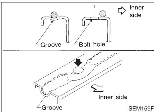
4. Apply a continuous bead of liquid gasket to mating surface of aluminum oil pan.
