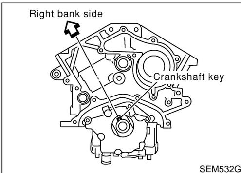
3. Before installing the cylinder head gasket, be sure that No. 1 cylinder is at TDC.
