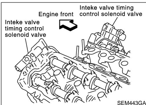
10. Remove intake valve timing control solenoid valves.
