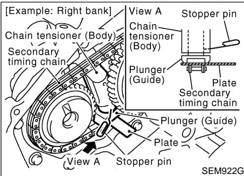
37. Remove secondary timing chains with camshaft sprockets.
