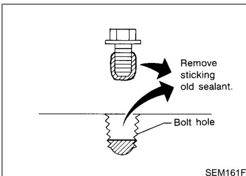
● **Remove old liquid gasket from the bolt hole and thread.**
