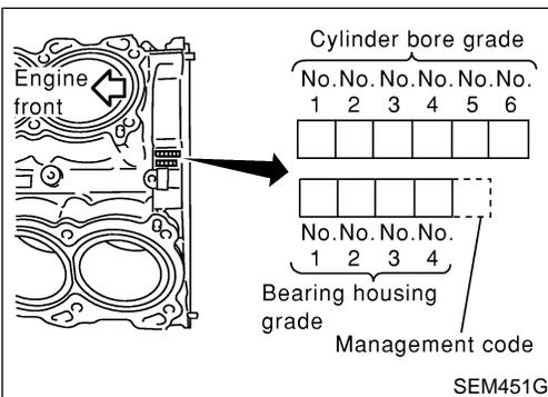
6. If crankshaft or cylinder block is replaced with a new one, select thickness of main bearings as follows:
