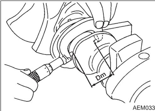
4. Measure outer diameters "Dm" of each crankshaft main journal.
