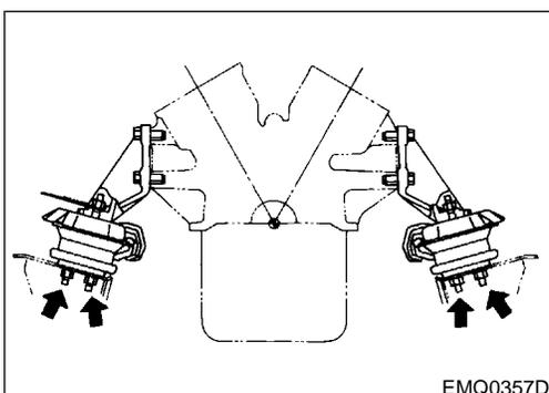
22. Remove front engine mounting nuts from both sides.
