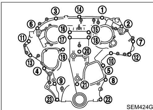
28. Remove front timing chain case bolts.
