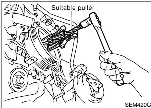
24. Remove crankshaft pulley with a suitable puller.
