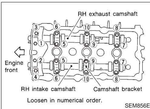
11. Remove intake and exhaust camshafts and camshaft brackets.
