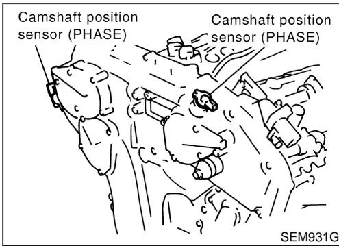
13. Remove camshaft position sensors (PHASE).
