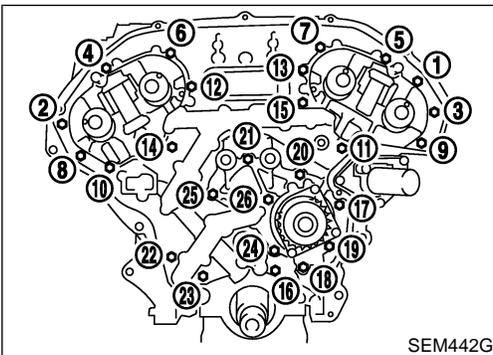
38. Remove rear timing chain case as follows if necessary.
