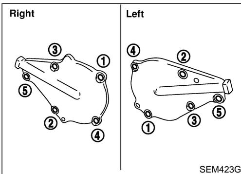
27. Remove intake valve timing control covers.
