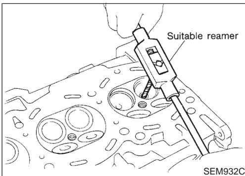
3. Ream cylinder head valve guide hole.
