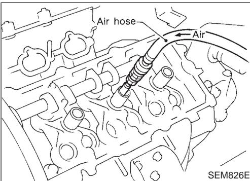
Remove spark plug, then install air hose adapter into spark plug hole and apply air pressure to hold valves in place. Apply a pressure of 490 kPa (5 kg/cm<sup>2</sup>, 71 psi).
