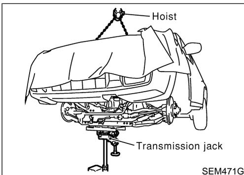
21. Set a suitable transmission jack under the front suspension member and hoist engine with engine slingers.
