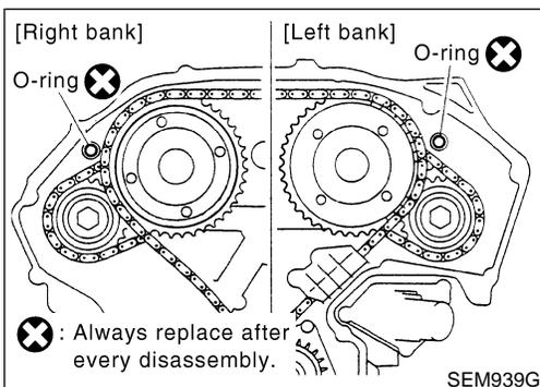
16. Install O-rings on rear timing chain case.
