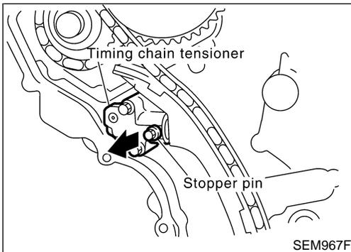
15. Install timing chain tensioner, then remove the stopper pin.
