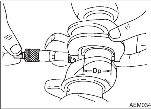
4. Measure outer diameter "Dp" of each crankshaft pin journal.
