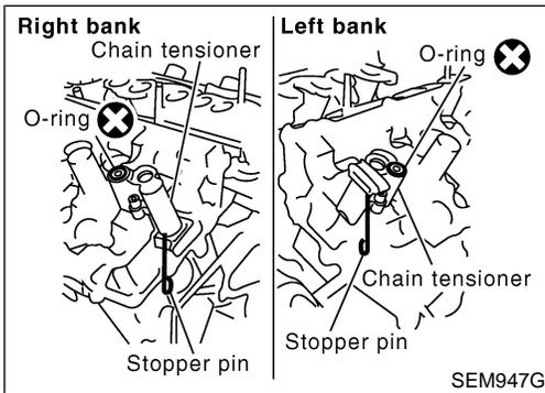
13. Remove RH and LH camshaft chain tensioners from cylinder head.
