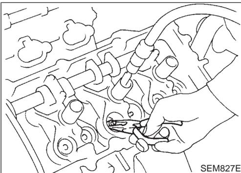
5. Remove valve oil seal.
