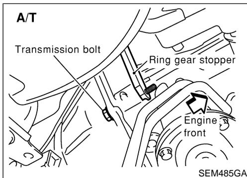
22. Remove starter motor, and set ring gear stopper using the mounting bolt hole.
