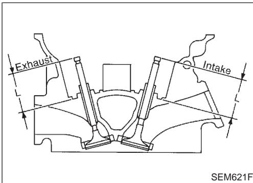
8. Use a depth gauge to measure the distance between the mounting surface of the cylinder head spring seat and the valve stem end. If the distance is shorter than specified, repeat step 5 above to adjust it. If it is longer, replace the valve seat with a new one.
