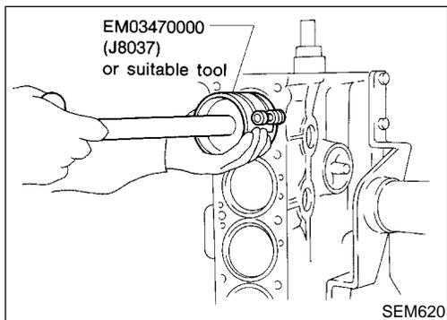
6. Install pistons with connecting rods.
