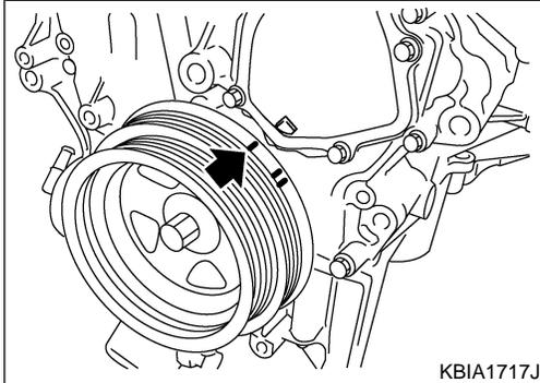
21. Set No. 1 piston at TDC on the compression stroke by rotating crankshaft.
