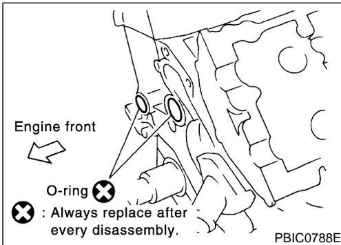
40. Remove O-rings from cylinder block.
