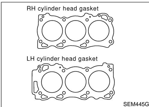
4. Install cylinder heads with new gaskets.
