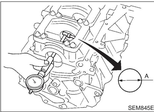
2. Install main bearing cap and bearing beam to cylinder block. **Tighten all bolts in correct order.**
