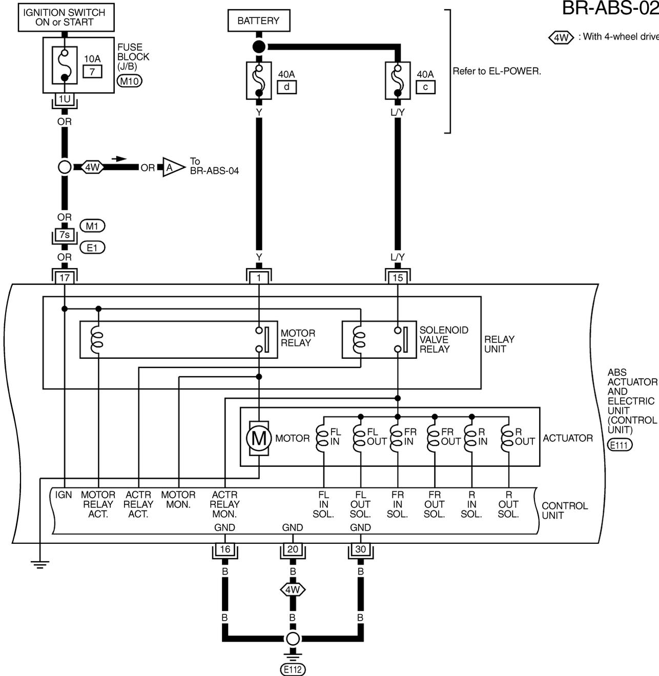
ABS ACTUATOR AND ELECTRIC UNIT (CONTROL UNIT) (E11)
