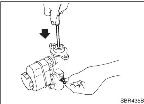
5. Install piston stopper while piston is pushed into cylinder.
