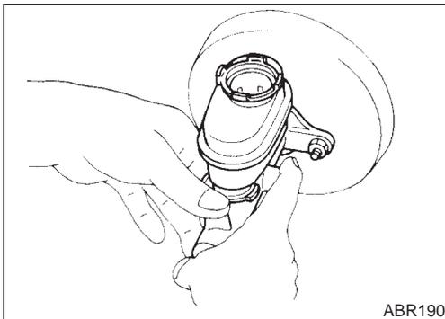
3. Install the plate and the guide into the cylinder body.
