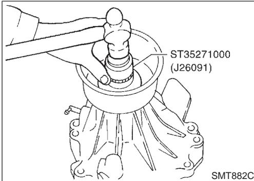
12. Apply ATF to the circumference of new rear oil seal, and tap it using a drift as shown in the figure so that it is aligned with case tip face.
