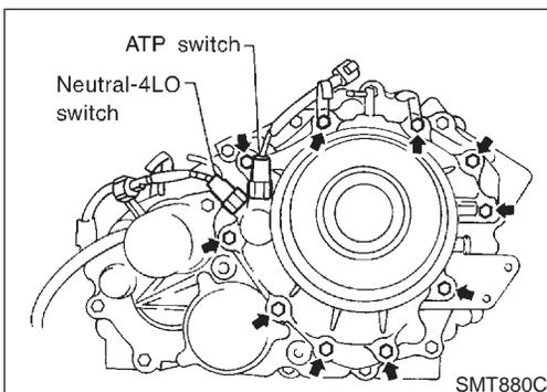
15. Remove all the gasket fluid from switch mounting area and inside rear case, with ATP switch and neutral-4LO switch threaded in 1 to 2 pitches, apply Genuine Thread Sealant or equivalent to the thread of the switches and tighten it to specified torque.
