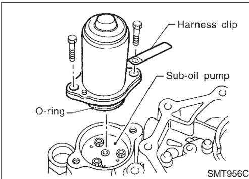
5. Apply ATF or petroleum jelly to new O-ring and install it to transfer motor.
