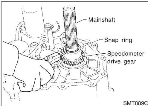
2. Check speedometer drive gear teeth for abnormal wear. Set speedometer drive gear properly on mainshaft, and secure it with snap ring.
