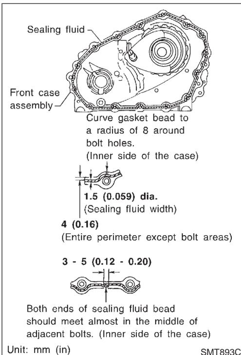
3. Apply Genuine Anaerobic Liquid Gasket or equivalent to the entire center case mounting surface of front case as shown in the figure. Refer to TF-151.
