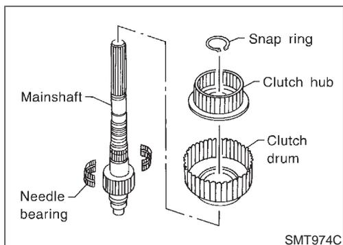
5. Install clutch drum, needle bearing and clutch hub to mainshaft, and secure them with snap ring.
