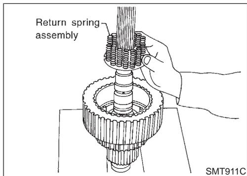
7. Align the notch of return spring assembly with the pin of clutch hub, and install it.
