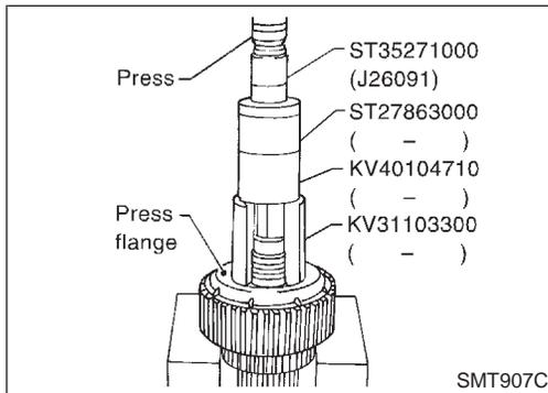
5. Set a drift (KV31103300), a support ring (KV40104710), a support ring (ST27863000) and a drift (ST35271000) to press flange as shown in the figure. Press drift until snap ring is out of place.
