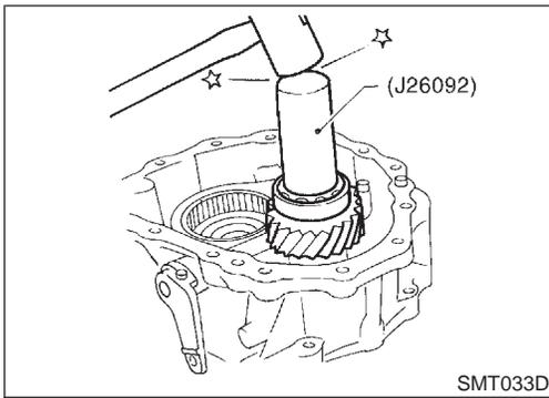
2. Select counter gear rear bearing shim.
