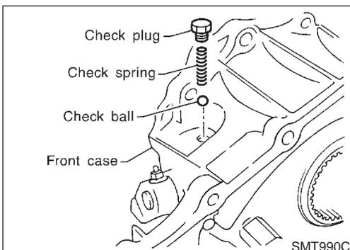
4. Remove all the liquid gasket on check plug and front case, and install check ball and check spring to front case. Apply Genuine Thread Sealant or equivalent\* to check plug, install it to front case, and tighten it to specified torque.
