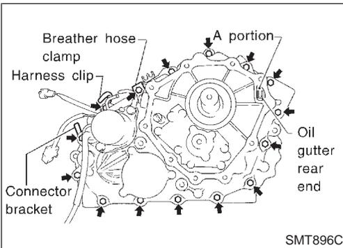
7. Make sure oil gutter rear end protrudes from point "A" in the figure.
