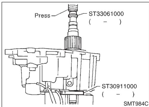
15. Place puller (ST30911000) to mainshaft rear bearing inner race, and set it to press stand.
