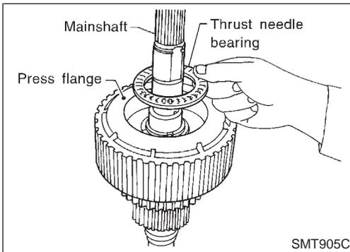
12. Install thrust needle bearing to press flange.
