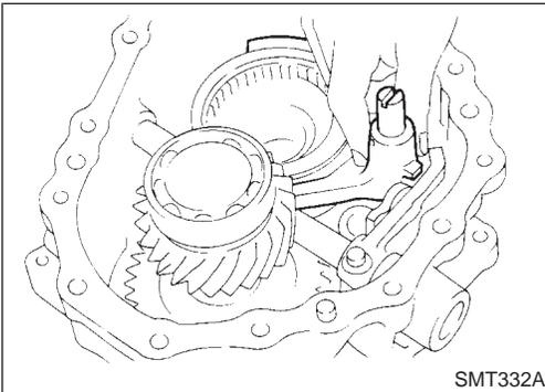
h. Install L & H shift rod and fork assembly with coupling sleeve.
