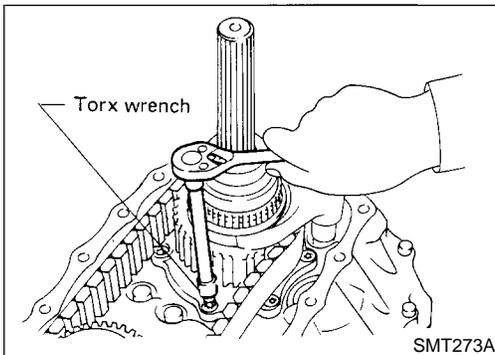
7. Remove bolts securing bearing retainer.
