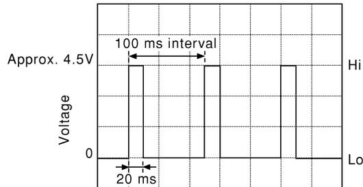
② ABS waveform during operation
