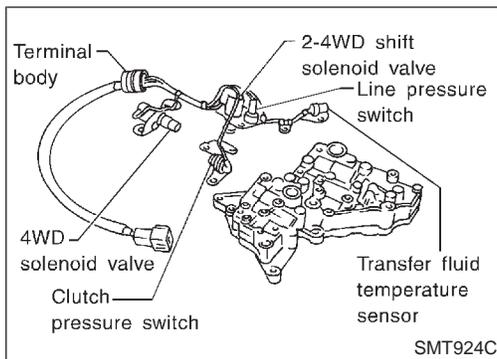
7. Remove 4WD solenoid valve, clutch pressure switch, 2-4WD shift solenoid valve, line pressure switch, and transfer fluid temperature sensor from control valve assembly.
