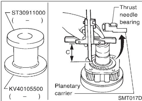
8. Set a support (KV40105500) to bushing replacer puller (ST30911000) as shown in the figure, and place planetary carrier on it.
