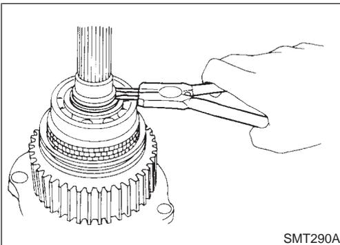
3. Remove snap ring and spacer.
