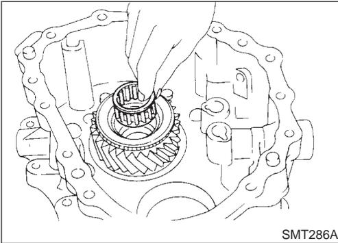
f. Remove needle bearing from main gear.
