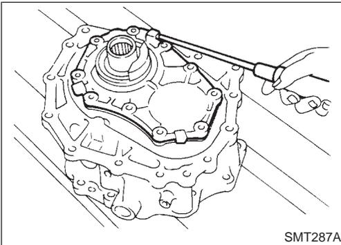
g. Remove bolts securing front case cover and then remove case.
