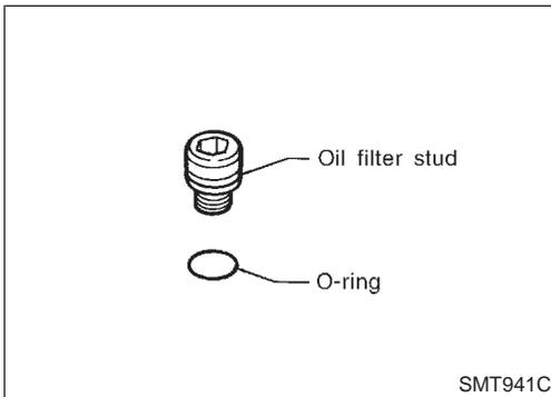
5. Remove O-ring from oil filter stud.
