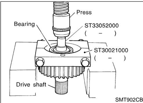
4. Set the puller (ST30021000) and the adapter (ST33052000). Remove front drive shaft rear bearing.
