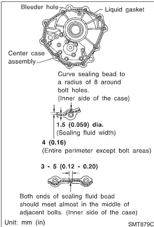
13. Apply Genuine Anaerobic Liquid Gasket or equivalent to entire rear case mounting surface of center case as shown in the figure. Refer to TF-151.
