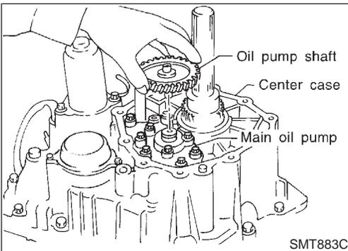
9. Fit double-flat end of oil pump shaft into slot of main oil pump and install it.
