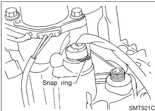
11. Secure terminal body with snap ring.
