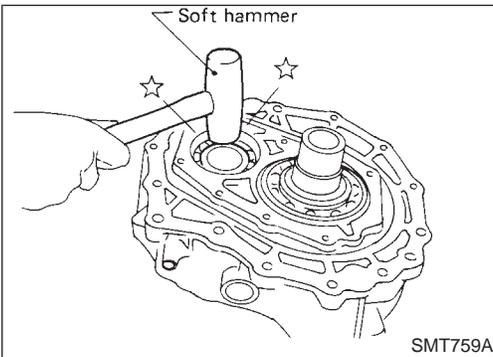
h. Remove counter gear by tapping lightly.
