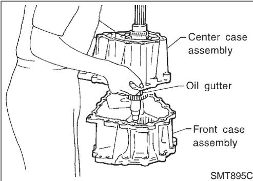
5. With the claws of oil gutter held by a finger, install center case assembly to front case assembly.
