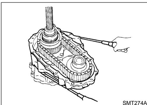
8. Remove bolts securing center case to front case and then separate center case and front case.
