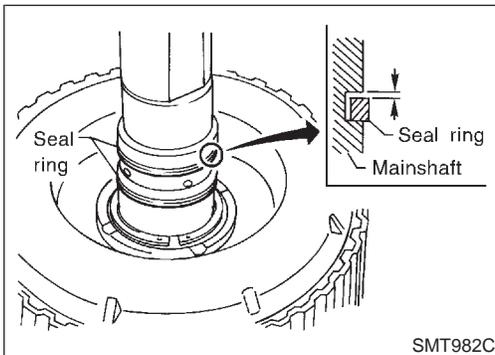
13. Apply petroleum jelly to new seal rings, and install them to mainshaft. Measure clearance between seal ring and groove using feeler gauge.
