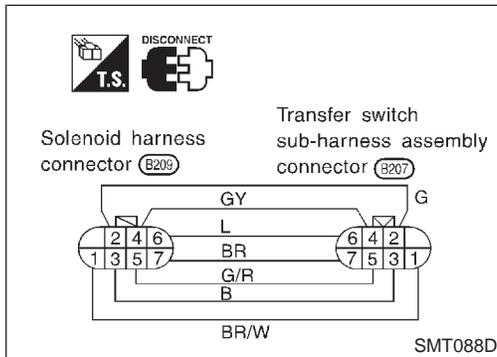
TRANSFER TERMINAL CORD ASSEMBLY SUB-HARNESS CONNECTOR
