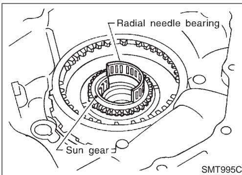
20. Apply petroleum jelly to radial needle bearing, and install it inside sun gear.
