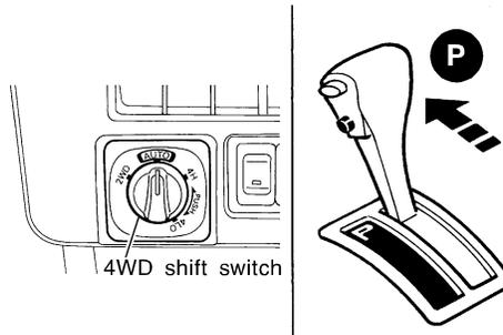
3. While shifting from "4H" to "4LO", does 4WD shift indicator lamp turn OFF and ATP warning lamp turn ON?
