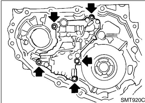
10. Install control valve assembly to center case, and tighten bolts.
