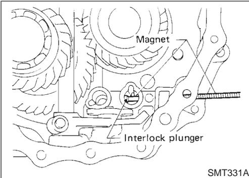
g. Insert interlock plunger into front case.
