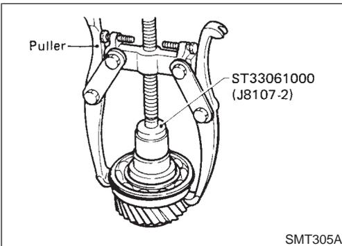
2. Pull out main gear bearing.
