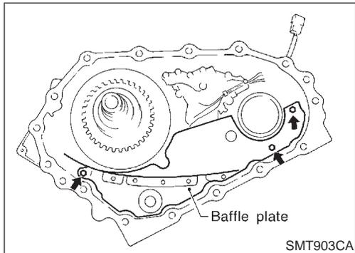
17. Install baffle plate to center case, and tighten bolts.
