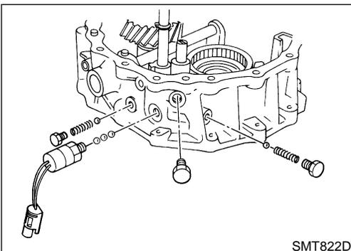
j. Install neutral position switch, check balls, check springs and plugs.
