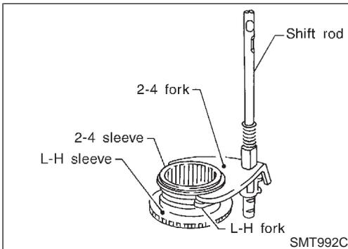
2. Install 2-4 sleeve and L-H sleeve to each fork.
