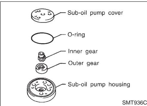
5. Remove sub-oil pump cover, outer gear, inner gear and O-ring from sub-oil pump housing.
