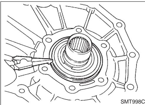
4. Remove snap ring from main gear bearing.
