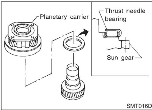
6. Install thrust needle bearing to sun gear.
