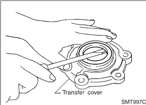
3. Remove oil seal from transfer cover.
