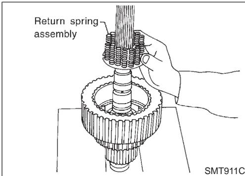
9. Remove return spring assembly from clutch hub.
