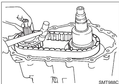
3. Install drive chain temporarily to front drive shaft and drive gear of clutch drum.
