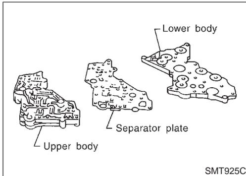
9. Place control valve with lower body facing up, remove two mounting bolts, and then remove lower body and separator plate from upper body.
