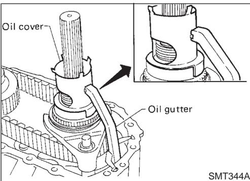
8. Install oil gutter and oil cover.
