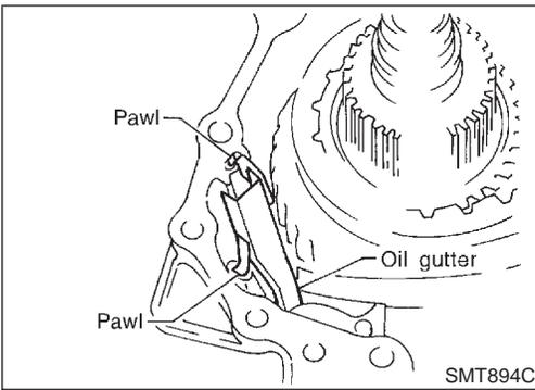
4. Make sure the two claws of oil gutter are securely attached to slots in center case.
