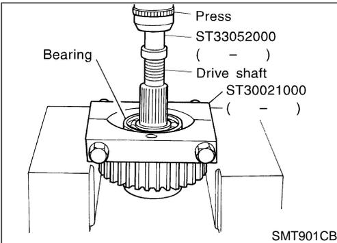
3. Set a puller (ST30021000) and an adapter (ST33052000). Remove front drive shaft front bearing.
