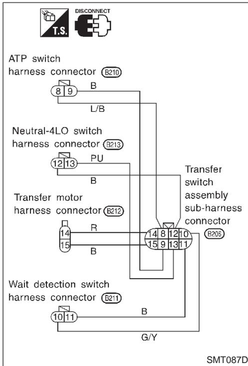
TRANSFER SWITCH ASSEMBLY SUB-HARNESS CONNECTOR
