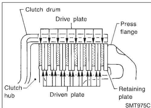
6. Install each clutch to clutch drum.
