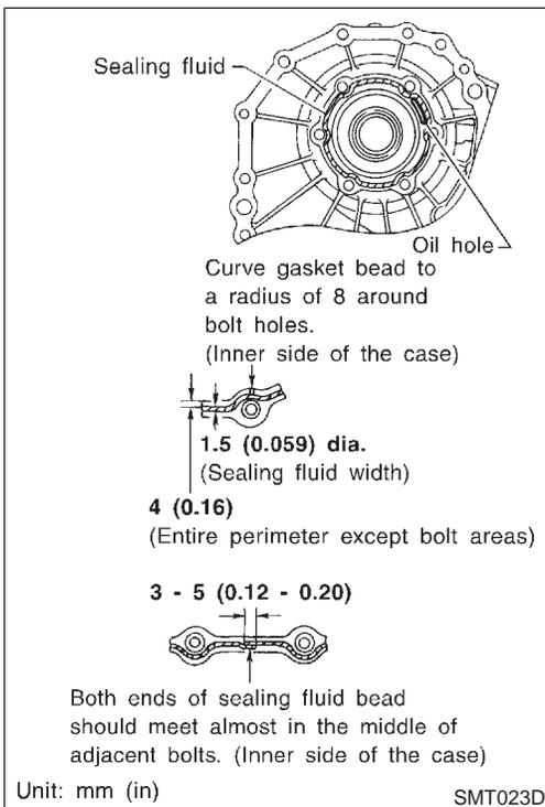
18. Apply Genuine Anaerobic Liquid Gasket or equivalent to transfer cover mounting surface of front case as shown in the figure.
