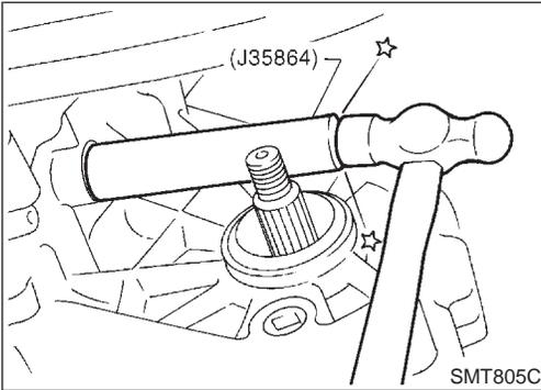
5. Install shift shaft oil seal.
