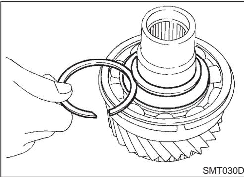
2. Select snap ring with proper thickness and install it.
