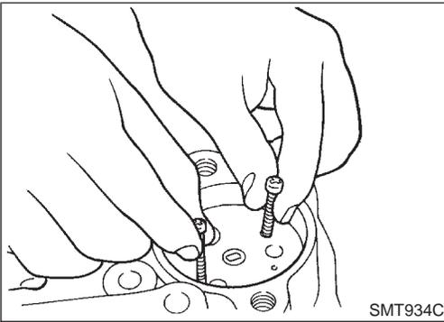
3. Thread two bolts (M4 x 0.8) into the holes of sub-oil pump as shown in the figure, and pull out to remove sub-oil pump.
