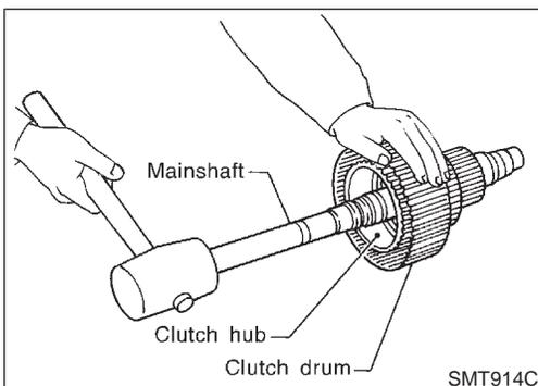
12. Tap mainshaft with a plastic hammer to remove it from clutch drum and clutch hub.
