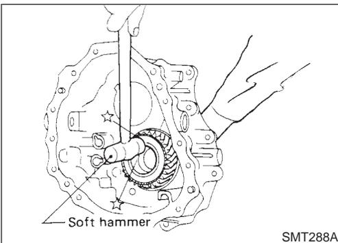
i. Remove main gear by tapping lightly.
