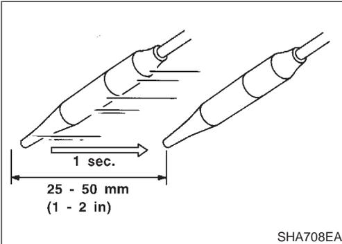
3. Move probe along component approximately 25 to 50 mm (1 to 2 in)/sec.
