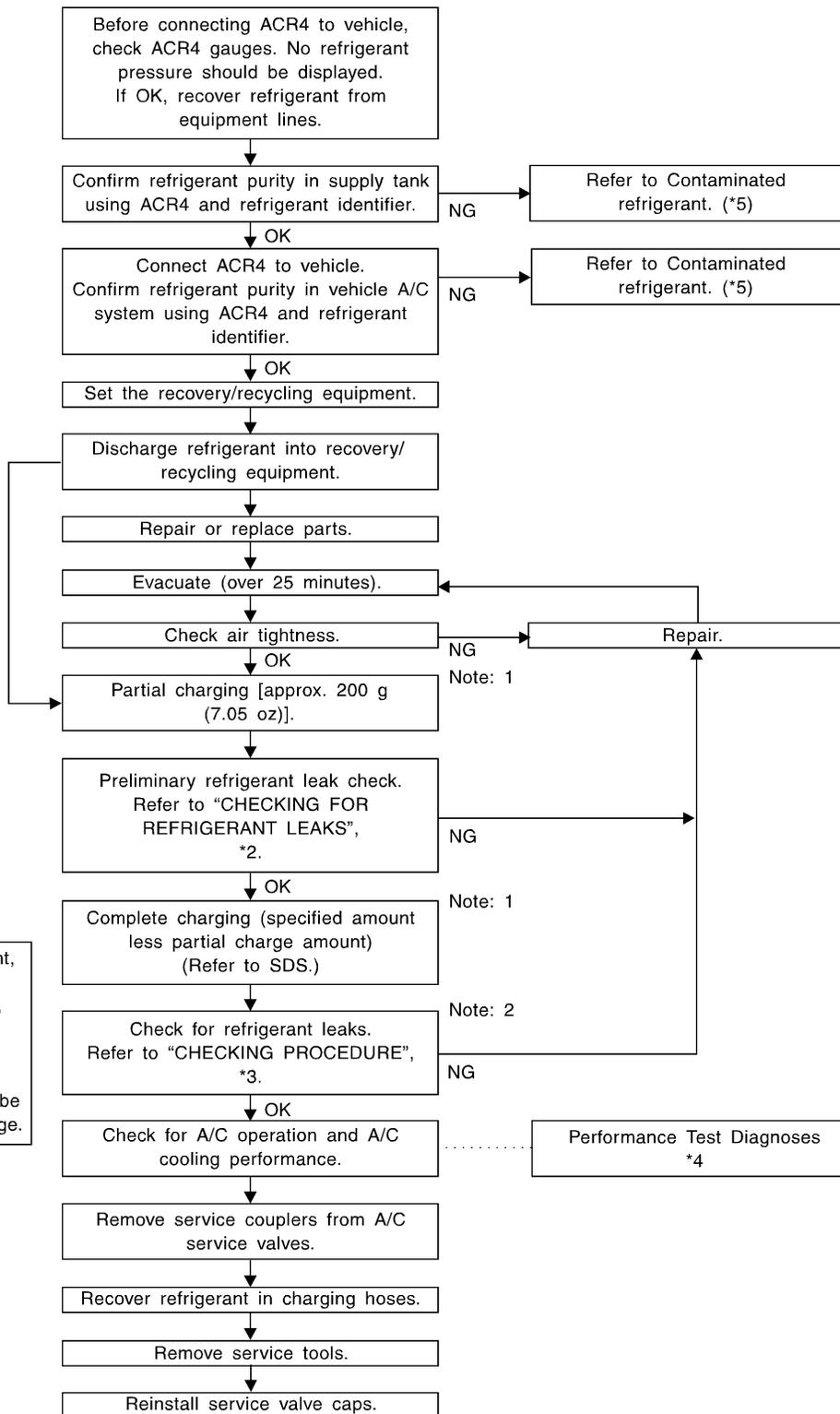
Note: 1 Before charging refrigerant, ensure engine is off.
