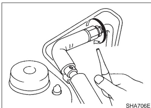
2. When testing, circle each fitting completely with probe.
