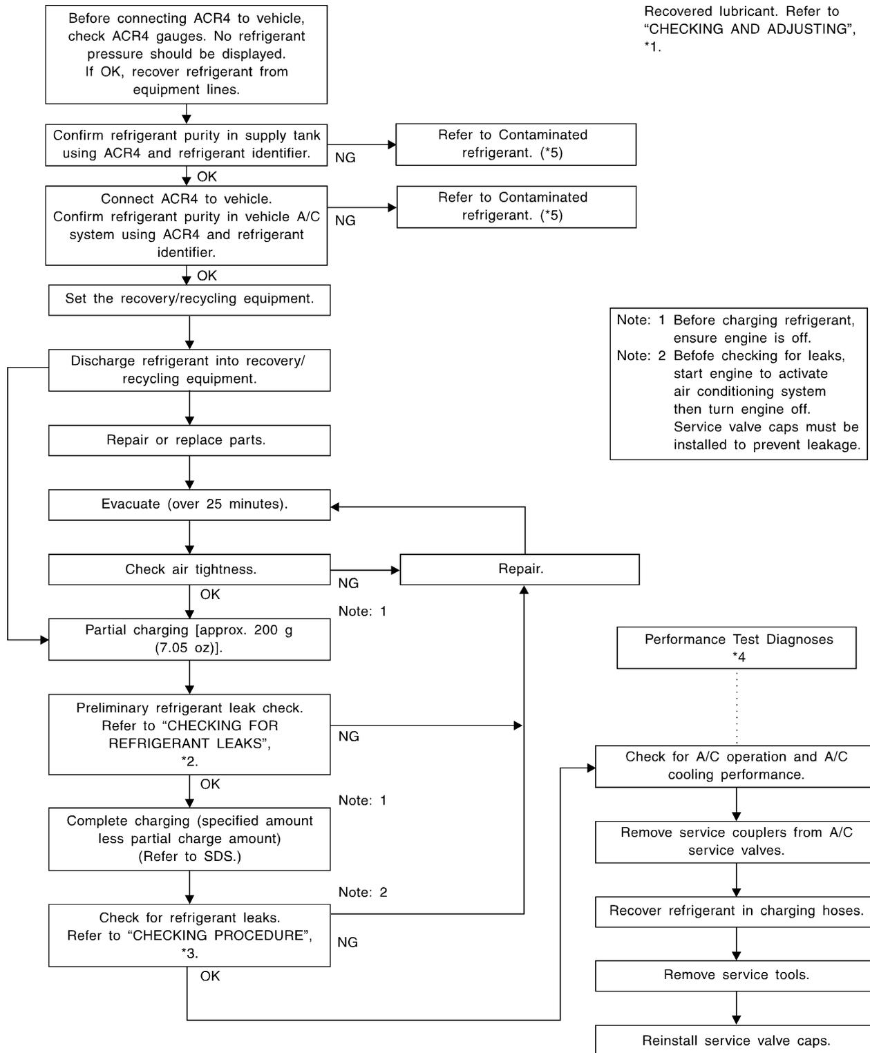
Note: 1 Before charging refrigerant, ensure engine is off.
