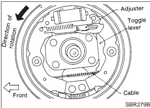
4. Connect parking brake cable to toggle lever.
