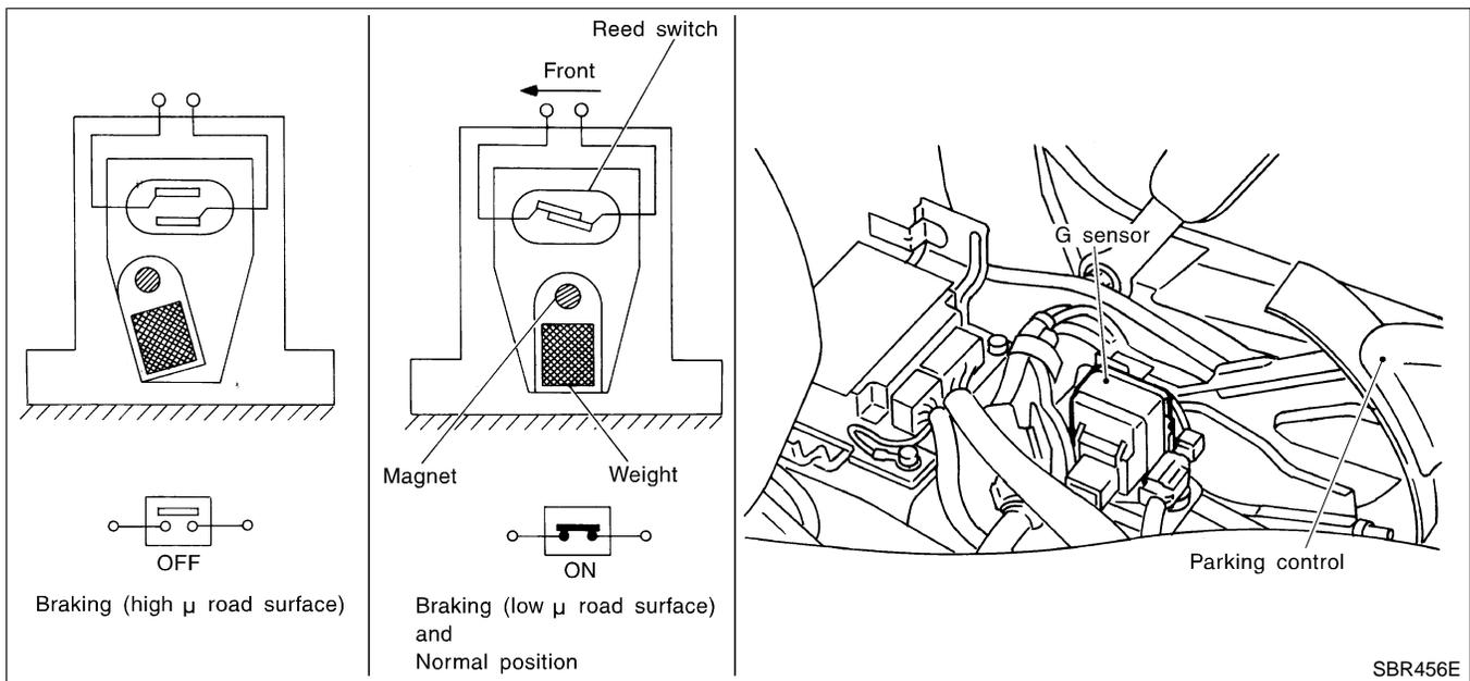
The reed switch turns on when it is affected by a magnetic field. During sudden deceleration (braking on a high  $\mu$  road), the weight moves and the magnet in the weight moves away from the reed switch. The magnetic field then diminishes and the reed switch turns off.
