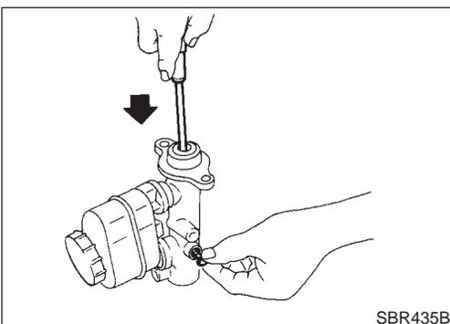
5. Install valve stopper while piston is pushed into cylinder.
