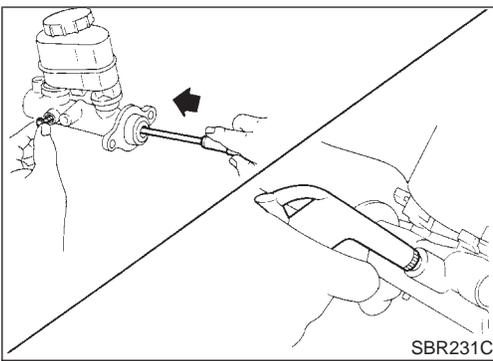
2. Remove piston stopper while piston is pushed into cylinder.
