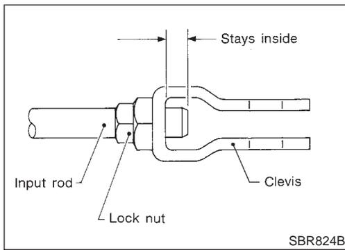
1. Loosen lock nut and adjust pedal free height by turning brake booster input rod. Then tighten lock nut.
