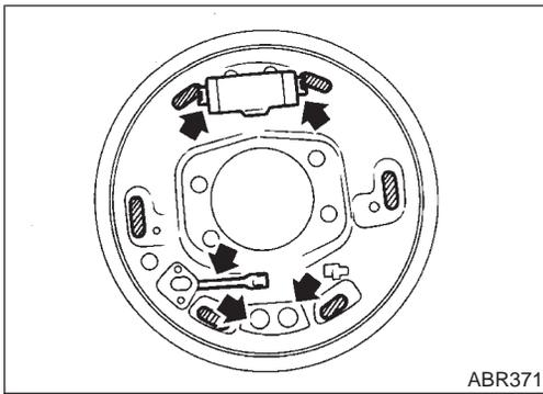
2. Apply brake grease to the contact areas (indicated by arrows and hatching) shown at left.
