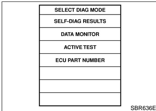
9. After the malfunctions are repaired, erase the self-diagnostic results stored in the control unit by touching "ERASE".
