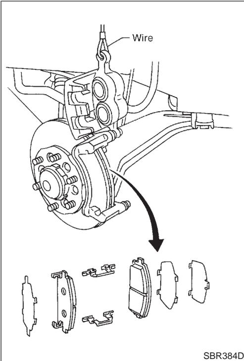
3. Open cylinder body upward. Then remove pad retainers, and inner and outer shims.
