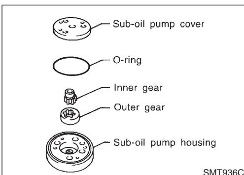
2. Install outer gear\* and inner gear to sub-oil pump housing, and measure side clearance. Refer to "Sub-oil Pump", "INSPECTION", TF-169.
