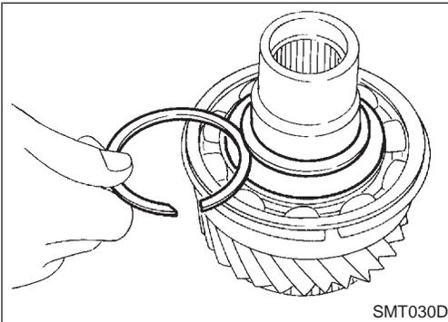
2. Select snap ring with proper thickness and install it.
