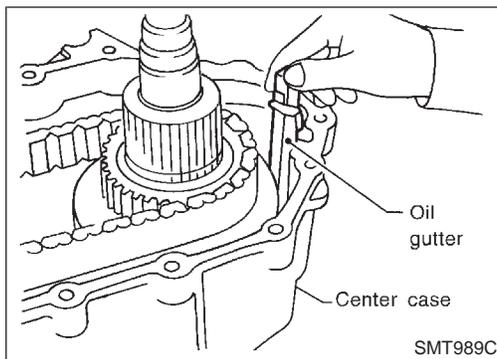
5. Align claw of oil gutter with center case, and install it.
