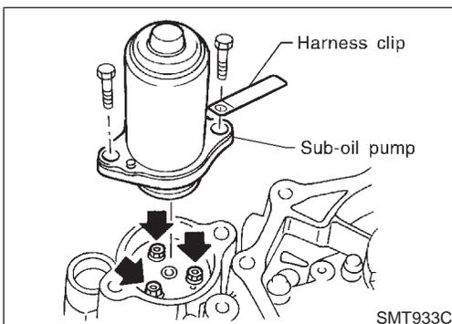
2. Remove sub-oil pump mounting bolts.
