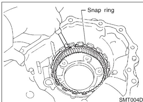
10. Remove snap ring, and remove internal gear.
