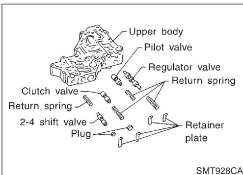
12. Remove each control valve, spring and plug.
