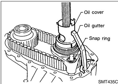
5. Remove oil cover and oil gutter.
