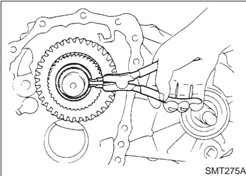
10. Disassemble center case assembly.
