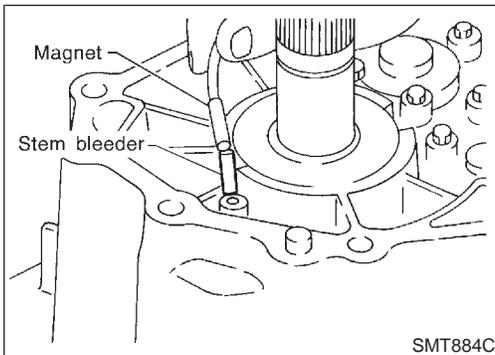
2. Remove stem bleeder from bleeder hole.
