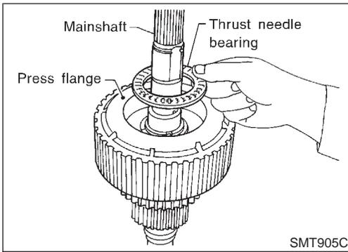
3. Remove thrust needle bearing from press flange.
