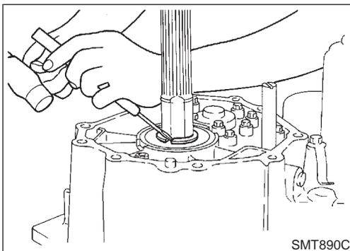
8. Remove C-rings from mainshaft bearing.
