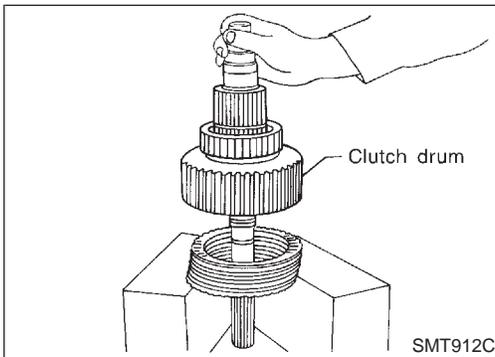
10. Remove each plate from clutch drum.
