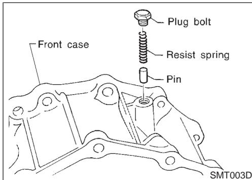
9. Remove plug bolt, then remove resist spring and pin.
