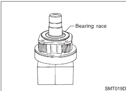
13. Set planetary carrier to press in the status described in step 8. Then install the selected bearing race to planetary carrier.
