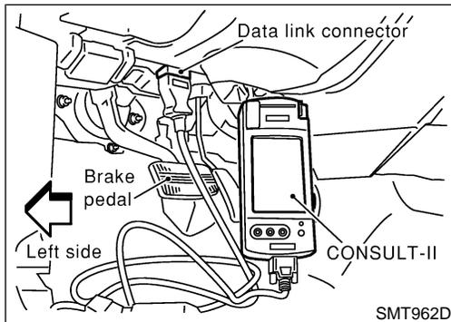
2. Connect CONSULT-II to data link connector which is located in instrument lower panel on driver side.
