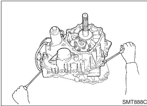
6. Insert screwdrivers as shown in the figure, and separate center case from front case. Then, remove center case by levering it up with a tire lever or the like.
