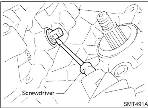
4. Remove shift shaft oil seal.
