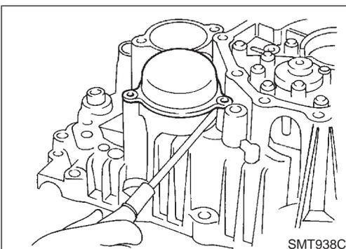
2. Insert a screwdriver as shown in the figure to remove oil filter.
