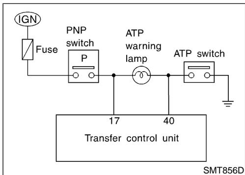
**Symptom 4. ATP Warning Lamp Does Not Turn ON**
