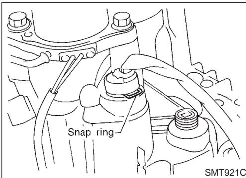
11. Secure terminal body with snap ring.
