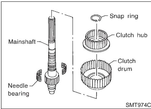
5. Install clutch drum, needle bearing and clutch hub to mainshaft, and secure them with snap ring.
