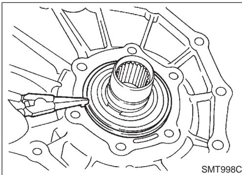
4. Remove snap ring from main gear bearing.
