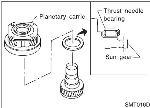
6. Install thrust needle bearing to sun gear.
