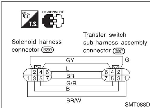
**TRANSFER TERMINAL CORD ASSEMBLY SUB-HARNESS CONNECTOR**
