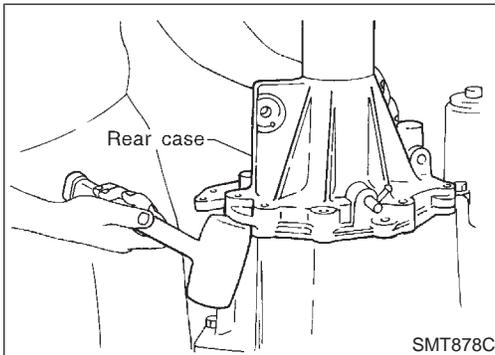
3. Remove rear case from center case by tapping it lightly with a plastic hammer.
