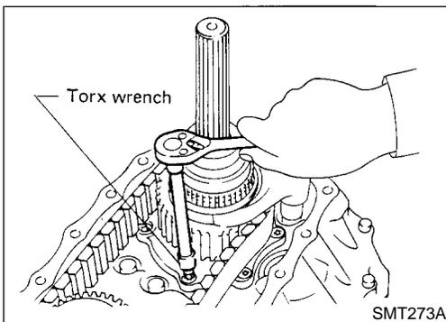
7. Remove bolts securing bearing retainer.
