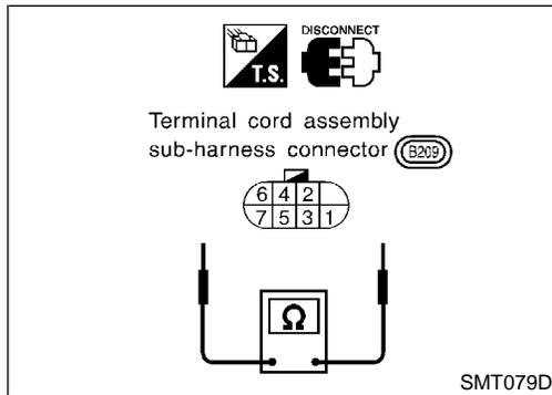
2-4WD Shift Solenoid Valve and Transfer Fluid Temperature Sensor
