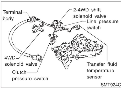
7. Remove 4WD solenoid valve, clutch pressure switch, 2-4WD shift solenoid valve, line pressure switch, and transfer fluid temperature sensor from control valve assembly.
