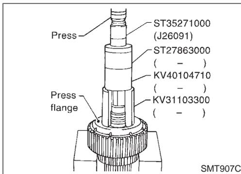
10. Pass mainshaft through snap ring. Set a drift (KV31103300), a support ring (KV40104710), a support ring (ST27863000) and a drift (ST35271000) to press flange at the position shown in the figure, and press snap ring until it fits into snap ring groove on mainshaft.
