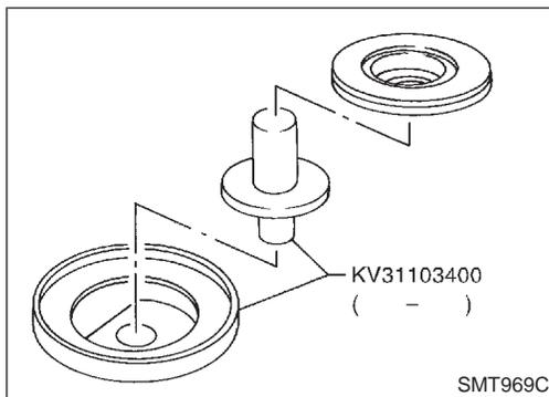
2. Set clutch piston to a clutch piston attachment (KV31103400).
