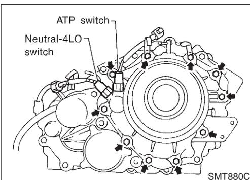
15. Remove all the gasket fluid 1215 (Three Bond) from switch mounting area and inside rear case, with ATP switch and neutral-4LO switch threaded in 1 to 2 pitches, apply gasket fluid 1215 (Three Bond) to the thread of the switches and tighten it to specified torque.
