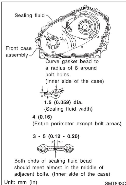
3. Apply sealing fluid 518 (Loctite) to the entire center case mounting surface of front case as shown in the figure.
