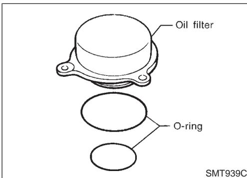
3. Apply ATF or petroleum jelly to two new O-rings, and install them to oil filter.
