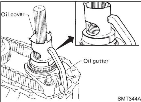
8. Install oil gutter and oil cover.
