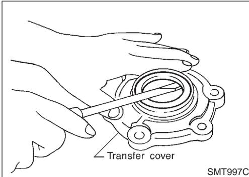
3. Remove oil seal from transfer cover.
