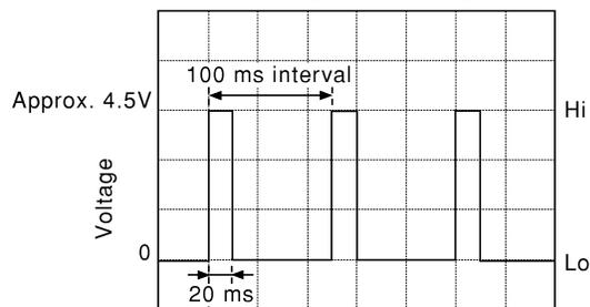
② ABS waveform during operation
