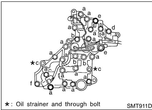
9. Install bolts as shown in the figure, and tighten them to specified torque.
