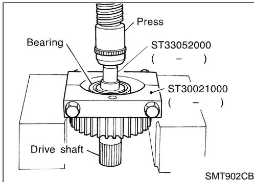
4. Set the puller (ST30021000) and the adapter (ST33052000). Remove front drive shaft rear bearing.
