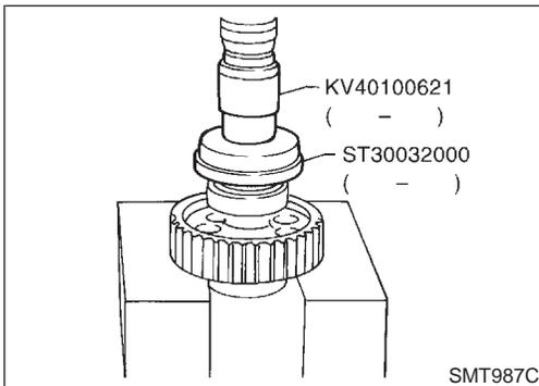
2. Place base (ST30032000) to front drive shaft front bearing inner race, and press it using the drift (KV40100621).
