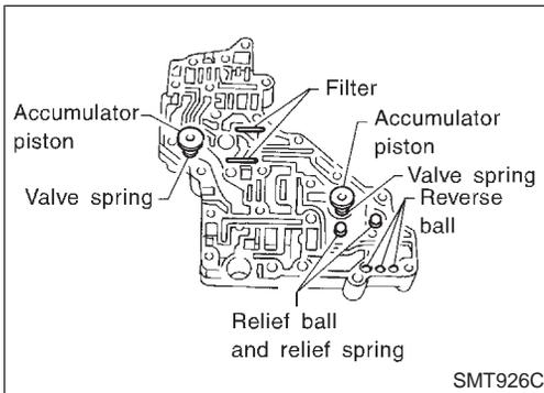
10. Make sure reverse balls, relief balls and relief springs, accumulator pistons, valve springs, and filters are securely installed as shown in the figure, and remove them.
