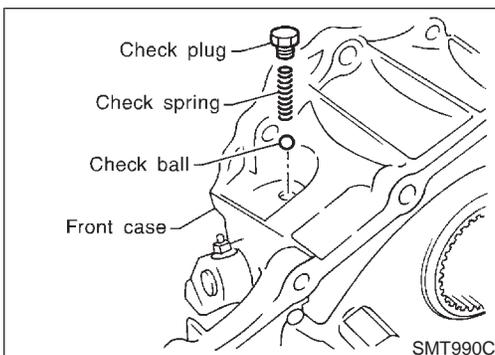
4. Remove all the liquid gasket on check plug and front case, and install check ball and check spring to front case. Apply gasket fluid 1215 (Three Bond) to check plug, install it to front case, and tighten it to specified torque.
