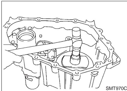
3. Set the clutch piston attachment to center case, and install clutch piston, tap it lightly.
