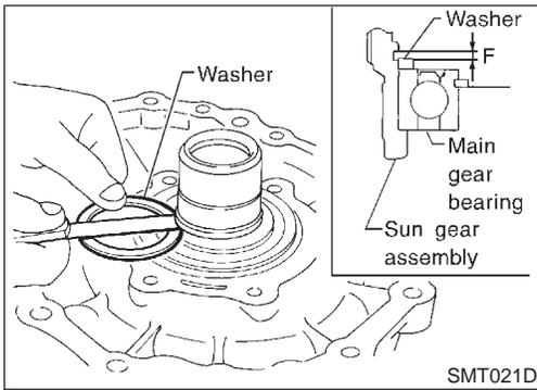
15. Install washer to sun gear assembly, and select proper snap ring so that end play "F" of sun gear is within specifications.
