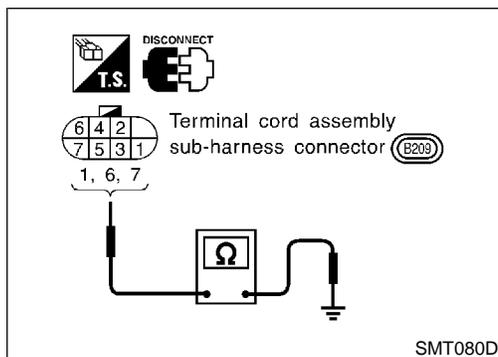
4WD Solenoid Valve, Clutch Pressure Switch and Line Pressure Switch
