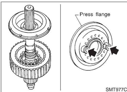
8. Install press flange (with the holes indicated by arrows aligned with pins of clutch hub).
