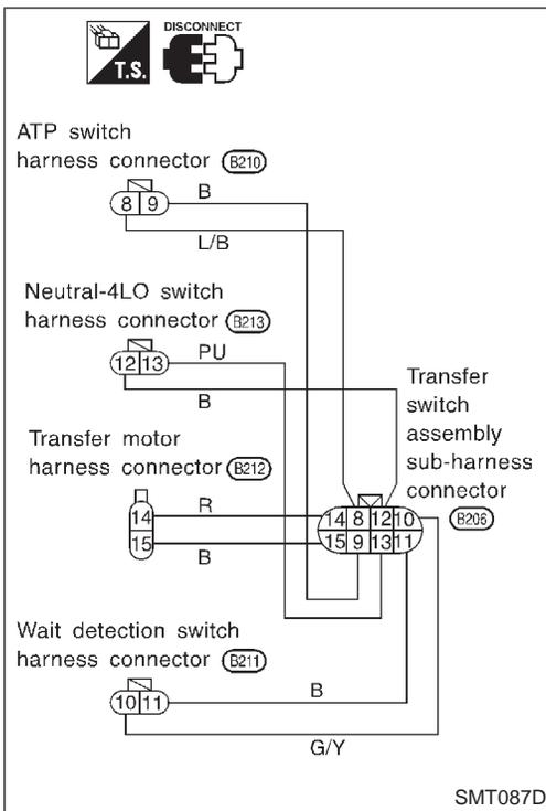
**TRANSFER SWITCH ASSEMBLY SUB-HARNESS CONNECTOR**
