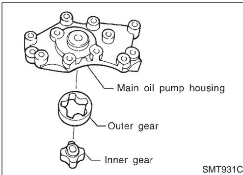
2. Remove outer gear and inner gear.
