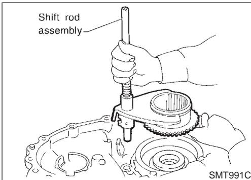
3. While aligning L-H sleeve with planetary carrier, install shift rod assembly to front case.
