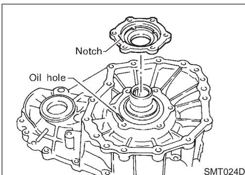
19. Align oil hole of front case with notch of transfer cover, and tighten bolts.
