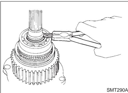
3. Remove snap ring and spacer.
