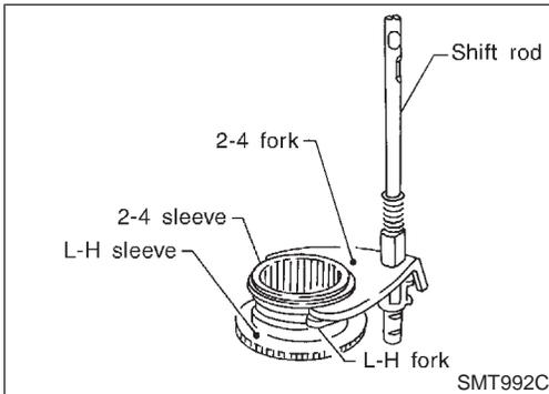
4. Remove 2-4 sleeve and L-H sleeve from 2-4 fork and L-H fork respectively.
