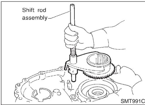
3. Remove shift rod components together with 2-4 sleeve and L-H sleeve.
