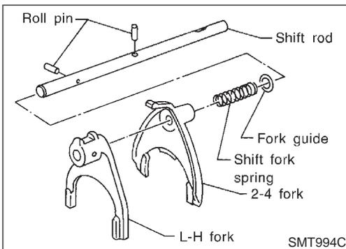
6. Remove L-H fork, 2-4 fork, shift fork spring and fork guide from shift rod.
