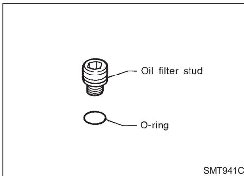
5. Remove O-ring from oil filter stud.
