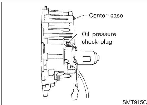
5. Remove all the liquid gasket from oil pressure check port and inside center case. With oil pressure check plug threaded in 1 or 2 pitches, apply gasket fluid 1215 (Three Bond) to the thread of plug, and tighten.
