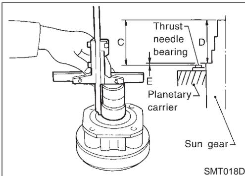
11. Measure "D" from the end of sun gear to the main gear bearing contact surface.
