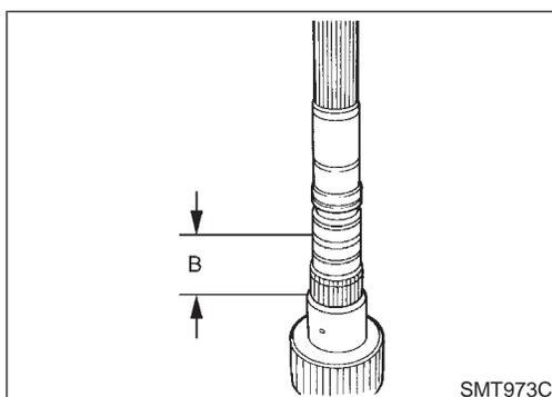
3. Measure dimension "B" between the gear end of mainshaft and the snap ring mounting portion.
