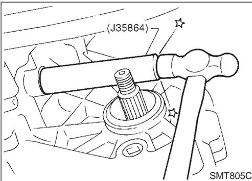
5. Install shift shaft oil seal.
