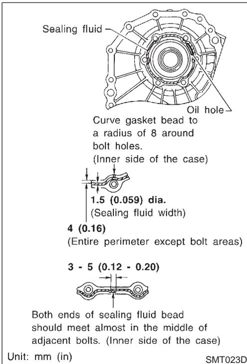
18. Apply sealing fluid (Loctite 518-C1335 x 25) to transfer cover mounting surface of front case as shown in the figure.
