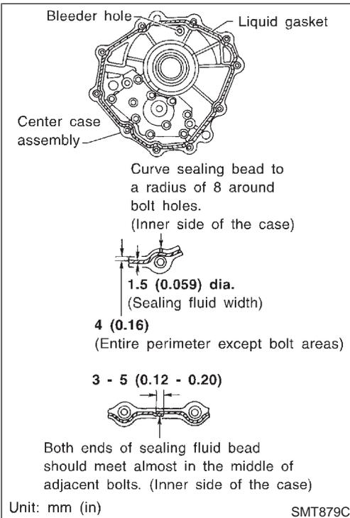
13. Apply sealing fluid 518 (Loctite) to entire rear case mounting surface of center case as shown in the figure.
