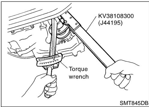
17. Install companion flange to front drive shaft, and tighten mounting nut.
