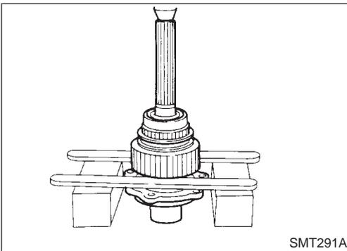
4. Press out front drive sprocket with mainshaft rear bearing and clutch gear together.
