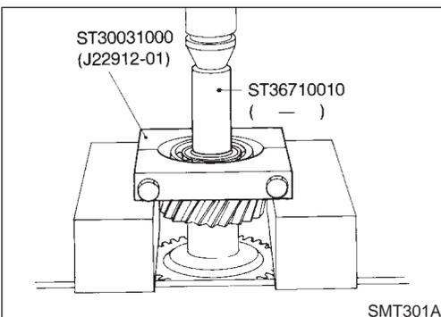
2. Press out counter gear rear bearing.
