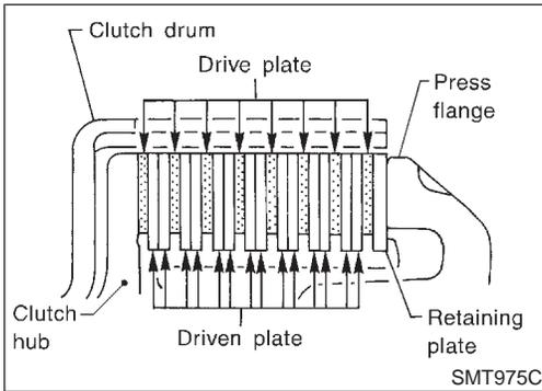
6. Install each clutch to clutch drum.
