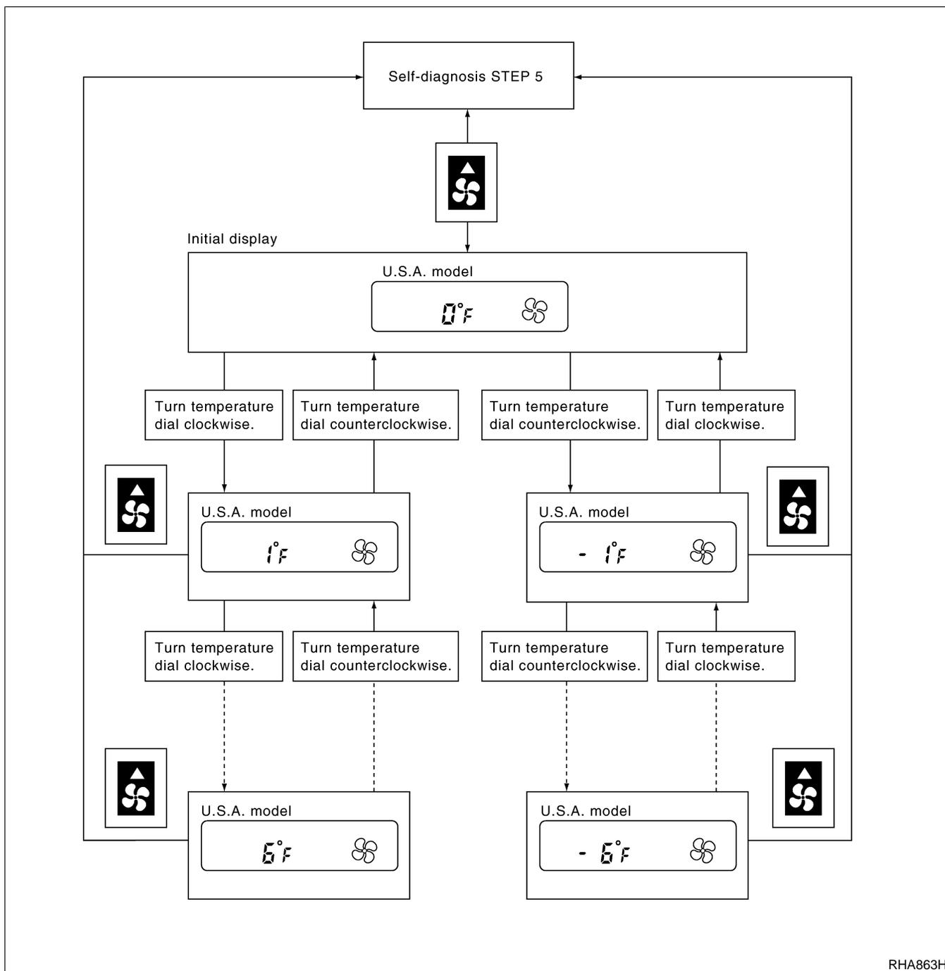
**When battery cable is disconnected, trimmer operation is canceled. Temperature set becomes that of initial condition, i.e.  $0^{\circ}\text{C}$  ( $0^{\circ}\text{F}$ ).**
