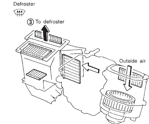
← : Air passed through heater core
