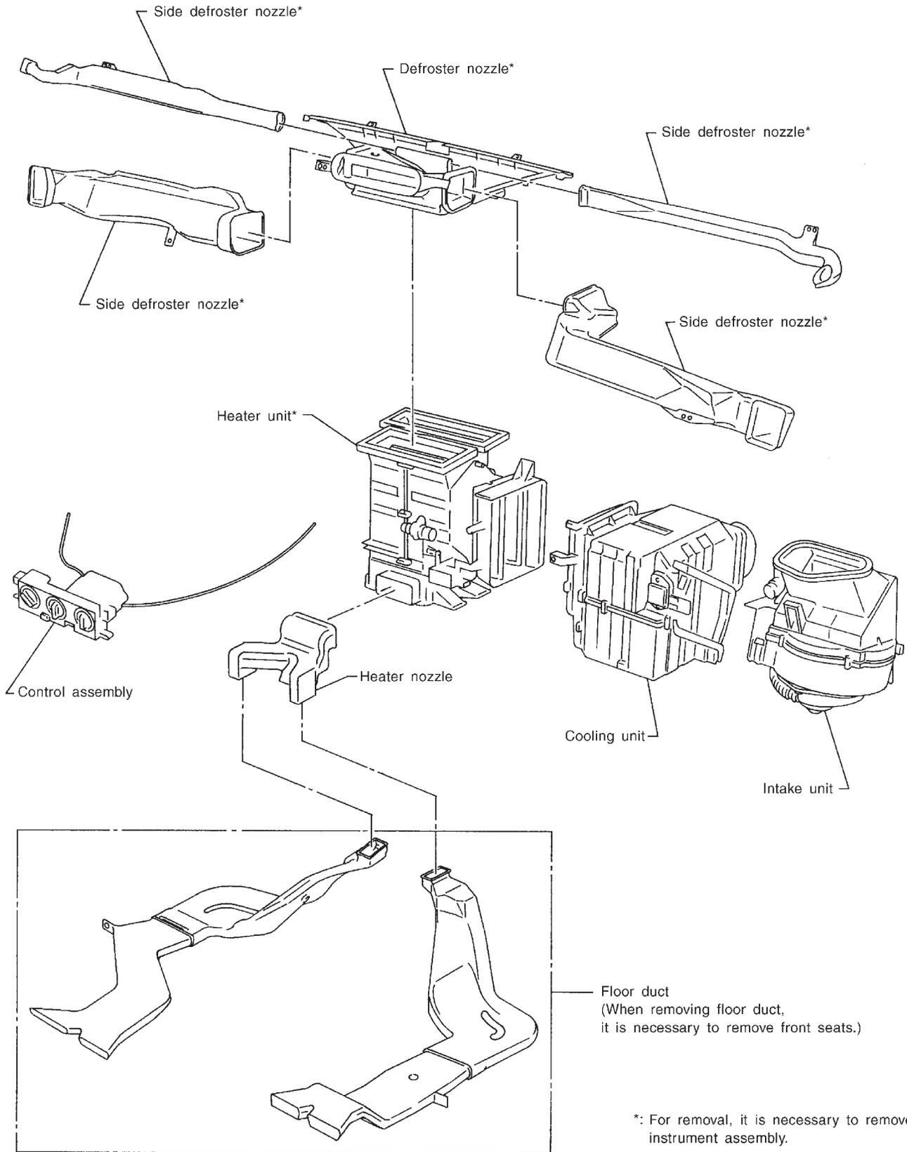
\*: For removal, it is necessary to remove instrument assembly.
