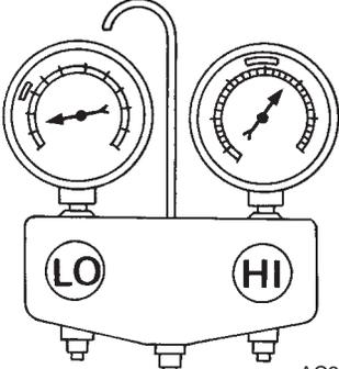
AC360A | Upper side of condenser and high-pressure side are hot, however, liquid tank is not so hot. | High-pressure tube or parts located between compressor and condenser are clogged or crushed. | <ul style="list-style-type: none"> <li>Check and repair or replace malfunctioning parts.</li> <li>Check lubricant for contamination.</li> </ul> |
