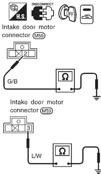
Continuity should exist when test leads are connected as shown, it should not exist when test leads are reversed.
