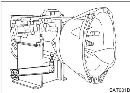
7. Install turbine revolution sensor.
