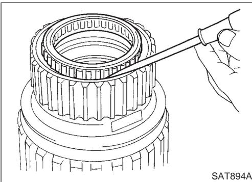
3. Install low one-way clutch onto forward clutch drum by pushing the roller in evenly.
