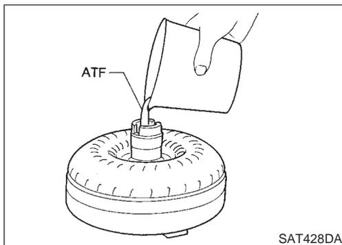
13. Install torque converter.
