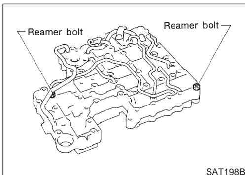
f. Temporarily assemble lower and upper bodies, using reamer bolt as a guide.
