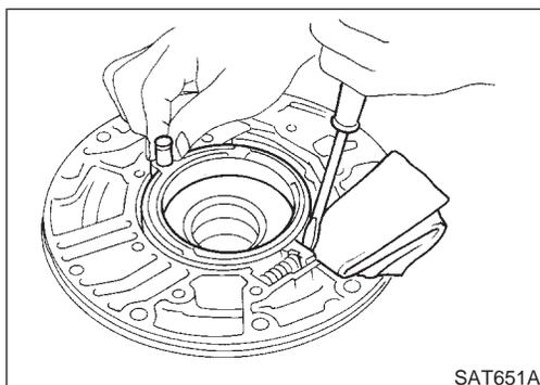
3. While pushing on cam ring remove pivot pin.
