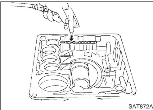
7. Check operation of low and reverse brake clutch piston. Refer to "DISASSEMBLY", AT-325.
