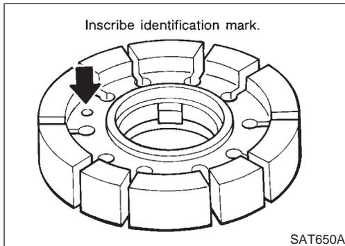
2. Remove rotor, vane rings and vanes.
