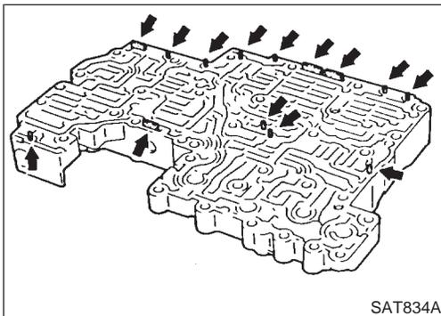
2. Install parallel pins and retainer plates.
