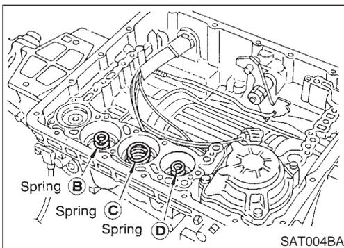
10. Install control valve assembly.
