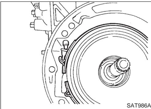
b. Remove brake band and band strut from transmission case.
