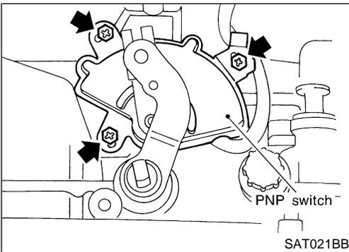
5. Remove PNP switch from transmission case.
