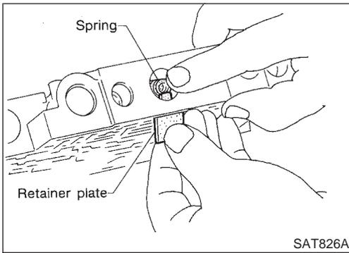
b. Remove retainer plates while holding spring.
