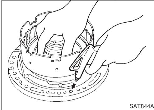
5. Install seal ring onto oil pump cover and install reverse clutch drum. While holding piston, gradually apply compressed air to oil hole until piston is removed.
