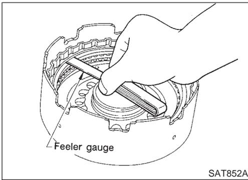
7. Measure clearance between retaining plate and snap ring. If not within allowable limit, select proper retaining plate.
