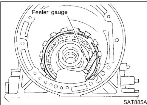
8. Measure clearance between retaining plate and snap ring. If not within allowable limit, select proper retaining plate.
