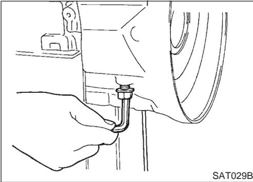
17. Remove brake band and band strut.
