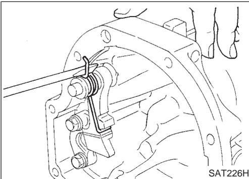
4. Bend return spring upward and install it onto adapter case.
