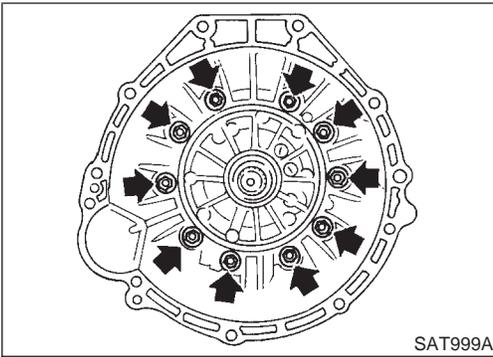
13. Remove converter housing from transmission case.
