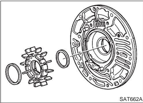
3. Install rotor, vanes and vane rings.
