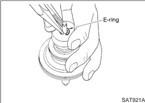
6. Place piston stem end on a wooden block. While pushing servo piston spring retainer down, install E-ring.
