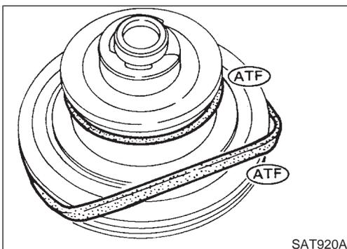
4. Install D-rings onto band servo piston.
