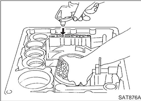
6. Remove low and reverse brake piston using compressed air.
