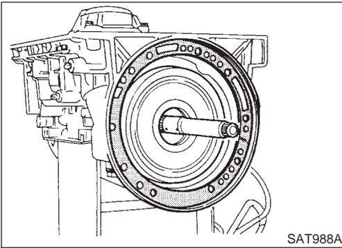
2. Install input shaft on transmission case.
