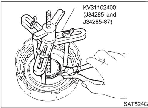
3. Remove snap ring from clutch drum while compressing clutch springs.
