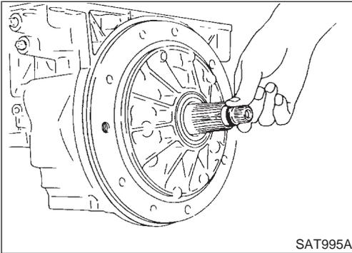
14. Remove O-ring from input shaft.
