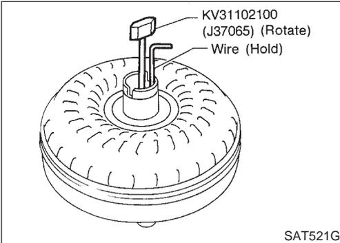
4. Check torque converter one-way clutch.
