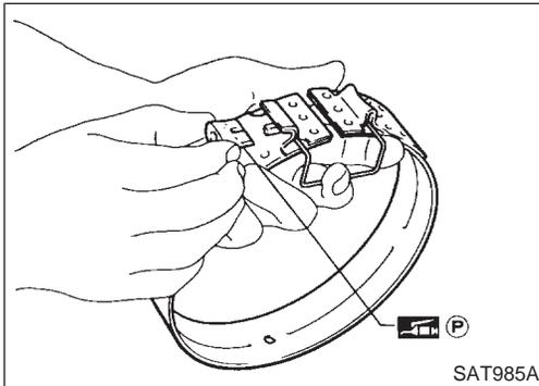
1. Install brake band and band strut.
