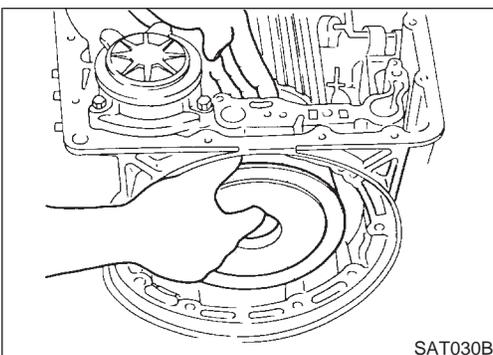
18. Remove front side clutch and gear components.
