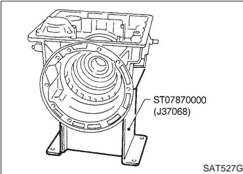
h. Place transmission case into horizontal position.
