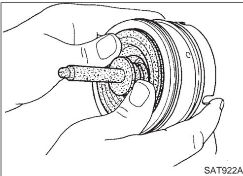
7. Install band servo piston assembly onto servo piston retainer by pushing it inward.
