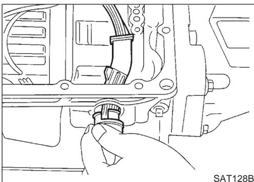
12. Remove terminal cord assembly from transmission case while pushing on stopper.
