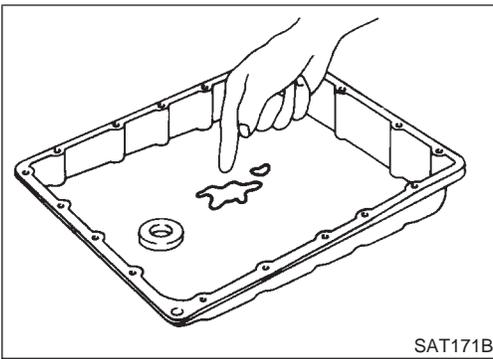
8. Check foreign materials in oil pan to help determine cause of malfunction. If the fluid is very dark, smells burned, or contains foreign particles, the frictional material (clutches, band) may need replacement. A tacky film that will not wipe clean indicates varnish build up. Varnish can cause valves, servo, and clutches to stick and may inhibit pump pressure.
