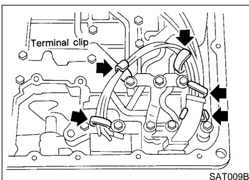
11. Remove control valve assembly.
