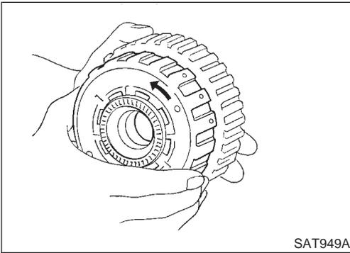
g. Check that overrun clutch hub rotates as shown while holding forward clutch hub.
