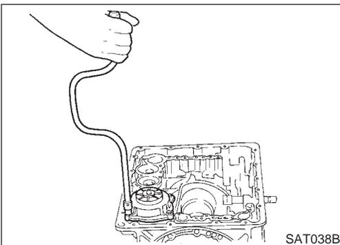
24. Remove band servo and accumulator components.
