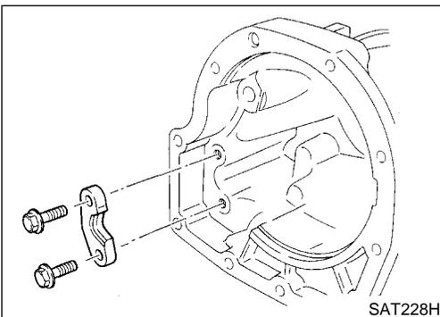
4. Remove parking actuator support from adapter case.
