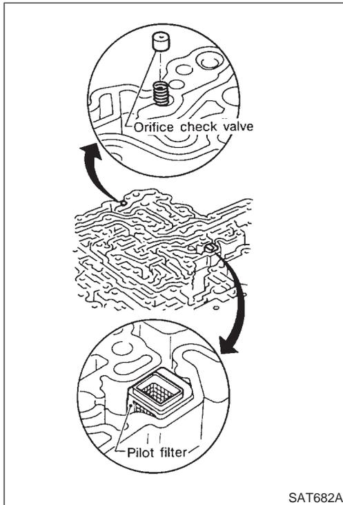
c. Place oil circuit of lower body face up. Install orifice check spring, orifice check valve and pilot filter.
