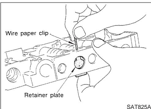
2. Remove valves at retainer plates.
