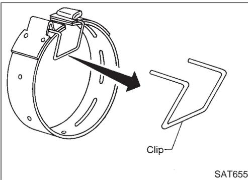
c. Hold brake band in a circular shape with clip.
