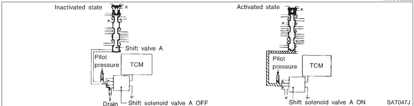
Pilot pressure generated by the operation of shift solenoid valves A and B is applied to the end face of shift valves A and B. The drawing above shows the operation of shift valve B. When the shift solenoid valve is "ON", pilot pressure applied to the end face of the shift valve overcomes spring force, moving the valve upward.
