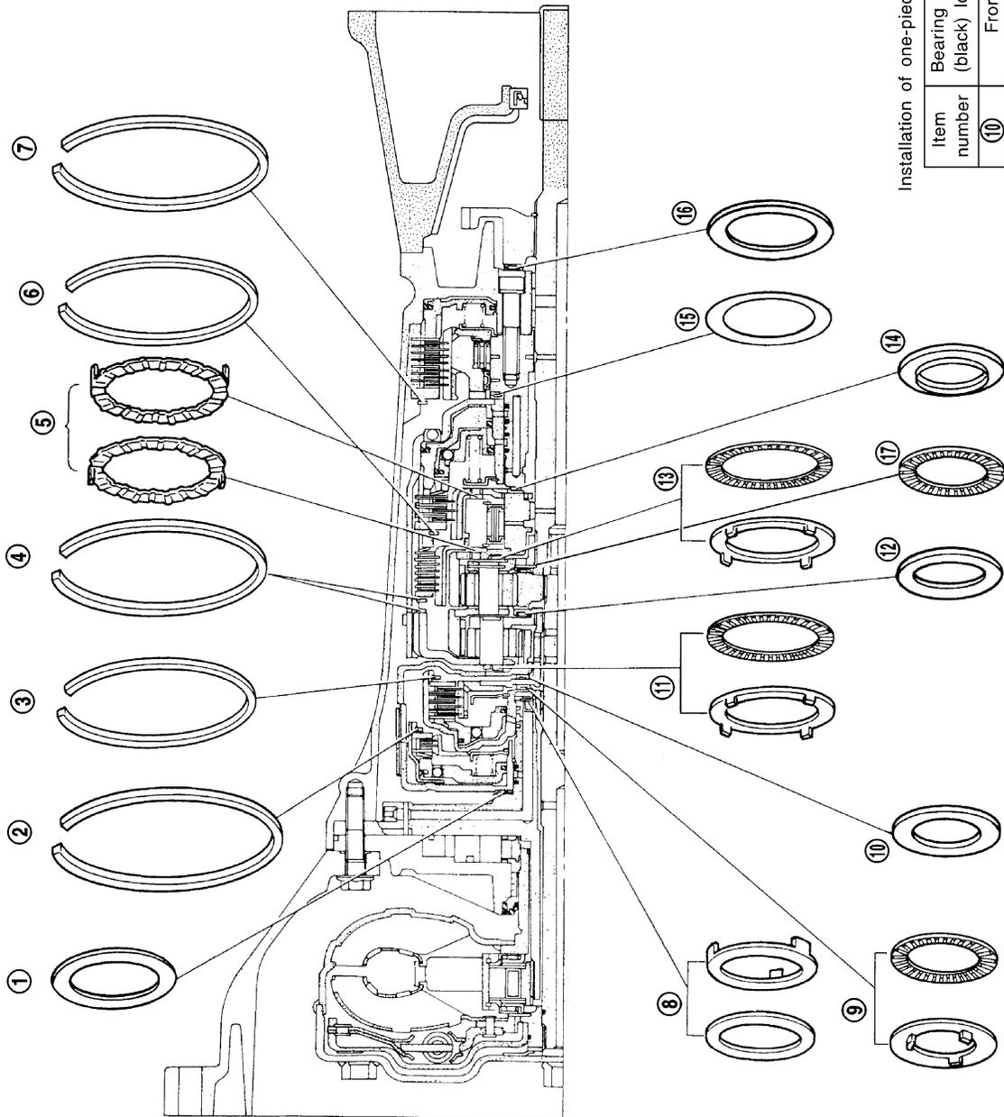
Installation of one-piece bearings
