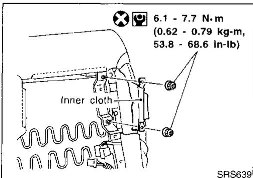
4. Secure the inner cloth which covers the side air bag module with nuts.
