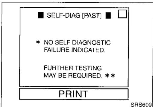
10. Check that no malfunction is detected on "SELF-DIAG [PAST]".
