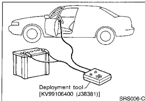
4. Connect red clip of deployment tool to battery positive terminal and black clip to negative terminal.
