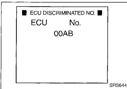
For NISSAN MODEL R50, the diagnosis sensor unit classification number assigned is 00AB.
