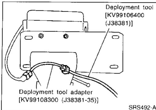
4. Connect deployment tool adapter [SST: KV99108300 (J38381-35)] to deployment tool [SST: KV99106400 (J38381)] connector and connector on air bag module.
