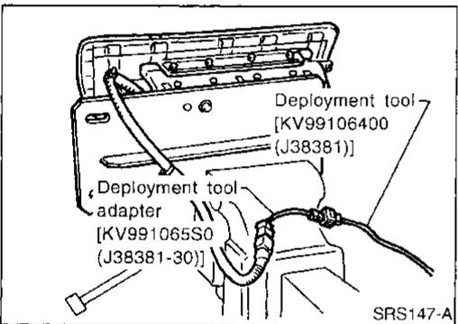
4. Connect deployment tool adapter [SST: KV991065S0 (J38381-30)] to deployment tool [SST: KV99106400 (J38381)] connector and air bag module connector.
