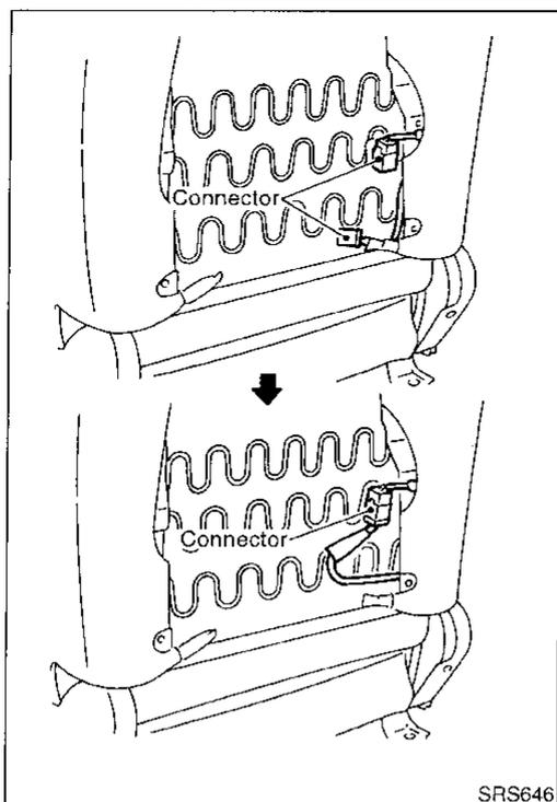
5. Connect side air bag module connector.
