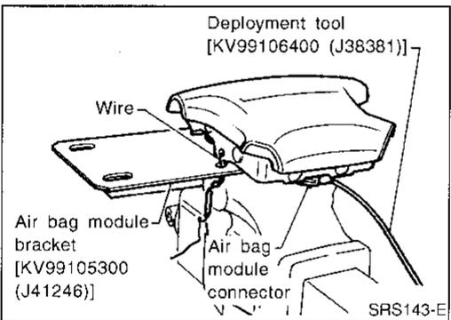
4. Connect deployment tool [SST: KV99106400 (J38381)] to air bag module connector.
