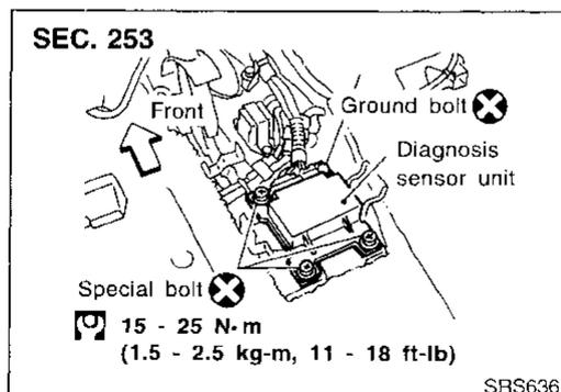
1. Disconnect connectors for driver and passenger air bag modules and seat belt pre-tensioner.
