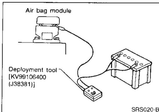
5. Connect red clip of deployment tool to battery positive terminal and black clip to negative terminal.
