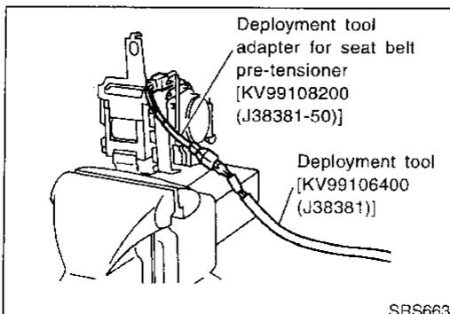
2. Connect deployment tool adapter [SST: KV99108200 (J38381-50)] to deployment tool [SST: KV99106400 (J38381)] connector and seat belt pre-tensioner connector.
