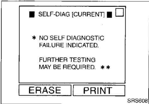
If no malfunction is detected on "SELF-DIAG [CURRENT]" even though malfunction is detected in "SRS Operation Check", check the battery voltage.
