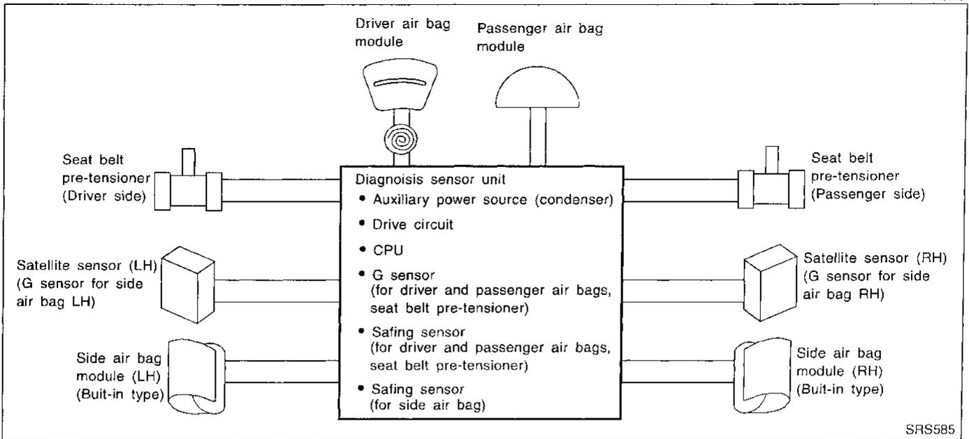
The air bag deploys if the diagnosis sensor unit activates while the ignition switch is in the "ON" or "START" position.
