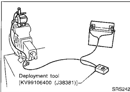
3. Connect red clip of deployment tool to battery positive terminal and black clip to negative terminal.
