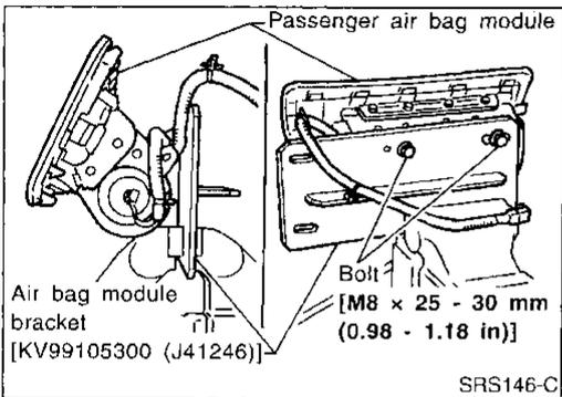
3. Match the two holes in air bag module bracket (held in vise) and passenger air bag module and fix them with two bolts [M8 x 25 - 30 mm (0.98 - 1.18 in)].
