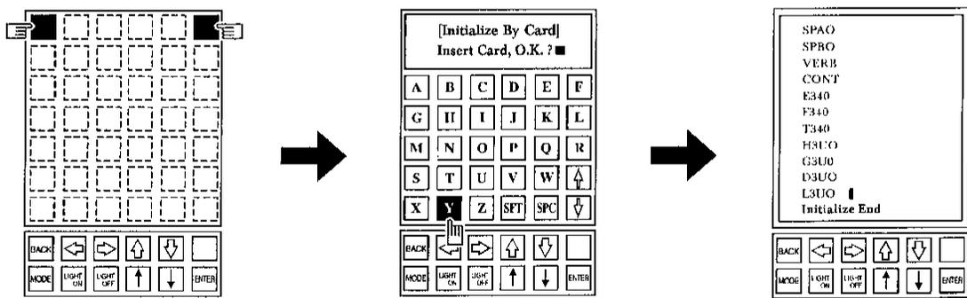
1. While holding down the upper left and right corner keys of the CONSULT touch panel, simultaneously press the power "ON" switch. While pushing the power "ON" switch, hold down both corner keys until the next screen appears.
