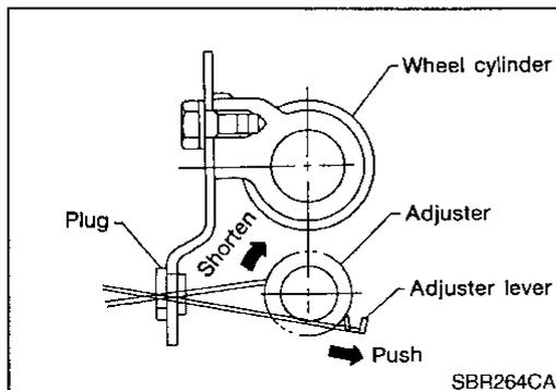
1. Release parking brake lever fully, then remove drum. If drum is hard to remove, the following procedures should be carried out.
