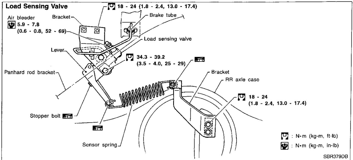
1. Tighten all flare nuts and mounting bolts.
