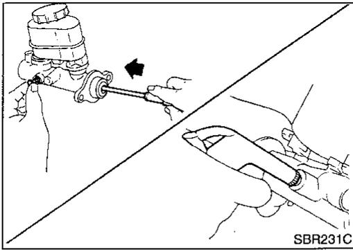
2. Remove piston stopper while piston is pushed into cylinder.
