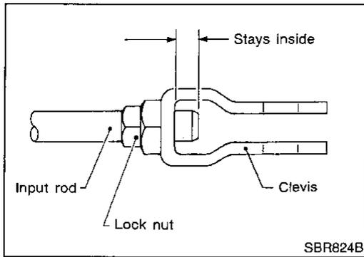
1. Loosen lock nut and adjust pedal free height by turning brake booster input rod. Then tighten lock nut.
