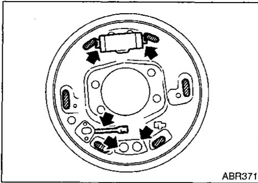
2. Apply brake grease to the contact areas (indicated by arrows and hatching) shown at left.
