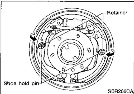
2. After removing shoe hold pin by rotating push retainer, remove leading shoe then remove trailing shoe. Remove spring by rotating shoes in direction arrow.
