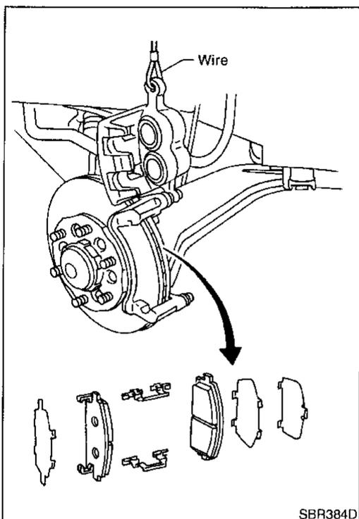
3. Open cylinder body upward. Then remove pad retainers, and inner and outer shims.
