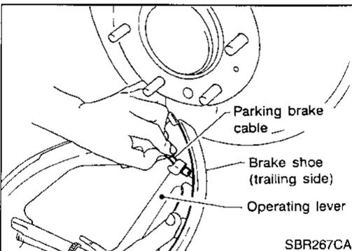
4. Disconnect parking brake cable from toggle lever.
