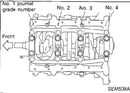
8. If crankshaft is reused, measure main bearing clearances and select thickness of main bearings.
