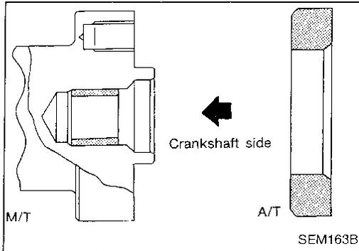
2. Install pilot bushing (M/T) or pilot converter (A/T).
