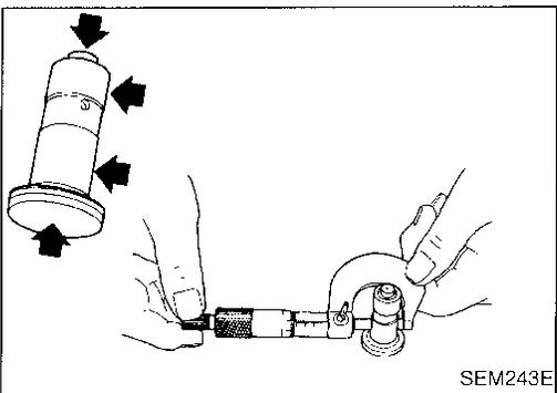
3. Check valve lifter guide inner diameter.
