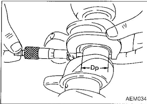
4. Measure outer diameter "Dp" of each crankshaft pin journal.
