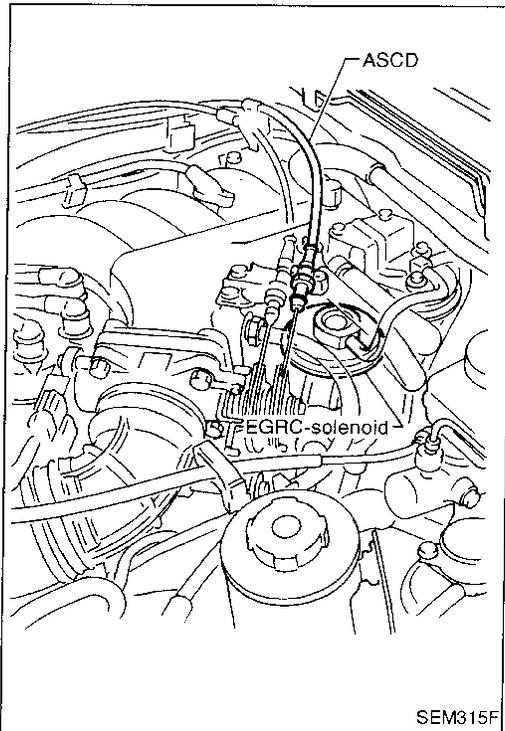
4. Separate ASCD and accelerator control wire from intake manifold collector.
