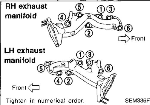
3. Install exhaust manifolds to cylinder head.
