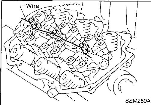
3. Install valve lifters into valve lifter guide.
