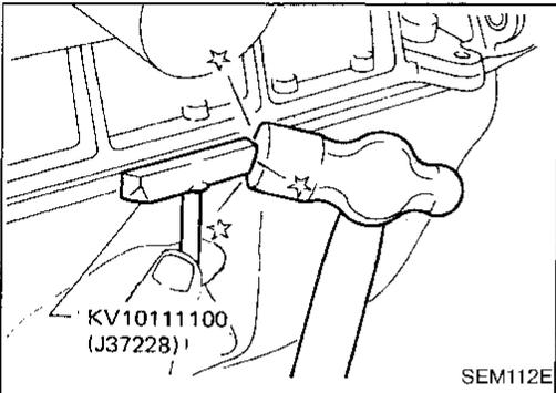
(2) Slide Tool by tapping its side with a hammer, and remove oil pan.
