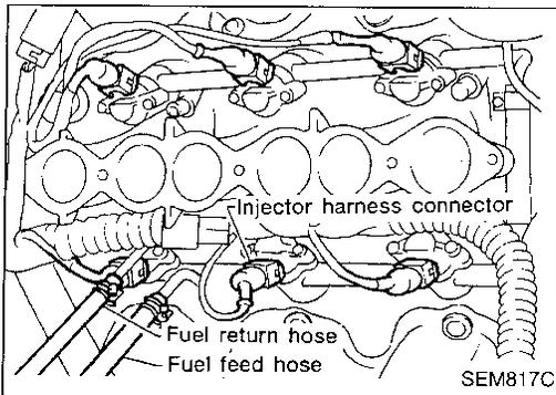
6. Remove fuel feed and fuel return hoses from injector fuel tube assembly.
