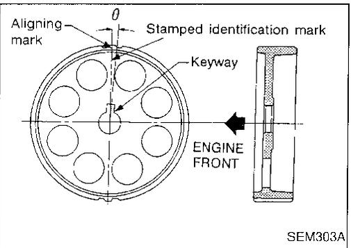
11. Install rear belt cover and camshaft sprocket.
