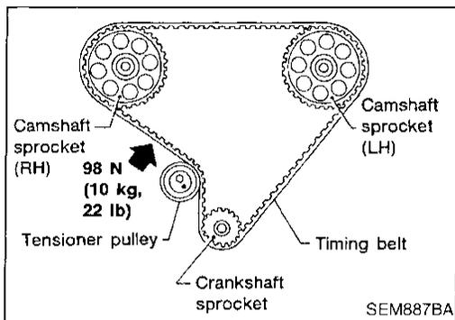
8. Push middle of timing belt between RH camshaft sprocket and tensioner pulley with force of 98 N (10 kg, 22 lb).
