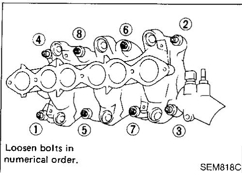
9. Remove intake manifold from engine. The following parts should be disconnected to remove intake manifold.
