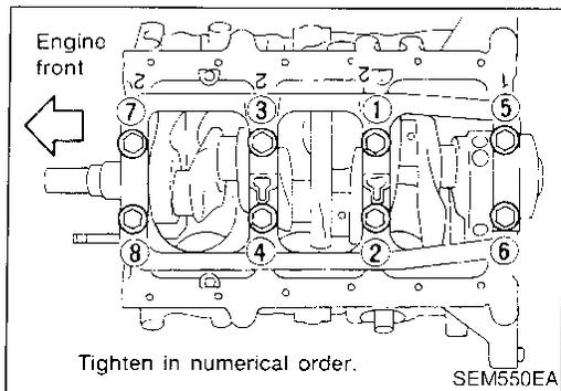
2. Install crankshaft and main bearing caps and tighten bolts to the specified torque.
