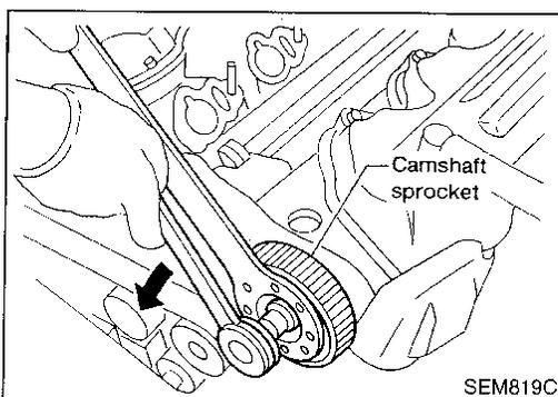
10. Remove both camshaft sprockets.
