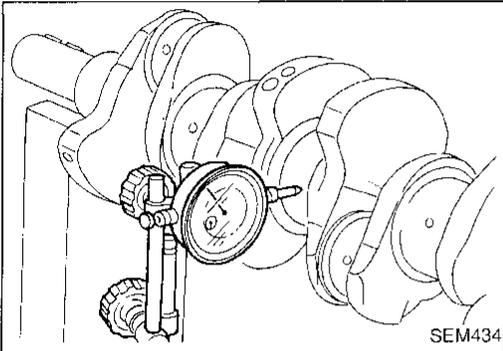
3. Measure crankshaft runout.
