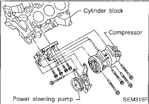
7. Install compressor and alternator bracket.
