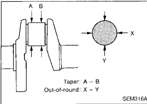
1. Check crankshaft main and pin journals for score, wear or cracks.
