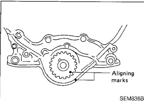
1. Set No. 1 piston at TDC on its compression stroke as follows:
