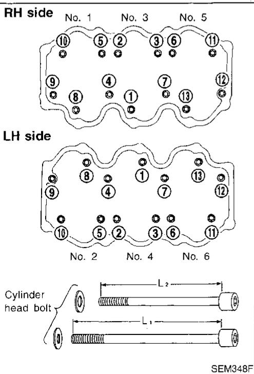
5. Tighten cylinder head bolts in numerical order using angle wrench [ST10120000 (J24239-01)].
