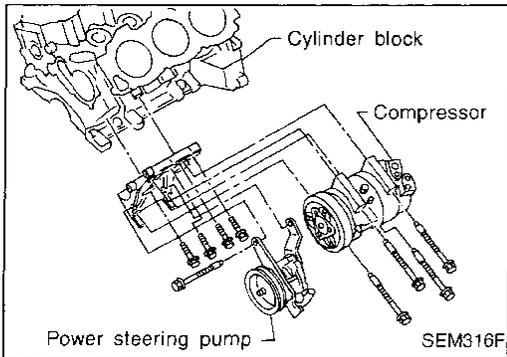
15. Remove compressor and power steering pump.
