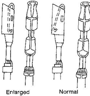
Any probe entering the terminal may enlarge the contact spring opening creating an intermittent signal.
