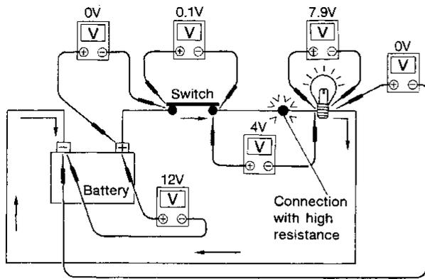
1. Connect the voltmeter as shown, starting at the battery and working your way around the circuit.
