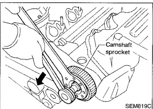
10. Remove both camshaft sprockets.
