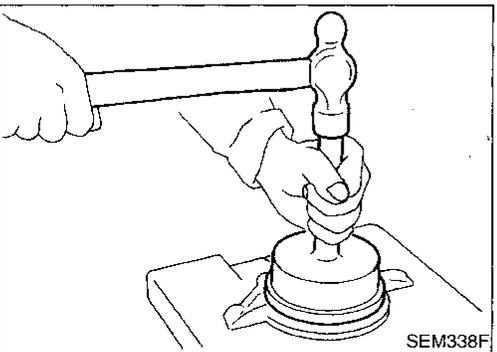
7. Install rear oil seal retainer.
