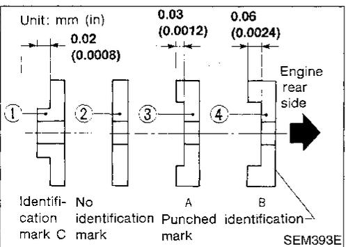
3. If it is out of the specified range, select thickness of camshaft locate plate to obtain standard specified end play.
