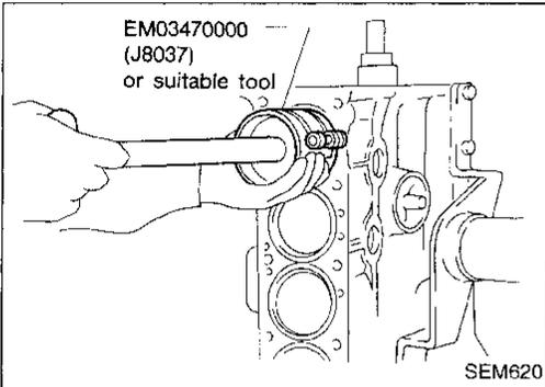
5. Install pistons with connecting rods.
