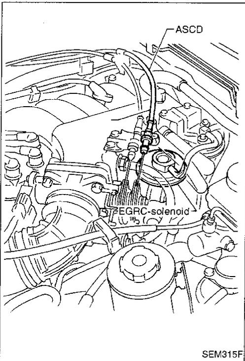
4. Separate ASCD and accelerator control wire from intake manifold collector.
