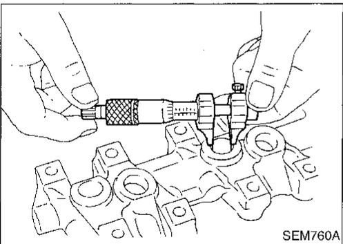
3. Check valve lifter guide inner diameter.
