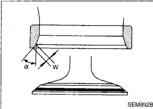
5. Cut or grind valve seat using suitable tool at the specified dimensions as shown in SDS (EM-49).
