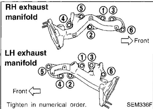
3. Install exhaust manifolds to cylinder head.
