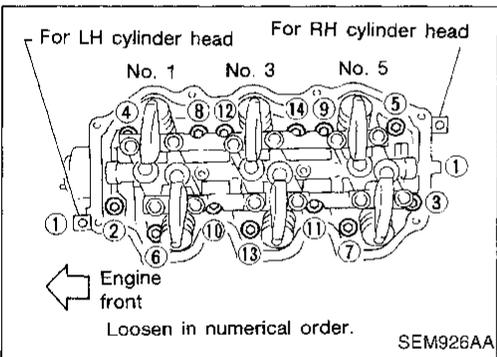
19. Remove cylinder head with exhaust manifold.
