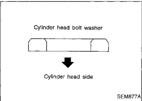
4. Install cylinder head with new gasket.
