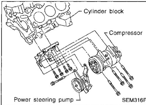
15. Remove compressor and power steering pump.
