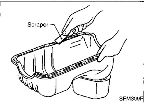
1. Before installing oil pan, remove all traces of liquid gasket from mating surface using a scraper.
