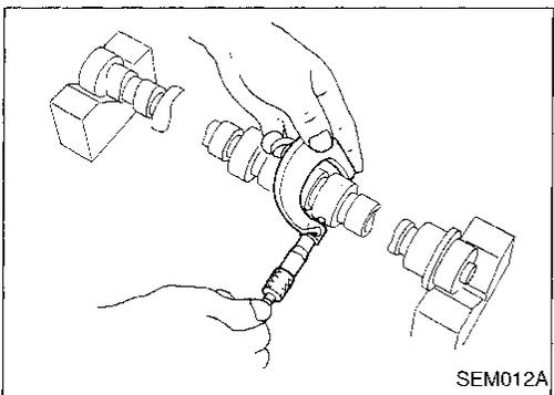
1. Measure inner diameter of camshaft bearing.
