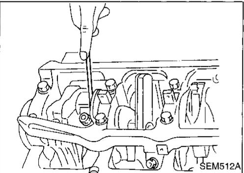
6. Measure connecting rod side clearance.
