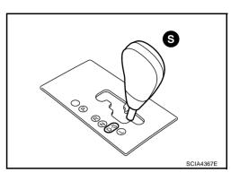
3. Accelerate vehicle by constantly depressing accelerator pedal fully depressed.
