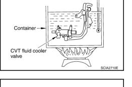
3. Make sure that CVT fluid cooler valve is fully closed.
