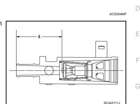
2. Put CVT fluid cooler valve into a water-filled container, and then heat it up to 82°C (180°F) or more for 10 minutes or more.
