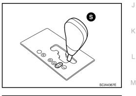
3. Accelerate vehicle by constantly depressing accelerator pedal half-way.
