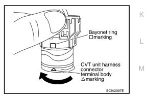
Rotate bayonet ring clockwise until ∆ marking on CVT unit harness connector terminal body is aligned with the slit on bayonet ring as shown in the figure (correctly fitting condition), install CVT unit harness connector to CVT unit harness connector terminal body.
