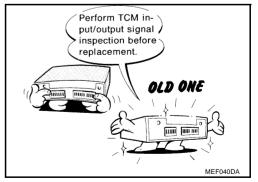
• When connecting or disconnecting pin connectors into or from TCM, take care not to damage pin terminals (bend or break).
