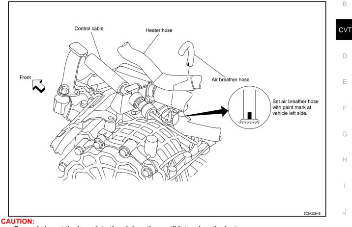
• Securely insert the hose into the air breather until it touches the bottom.
