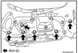
5. Remove rear plate cover. Refer to <u>EM-28, "Removal and Instal-</u> lation".
