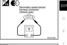
Check voltage between output speed sensor (secondary speed 5. sensor) harness connector terminal and ground.
