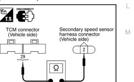
Ř T.S. Secondary speed sensor harness connector (Vehicle side) 2 1 3 V  $\oplus$ SCIA2346E
