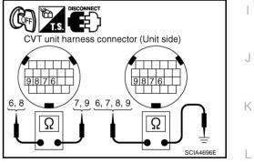
4. If NG, replace the transaxle assembly. Refer to CVT-224, "Removal and Installation" .
