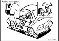
5. Engine start, apply foot brake, and place selector lever in "D" position.
