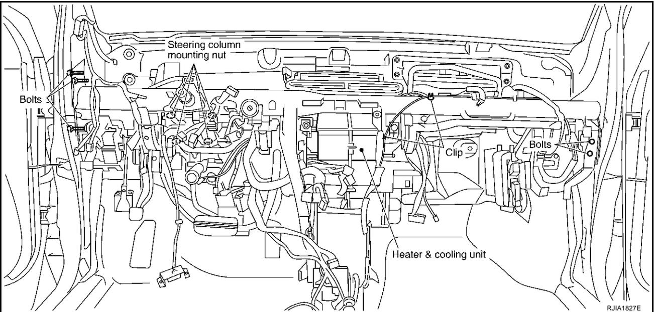
11. Remove mounting screws from heater & cooling unit.
