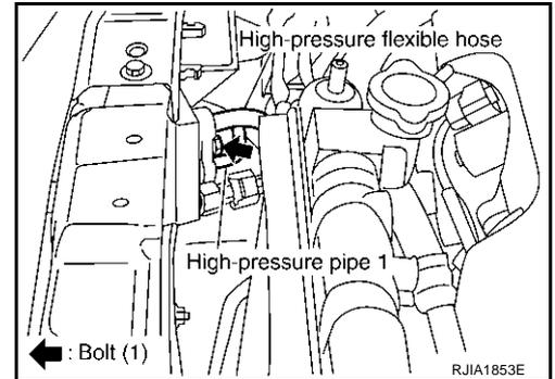
8. Remove mounting bolts for condenser, then remove condenser.
