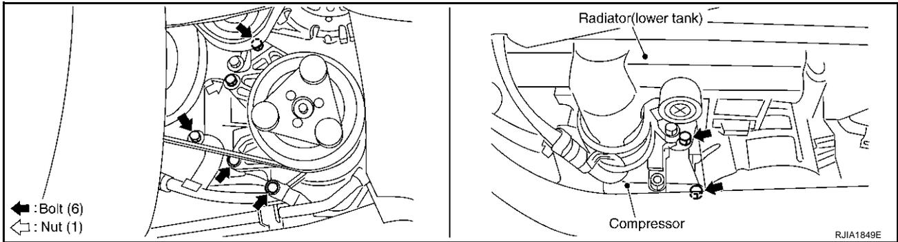
9. Remove compressor from passenger side of the vehicle.
