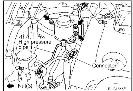
11. Disconnect cooling fan connector.
