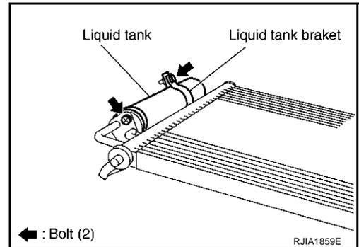
5. Lift liquid tank bracket upwards. Remove bracket from protruding part of condenser.
