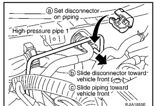
15. Remove the high-pressure pipe 1 mounting bolt, and then remove it.
