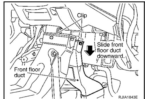
3. Peel back the floor carpet to a point where the floor duct is visible.
