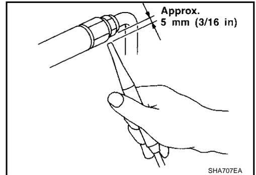
2. When testing, circle each fitting completely with probe.
