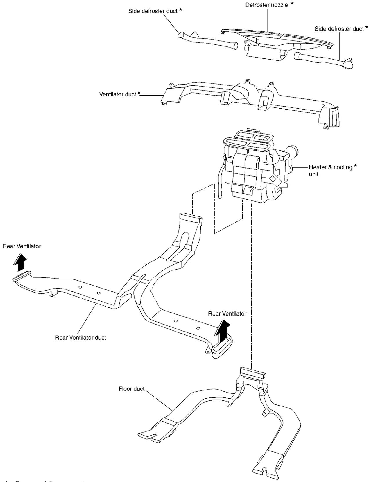
\* : For removal, it necessary to remove instrument panel.
