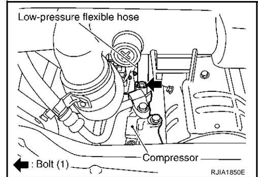
5. Remove mounting bolt from low-pressure flexible hose.
