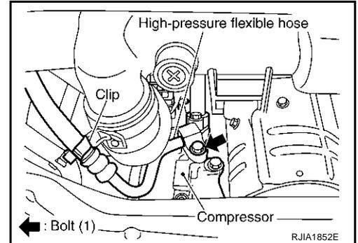
4. Remove the mounting nut for high-pressure flexible hose (Condenser side), and then remove the high-pressure flexible hose.
