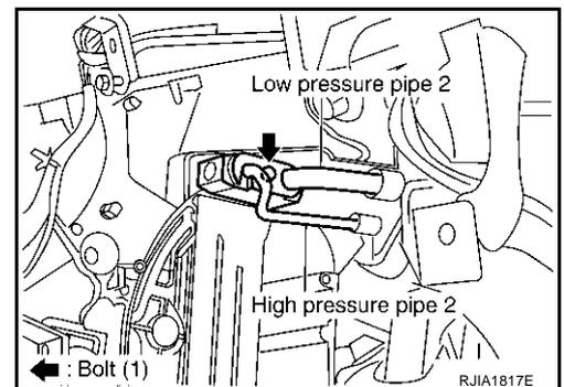
12. Slide the evaporator to passenger side, then remove the intake sensor.
