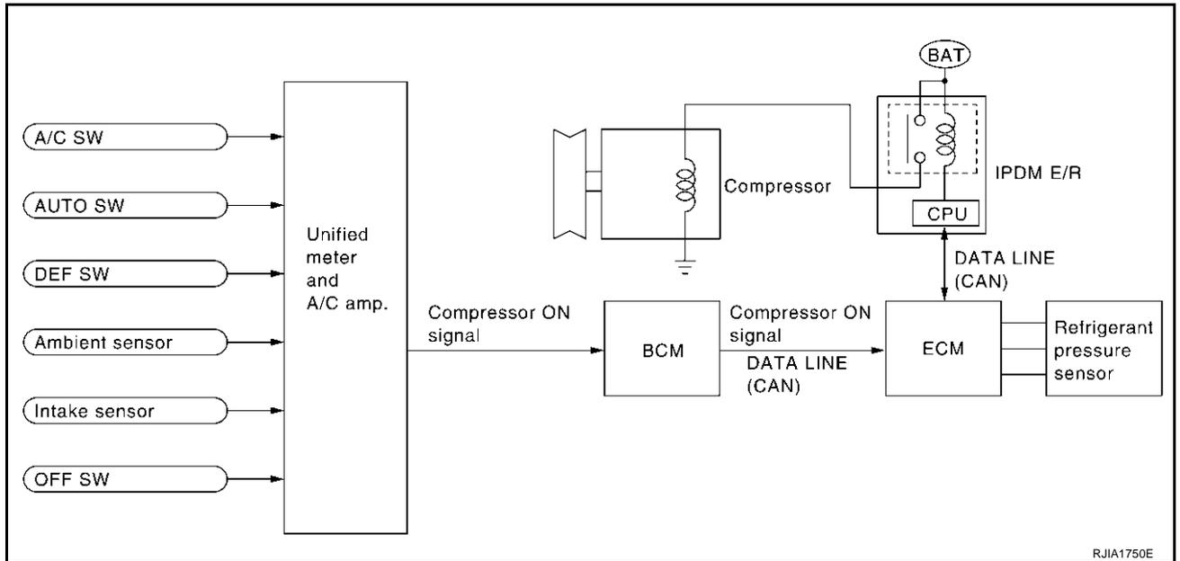
When A/C switch or DEF switch is pressed, unified meter and A/C amp. inputs compressor ON signal to BCM. BCM sends compressor ON signal to ECM, via CAN communication line.
