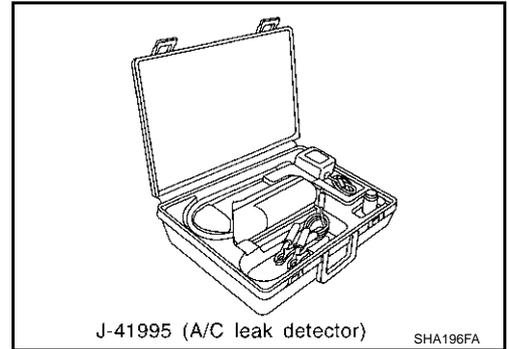
1. Position probe approximately 5 mm (3/16 in) away from point to be checked.
