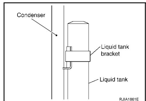
**Bolt mounting the liquid tank bracket (upper side)**
