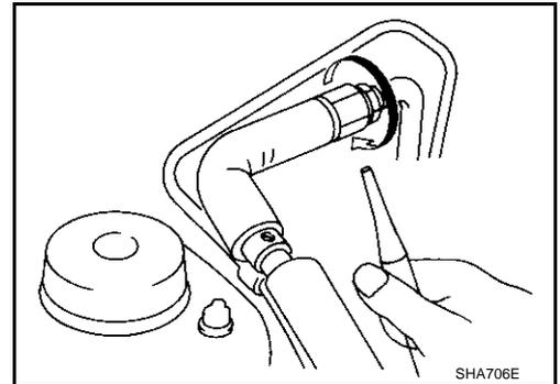
3. Move probe along component approximately 25 to 50 mm (1 to 2 in)/sec.
