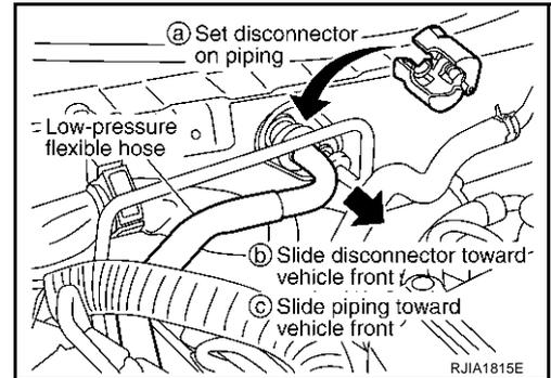
5. Disconnect two heater hoses from heater core.
