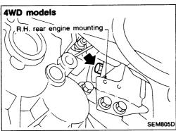
15. Remove R.H. rear engine mounting. (4WD models only)
