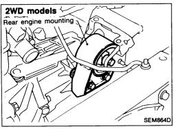
16. Remove rear engine mounting (engine left side) and then slowly lower transmission jack.
