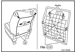
2. From the back of the seatback, press the headrest holder tabs at the base of the stay pipe to disengage. Then pull the headrest holder up to remove.
