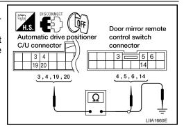
4. Check continuity between automatic drive positioner control unit connector M41 terminals 3, 4, 19, 20 and ground.
