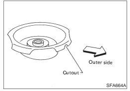
Install upper spring seat with its cutout facing the outer side of vehicle.
