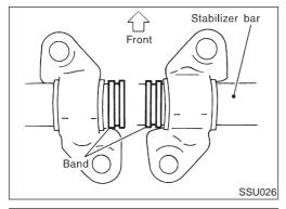
• When installing stabilizer, make sure that band and clamp face in their correct directions.
