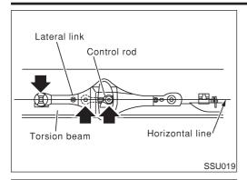
4. Using a transmission jack to lift the torsion beam, place lateral link and control rod horizontally against torsion beam. Tighten bolts and nuts to specified torque.
