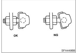
• Install stabilizer bar with ball joint socket properly placed.
