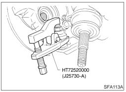
5. Separate lower ball joint stud from knuckle with suitable tool. Refer to AX-5, "FRONT AXLE — Wheel Hub and Knuckle".
