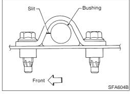
Make sure that slit in bushing is in the position shown in the figure.
