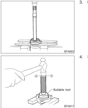
B. Press support bearing assembly off of drive shaft.
