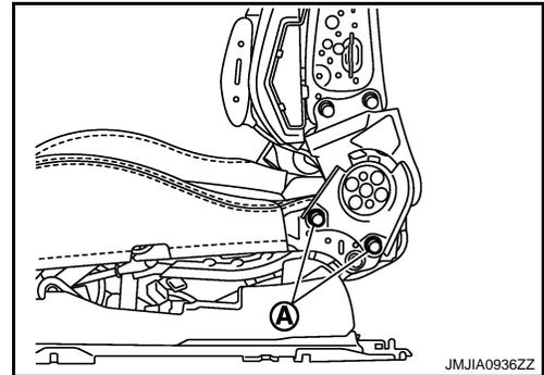
9. Remove the reclining device outer cover (front, rear).
