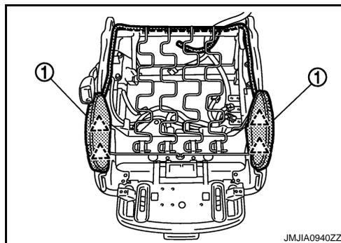
8. Remove the seat slide outer finisher.
