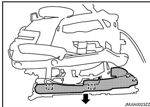
9. Remove the seat slide inner finisher.
