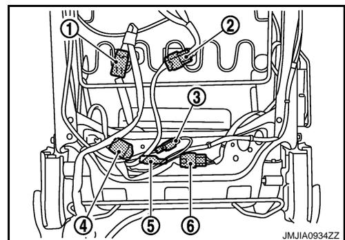
7. Remove the side support bag and unit.(Side support model only.)
