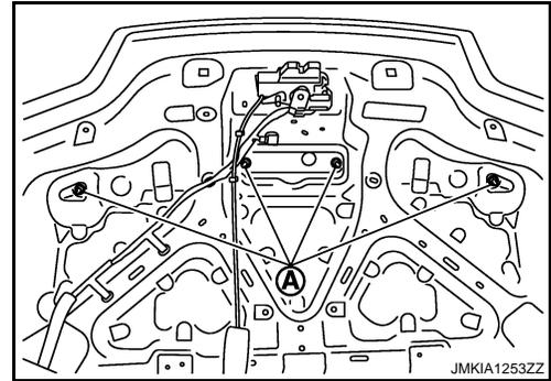
4. Apply protection tape (A) around outer circumference of trunk lid finisher outer (1).
