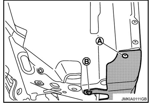
3. Remove screw (A) of center mud guard rear end.
