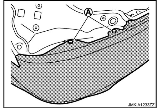
4. Remove bolts (A) of bumper fascia underside (LH/RH).
