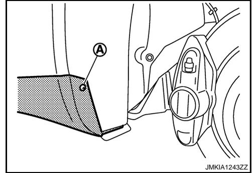
4. Remove screws of center mud guard underside.
