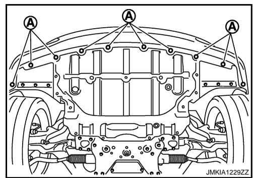
7. Remove fender protector (front) mounting bolts and clips, and then remove screw (A) of fixing bumper fascia left and right side.
