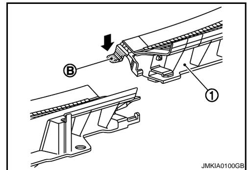
9. Remove the following parts after removing cowl top cover.
