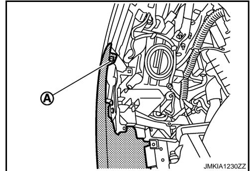
8. Pull the bumper fascia side toward the vehicle side to disengage the fitting of bumper side bracket and bumper fascia side.
