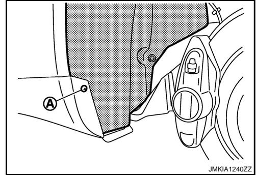
3. Remove rear wheel house protector mounting nuts and then remove rear wheel house protector.
