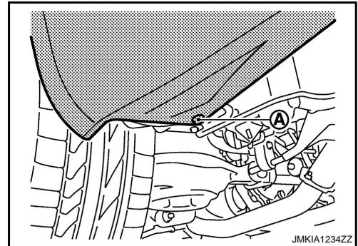
5. Remove screws (A) of bumper fascia front end upper (LH/RH).
