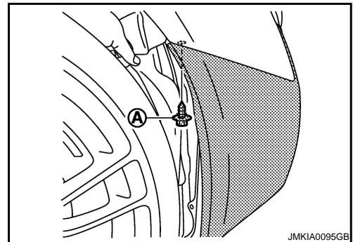
6. Remove clips of bumper fascia underside, and then pull out bumper fascia toward rear of vehicle.
