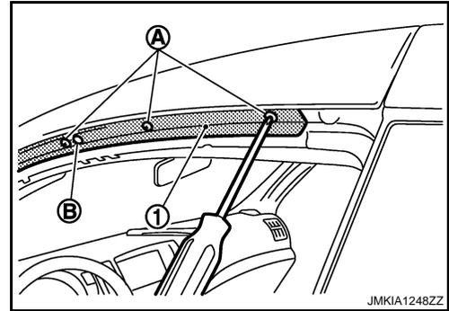
4. Remove front pillar finisher (1) fixing clips with remover tool (A).
