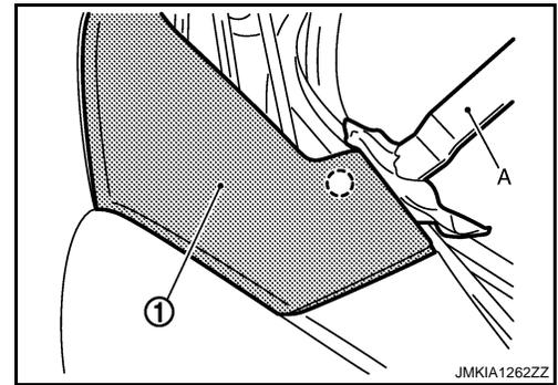
4. Disengage trunk drip cover (1) fixing metal clip using remover tool (A).
