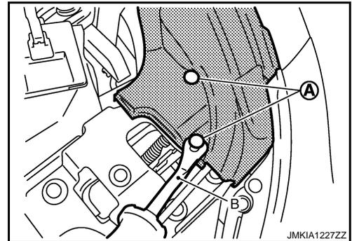
5. Remove bolts (A), and then remove bumper bracket (1).
