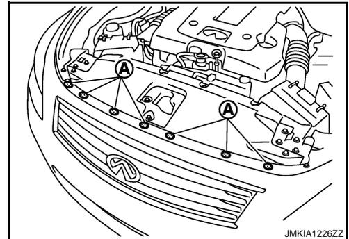
3. Remove radiator core support ornament. Refer to [DLK-214, "Removal and Installation"](#).
