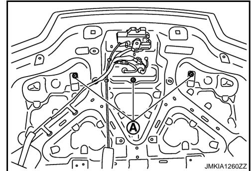
6. Release rear spoiler connection between trunk lid panel and rear spoiler, using a remover tool, and take off double-faced adhesive tape.
