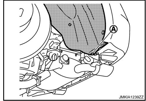
2. Remove screw (A) of rear wheel house protector located center mud guard.
