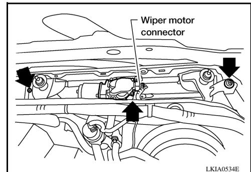
3. Remove wiper motor from wiper frame assembly.
