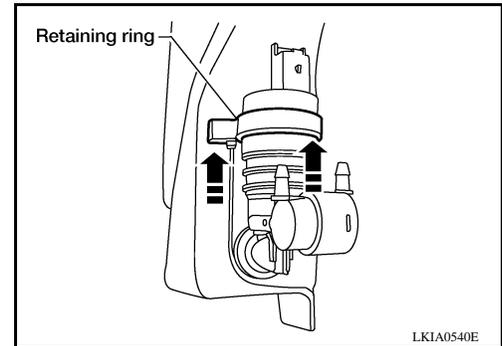
5. Remove washer motor from washer fluid reservoir.
