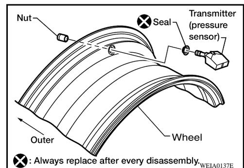
**Transmitter nut tightening torque : 7.7 N·m (0.79 kg·m, 68 in·lb)**
