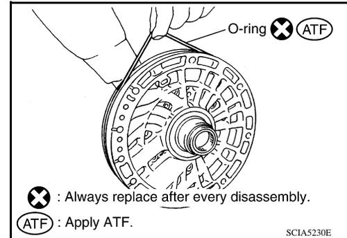
2. Install O-ring to oil pump housing.
