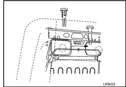
4. Remove the snap ring and the lumbar support lever knob.
