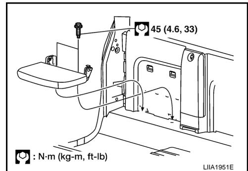
3. Remove the bolt, lift and remove the seatback assembly.
