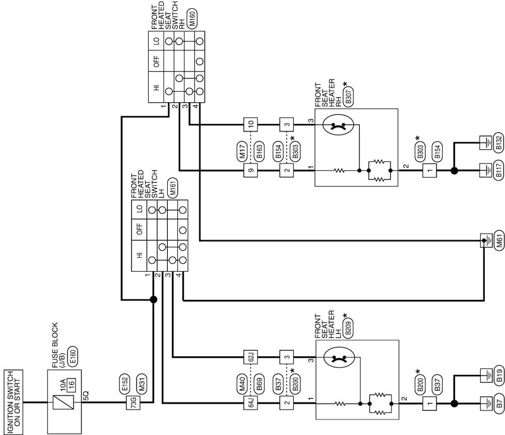
\* : THIS CONNECTORS IS NOT SHOWN IN "HARNES LAYOUT" OF PG SECTION
