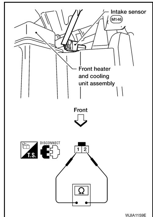
If NG, replace intake sensor. Refer to [VTL-8. "Removal and Installation"](#).
