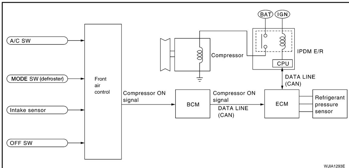
When the A/C switch is pressed, or the mode dial is turned to the DEF or D/F position, the front air control outputs a compressor ON signal to BCM.
