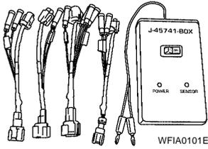
WFI0101E<br>Checking operation of ABS active wheel sensors |
