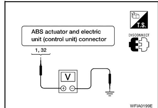
**3. CHECK ABS ACTUATOR AND ELECTRIC UNIT (CONTROL UNIT) GROUND CIRCUIT**
