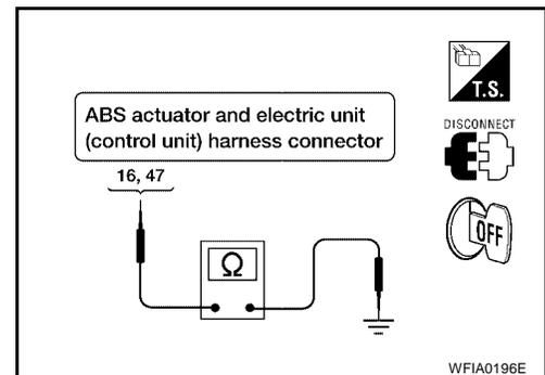
**ABS Warning Lamp Stays On When Ignition Switch Is Turned On** EFS005F6**1. CARRY OUT SELF-DIAGNOSIS**
