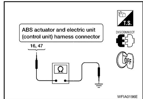
**ABS Warning Lamp Stays On When Ignition Switch Is Turned On** EFS005FD
