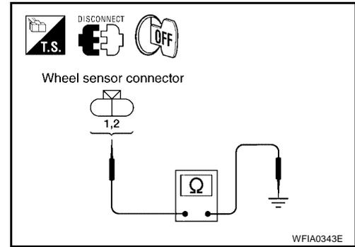
**6. CHECK WIRING HARNESS FOR OPEN CIRCUIT**
