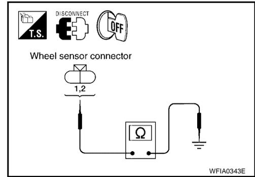
**6. CHECK WIRING HARNESS FOR OPEN CIRCUIT**
