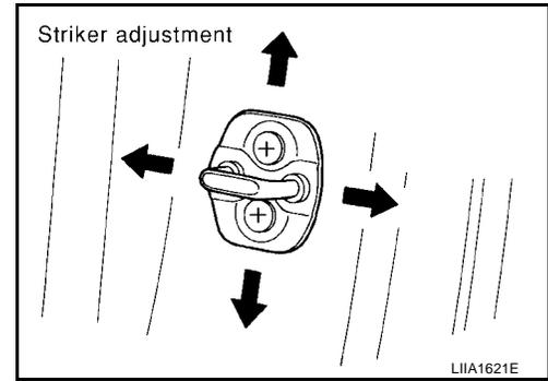
2. Remove the upper striker covers and adjust the striker so that it becomes parallel with the lock insertion direction.
