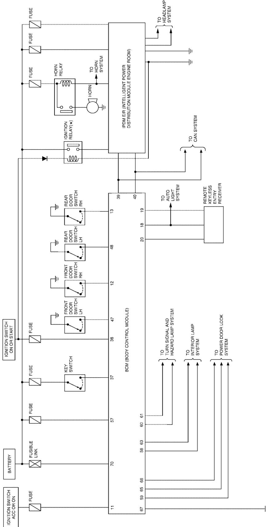
\*: THIS RELAY IS BUILT INTO THE IPDM E/R (INTELLIGENT POWER DISTRIBUTION MODULE ENGINE ROOM)
