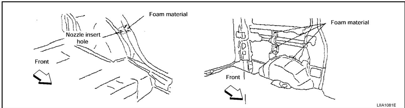
2. Fill procedures before installation of service part.
