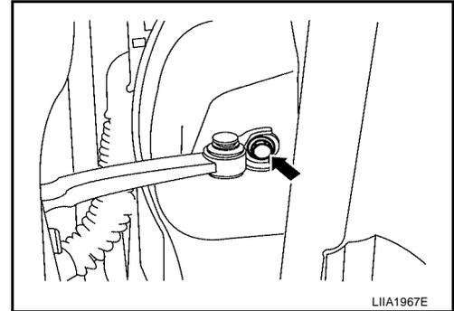
7. Remove the door-side hinge nuts and bolts, and remove the door assembly.
