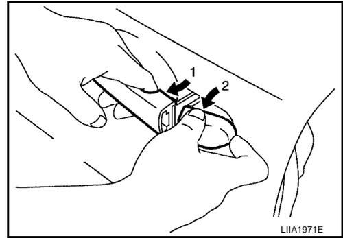
4. While pulling the outside handle, slide it toward the rear of vehicle to remove.
