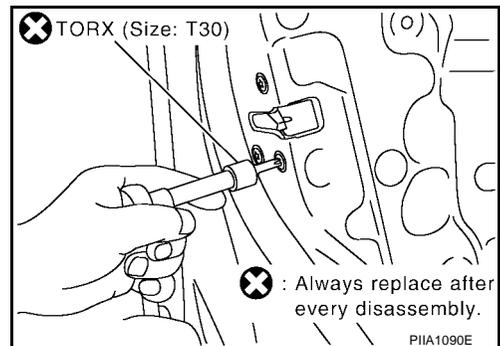
7. While pulling outside handle bracket, slide toward rear of vehicle to remove outside handle bracket and door lock assembly.
