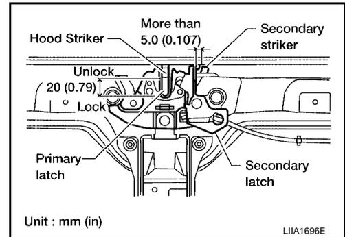
4. After adjusting hood lock, tighten the lock bolts to the specified torque.
