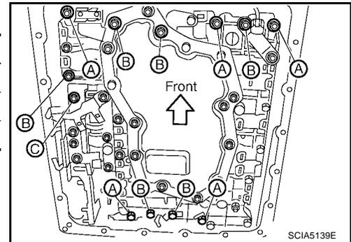
9. Tighten bolts 1, 2 and 3 temporarily to prevent dislocation. After that tighten them in order (1 → 2 → 3), and then tighten other bolts.
