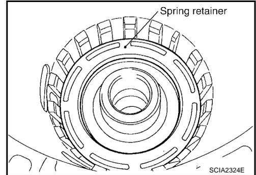
17. install snap ring in transmission case while compressing return spring using Tool.
