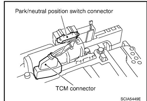
2. Install A/T assembly harness connector to control valve with TCM.
