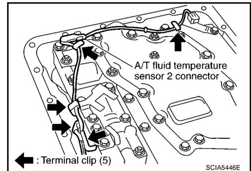
9. Straighten terminal clips to free revolution sensor harness.
