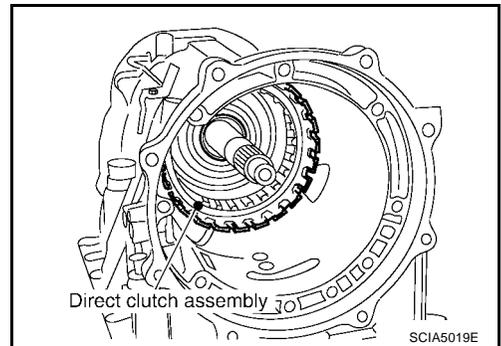
37. Install needle bearing in drum support.
