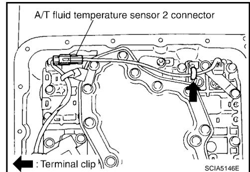
5. Remove A/T fluid temperature sensor 2 with bracket from control valve with TCM.
