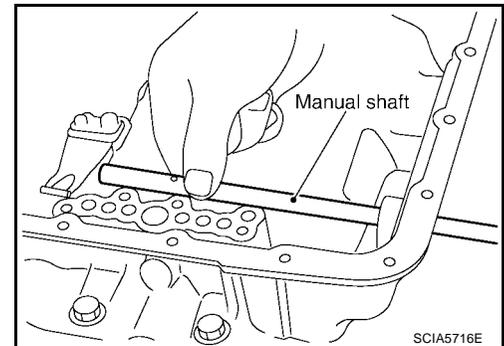
65. Remove manual shaft oil seals using suitable tool.
