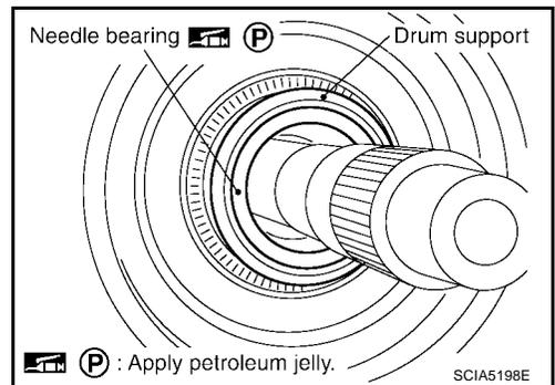
38. Install high and low reverse clutch assembly in direct clutch.
