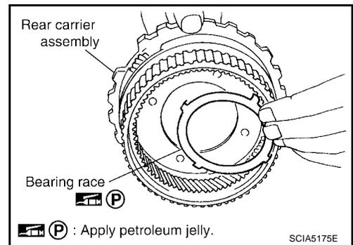
43. Install rear carrier assembly in direct clutch drum.
