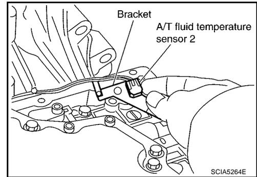
2. Install A/T fluid temperature sensor 2 (with bracket) in control valve with TCM. Tighten A/T fluid temperature sensor 2 bolt to the specified torque. Refer to [AT-233, "COMPONENTS"](#).
