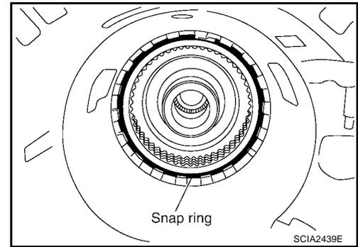
23. Measure clearance between retaining plate and snap ring. If not within specified clearance, select proper retaining plate.
