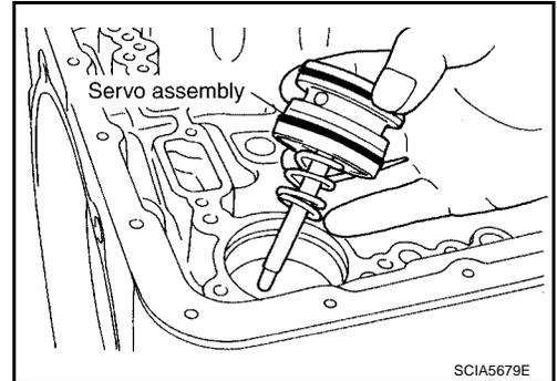
69. Remove return spring from servo assembly.
