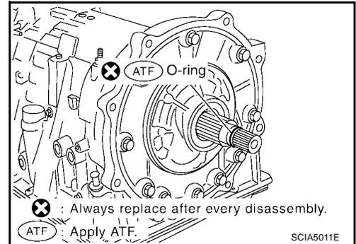
7. Install converter housing to transmission case.
