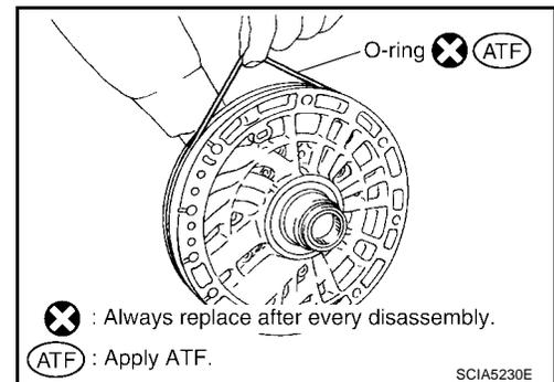
2. Install O-ring to oil pump housing.
