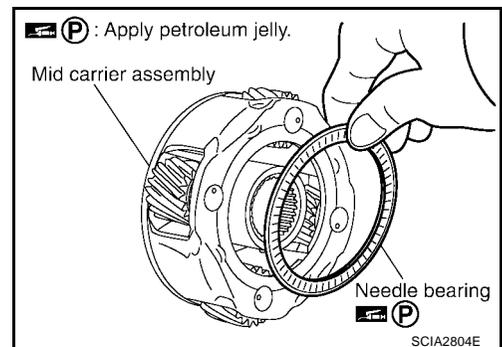
45. Install needle bearing (front side) to mid carrier assembly.
