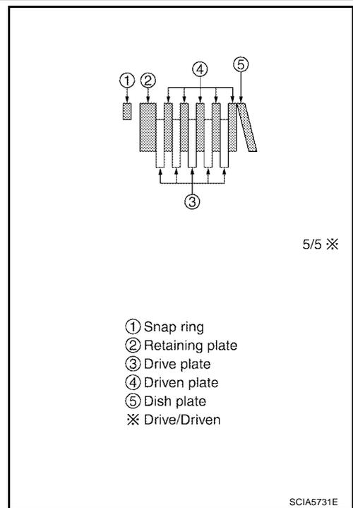
19. For VQ40DE engine install reverse brake drive plates (3), driven plates (4) and dish plates (5) in transmission case.
