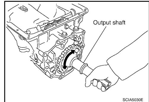
34. Install bearing race to output shaft.
