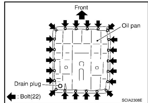
29. Check for foreign materials in oil pan to help determine cause of malfunction. If the A/T fluid is very dark, smells burned, or contains foreign particles, the friction material (clutches, band) may need replacement. A tacky film that will not wipe clean indicates varnish build up. Varnish can cause valves, servo, and clutches to stick and can inhibit pump pressure.
