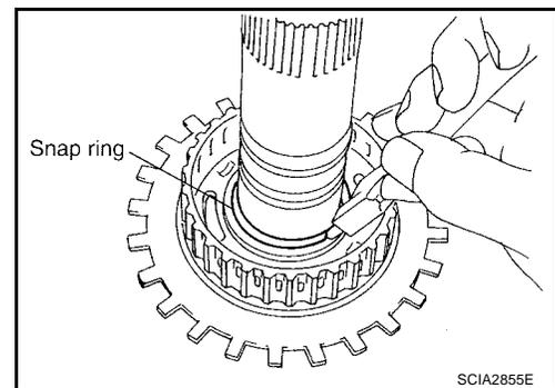
8. Check operation of 1st one-way clutch.
