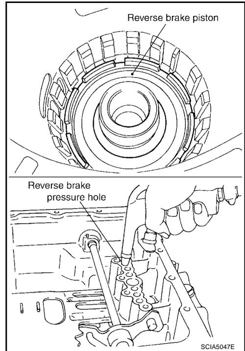
59. Remove D-rings from reverse brake piston.
