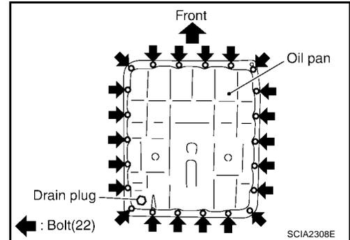
3. Check for foreign materials in oil pan to help determine cause of malfunction. If the A/T fluid is very dark, smells burned, or contains foreign particles, the friction material (clutches, band) may need replacement. A tacky film that will not wipe clean indicates varnish build up. Varnish can cause valves, servo, and clutches to stick and can inhibit pump pressure.
