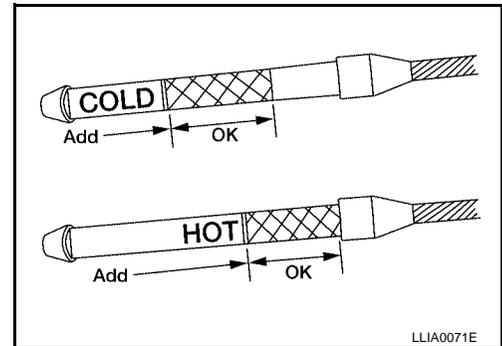
8. Install the ATF level gauge in the charging pipe and install the ATF level gauge bolt.
