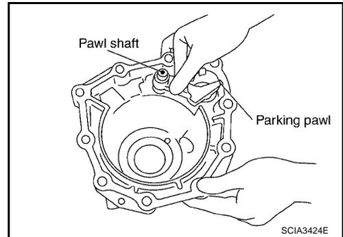
29. Install parking actuator support to rear extension (2WD models) or adapter case (4WD models).
