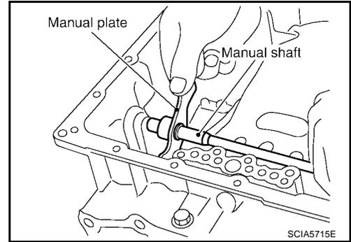
6. Install retaining pin into the manual plate and manual shaft.
