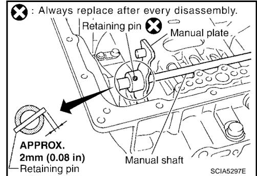
7. Install retaining pin into the transmission case and manual shaft.
