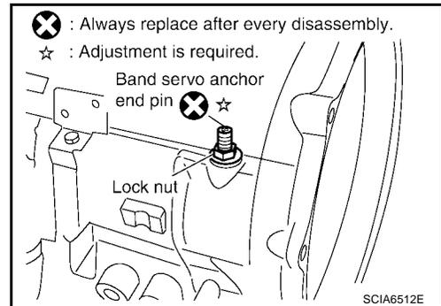
50. Install brake band in transmission case.
