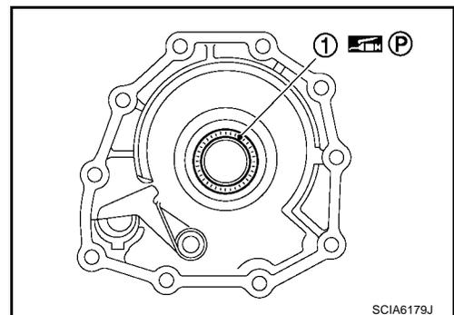
31. Install seal rings to output shaft.
