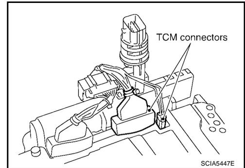
17. Remove A/T assembly harness connector from control valve with TCM using suitable tool.
