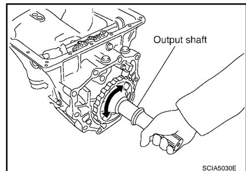
46. Remove parking gear from output shaft.
