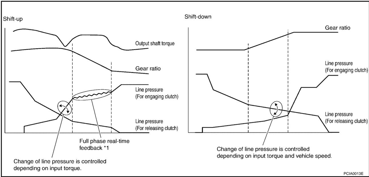
\*1: Full phase real-time feedback control monitors movement of gear ratio at gear change, and controls oil pressure at real-time to achieve the best gear ratio.
