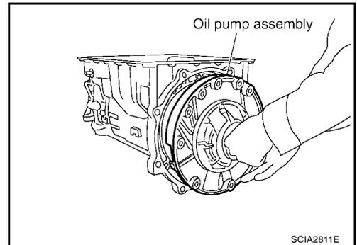
4. Apply recommended sealant (Genuine RTV Silicone Sealant or equivalent. Refer to [GI-48, "Recommended Chemical Products and Sealants"](#) .) to oil pump assembly as shown.
