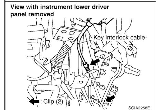
4. Insert interlock rod into adjuster holder.
