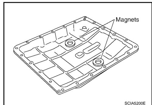
17. Install oil pan to transmission case.
