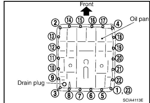
4. Install drain plug to oil pan.
