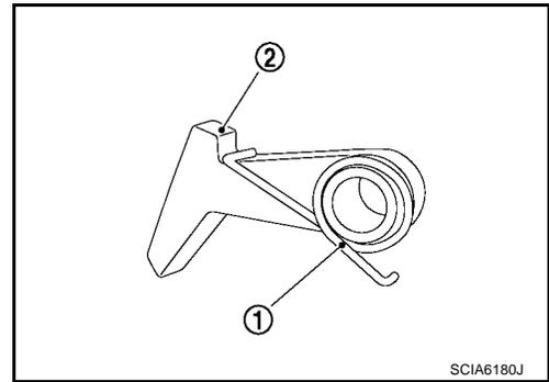
28. Install parking pawl (with return spring) and pawl shaft to rear extension (2WD models) or adapter case (4WD models).
