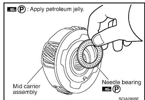
46. Install mid carrier assembly in rear carrier assembly.
