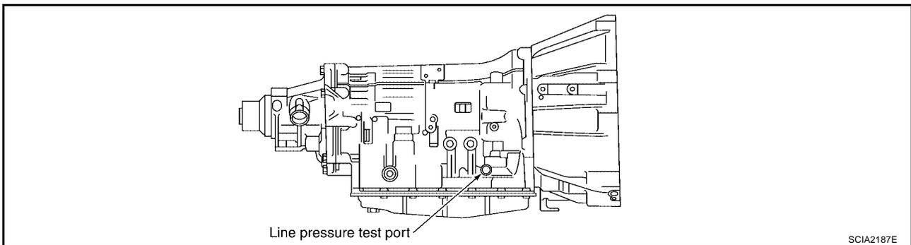
**Line Pressure Test Procedure**
