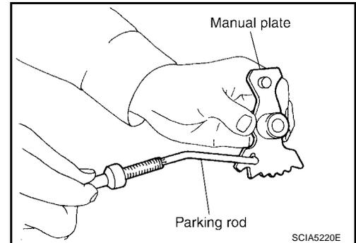
64. Remove manual shaft from transmission case.
