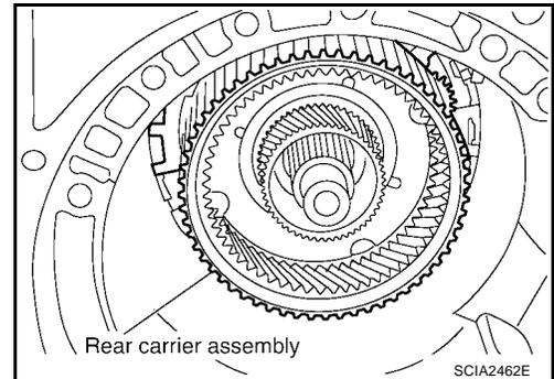
44. Install needle bearing (rear side) to mid carrier assembly.
