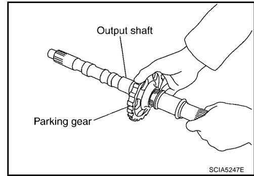
33. Install output shaft in transmission case.
