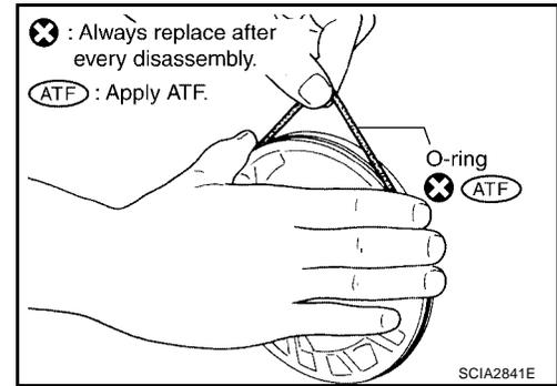
4. Remove O-ring from oil pump cover.
