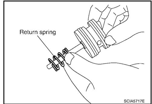
70. Remove O-rings from servo assembly.
