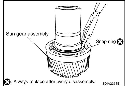
5. Install the sun gear assembly to the planetary carrier assembly.
