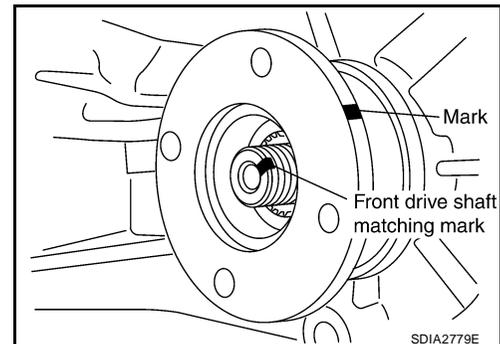
6. Remove the companion flange, using suitable tool.
