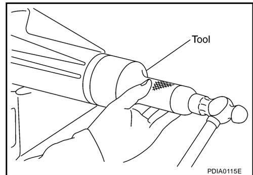
32. Apply petroleum jelly to the circumference of the new dust cover. Position the dust cover using the identification mark as shown.
