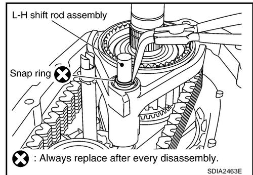
19. Install the snap ring to the mainshaft, using suitable tool.
