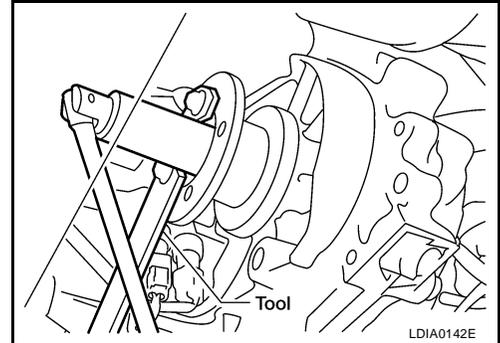
4. Put a matching mark on top of the front drive shaft in line with the mark on the companion flange.
