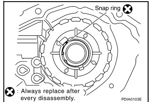
5. Install the internal gear with the groove facing up into the front case.
