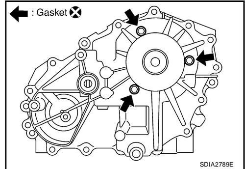
15. Remove the rear case bolts and harness bracket from the rear case.
