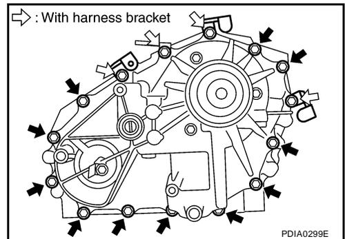
16. Separate the front case from the rear case. Then remove the rear case by prying it up, using suitable tool.
