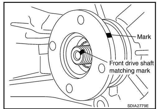
40. Install the companion flange self-lock nut. Tighten to the specified torque, using Tool. Refer to [TF-110, "COMPONENTS"](#).
