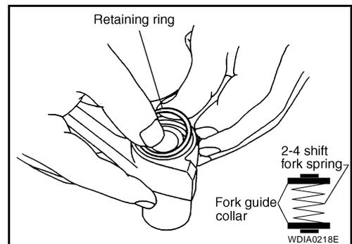
4. Install the 2-4 shift bracket to the L-H shift rod.
