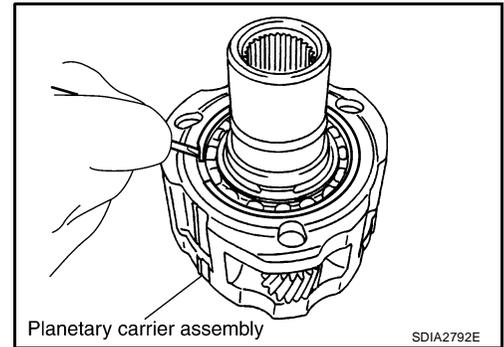
3. Remove the snap ring from the sun gear assembly, using suitable tool.
