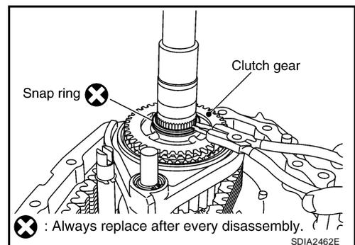
21. Install the snap ring to the mainshaft, using suitable tool.
