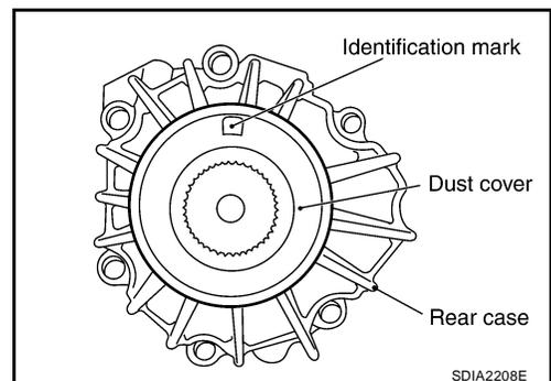
33. Install the dust cover to the rear case, using Tool.
