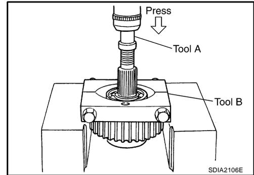
2. Remove the rear bearing, using Tools.
