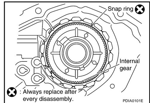
34. Remove the internal gear from the front case.
