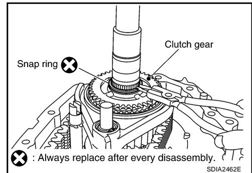
25. Remove the snap ring from the L-H shift rod assembly, using suitable tool.
