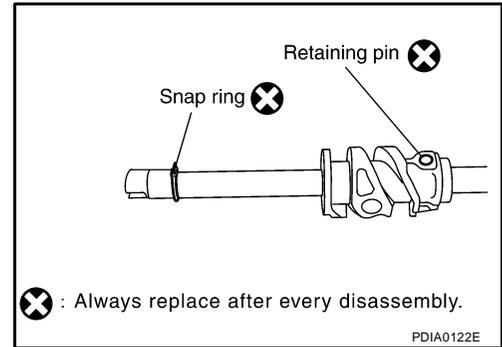
4. Remove the retaining pin from the L-H shift rod.
