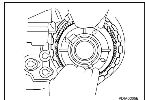
35. Remove the snap ring from the front case.
