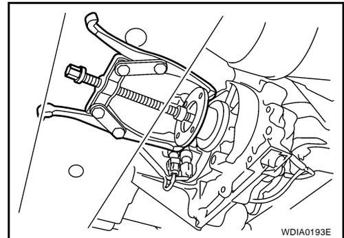
6. Remove the front oil seal from the front case, using Tool.
