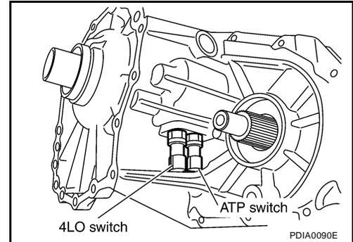
9. Remove the wait detection switch (gray) from the rear case.
