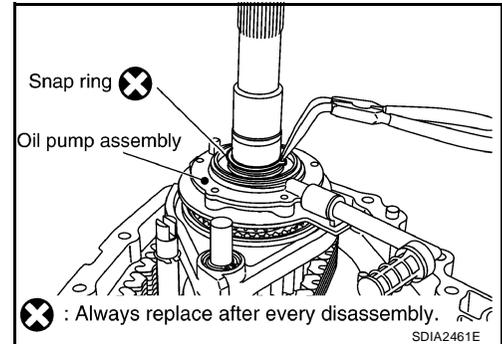
23. Remove the snap ring from the mainshaft, using suitable tool.
