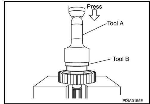
2. Install the front bearing, using Tools.
