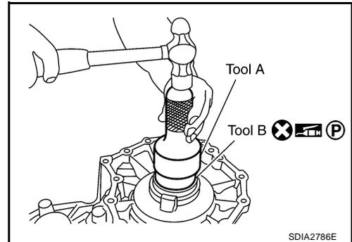
31. Install the rear oil seal until it is flush with the end face of the rear case, using Tool.
