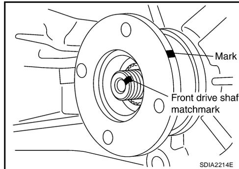
3. Install the self-lock nut and tighten to the specified torque, using Tool. Refer to [TF-110, "COMPONENTS"](#).
