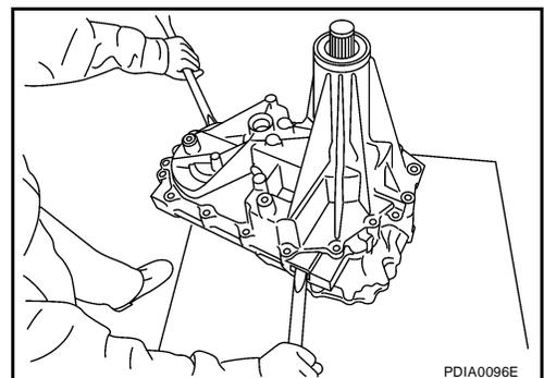
18. Remove the snap ring from the mainshaft, using suitable tool.
