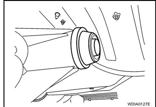
4. Remove the rear oil seal from the rear case, using Tool.
