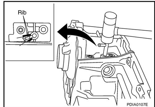
2. Install the baffle plate to the front case. Tighten the bolt to the specified torque. Refer to [TF-110, "COMPONENTS"](#).
