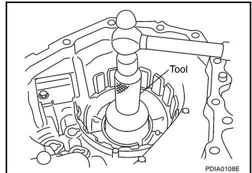
4. Install the snap ring to the front case.
