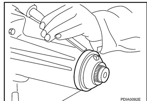
12. Remove the rear oil seal from the rear case, using Tool.
