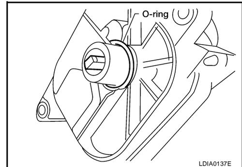
2. Install the transfer control device.
