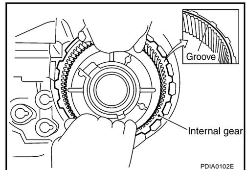
6. Install the snap ring to the front case.
