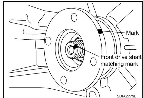
5. Remove the companion flange, using suitable tool.
