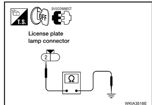
5. Check continuity between rear combination lamp (tail) harness connector and ground.
