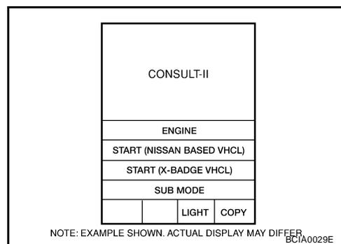
3. Touch "IPDM E/R" on "SELECT SYSTEM" screen. If "IPDM E/R" is not displayed, refer to [GI-40, "CONSULT-II Data Link Connector \(DLC\) Circuit"](#).
