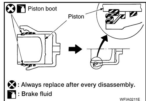
3. Insert into cylinder body by hand and insert piston boot piston-side lip into piston groove.
