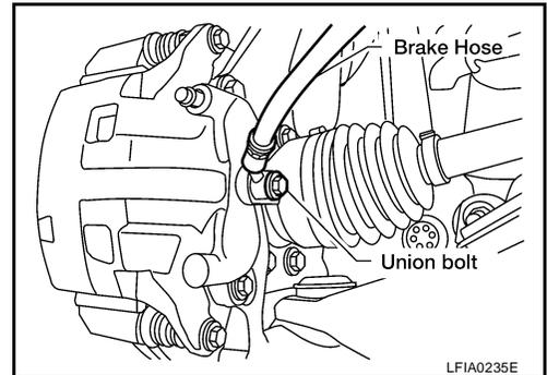
5. Refill new brake fluid and bleed air. Refer to [BR-10, "Bleeding Brake System"](#) .
