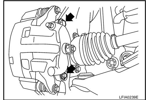
4. Install brake hose to brake caliper assembly, if removed, then tighten union bolt to the specified torque. Refer to [BR-22, "Components"](#) .
