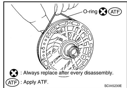
2. Install O-ring to oil pump housing.
