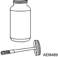
Lubricating oxygen sensor thread cleaning tool when reconditioning exhaust system threads.                                                                                                                                                                                            |
