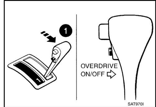
7. Release the overdrive control switch (the O/D OFF indicator lamp will begin to flash ON and OFF).
