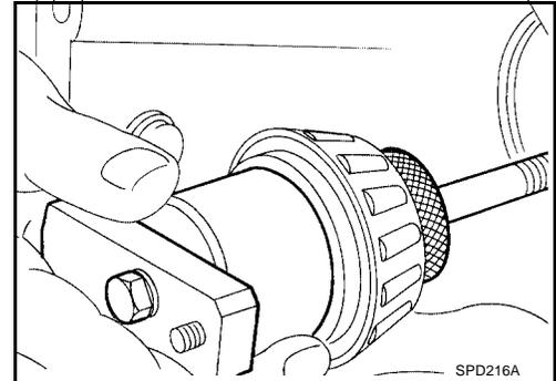
4. Install the J34309-2 gauge anvil with the front pinion bearing into the final drive housing and assemble it to the J34309-1 gauge screw. Make sure that the J34309-16 gauge plate will turn a full 360 degrees, and tighten the two sections by hand to set bearing preload.
