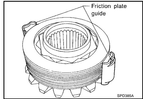
4. Install differential case B over side gear, discs, plates, spacer and friction plate guide assembly.
