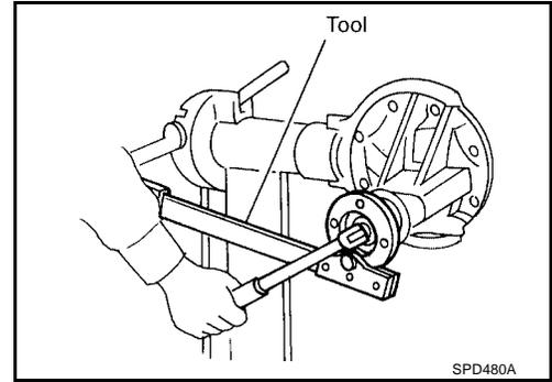
4. Take out drive pinion together with pinion rear bearing inner cone, drive pinion bearing spacer and pinion bearing adjusting shim.
