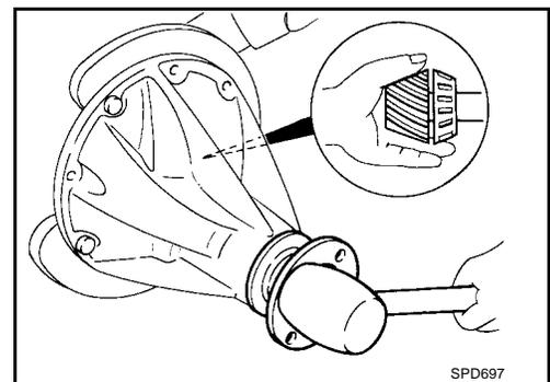
9. Tighten pinion nut until total preload is within specification.
