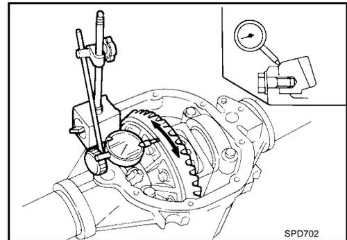
10. Check tooth contact. Refer to [RFD-29, "TOOTH CONTACT"](#).
