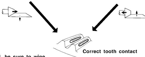
When adjustment is completed, be sure to wipe off completely the ferric oxide and oil or their equivalent.
