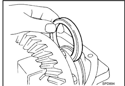
4. Use Tool to place original carrier side bearing adjusting shims on the carrier end, opposite the ring gear.
