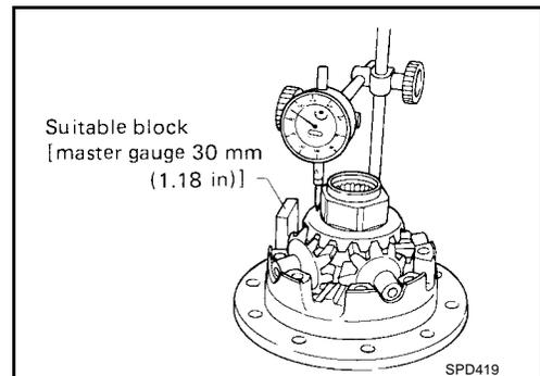
From the above equation, end play of 0.37 mm exceeds the specified range of 0.05 to 0.15 mm. Select suitable discs and plates to adjust correctly.
