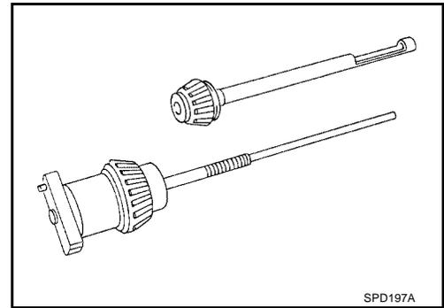
3. Place the pinion preload shim selector tool gauge screw assembly, J34309-1, with the pinion rear bearing inner cone installed, into the final drive housing.
