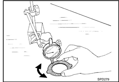
4. Measure frictional surfaces and projected portions of friction disc, friction plate, spring plate, and determine each part's differences to see if the specified wear limit has been exceeded.
