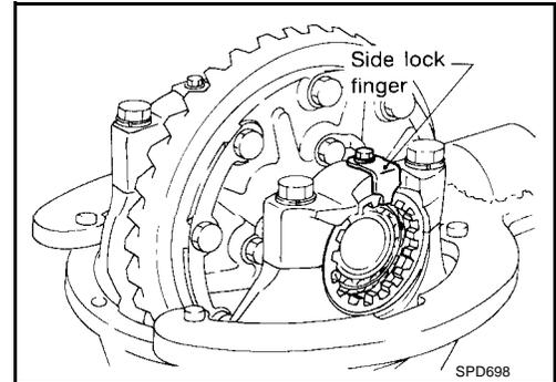
7. Check runout of ring gear with a dial indicator.
