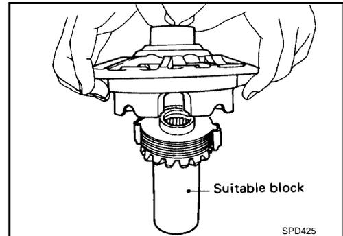
5. Install pinion mate gears and pinion mate thrust washers on pinion mate shaft, then install pinion mate shaft in differential case B.
