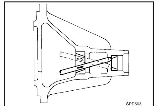
7. Remove pinion rear bearing inner cone and drive pinion adjusting washer.
