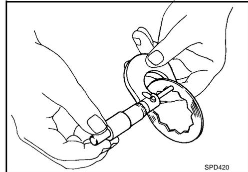
4. Measure the length of differential case contact surface to back side of side gear.
