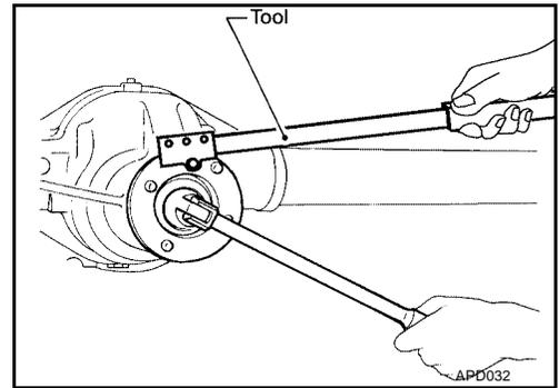
3. Remove companion flange using a suitable tool.
