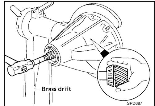
5. Remove front oil seal and pinion front bearing inner cone.
