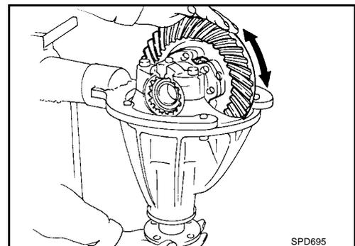
Usually the pattern will be correct if shims are correctly calculated and the backlash is correct. However, in rare cases, trial and error processes may be employed to obtain a correct pattern. The tooth pattern is the best indication of how well a differential has been set up.
