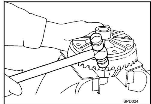
5. Punch off pinion mate shaft lock pin from differential case.
