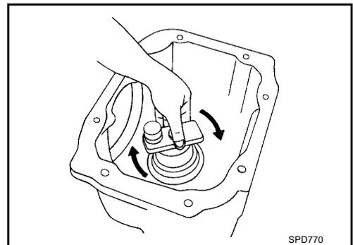
6. Measure the turning torque at the end of the J34309-2 gauge anvil using Tool.
