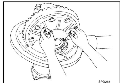
4. Tighten both right and left side bearing adjusters alternately and measure ring gear backlash and total preload at the same time. Adjust right and left side bearing adjusters by tightening them alternately so that proper ring gear backlash and total preload can be obtained.
