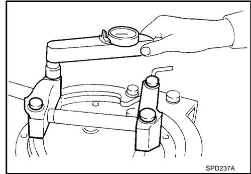
10. Select the correct standard pinion height adjusting washer thickness using a standard gauge of 2.5, 3.0, or 3.5 mm (0.098, 0.118, or 0.138 in) and the J34309-101 feeler gauge. Measure the distance between the J34309-12 "H233B" pinion height adapter and the arbor.
