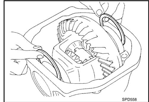
4. Drive in side bearing spacer with Tool.
