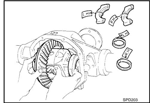
3. Insert left and right side bearing adjusting shims in place between side bearing outer races and differential carrier assembly.
