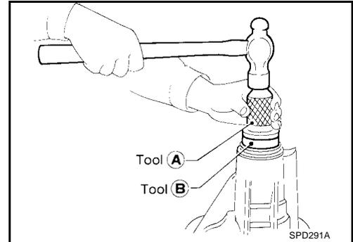
6. Install drive pinion bearing spacer, pinion bearing adjusting shim and drive pinion in gear carrier.
