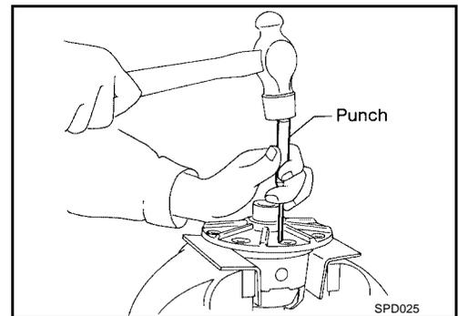
6. Disassemble the LH and RH differential case (4WD models).
