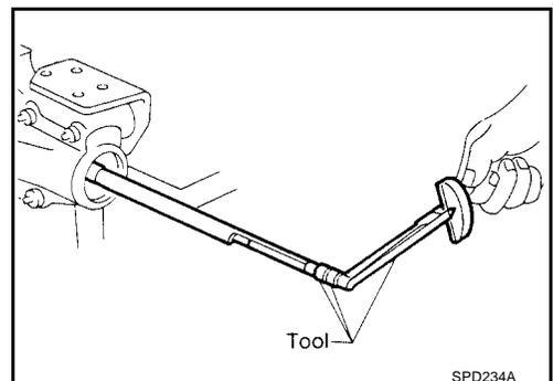
7. Place the J34309-11 pinion height adapter onto the gauge plate and tighten it by hand.
