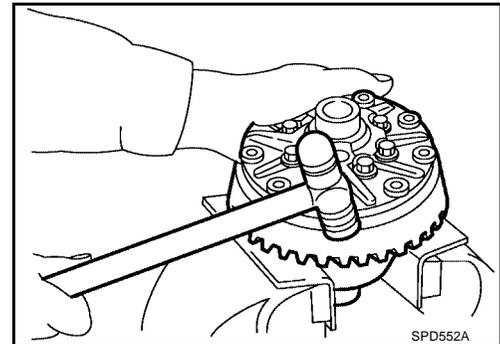
4. Remove couple bolts on differential cases A and B with a press.
