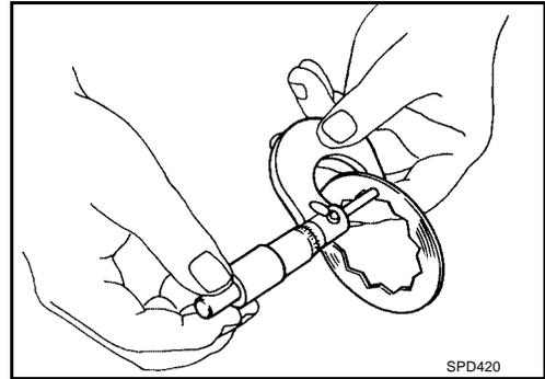
4. Measure values of the length of differential case contact surface to back side of side gear.
