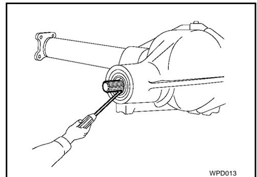
6. Apply multi-purpose grease to cavity at sealing lips of oil seal. Press front oil seal into carrier using Tool.
