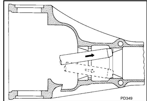
7. Remove pinion rear bearing inner cone and pinion height adjusting washer.
