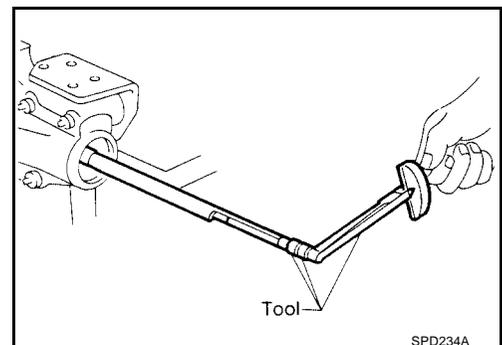
7. Place the J34309-12 "H233B" pinion height adapter onto the gauge plate and tighten it by hand.
