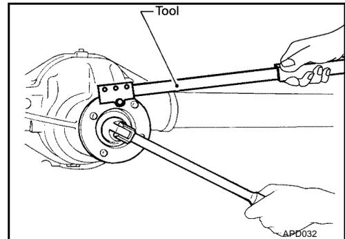
10. Tighten the pinion nut by very small degrees until the specified preload is achieved. When checking the preload, turn the drive pinion in both directions several times to set the bearing rollers.
