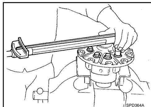
12. Install side bearing inner race.
