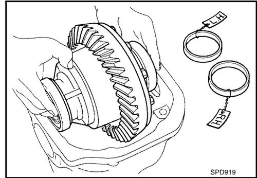
3. Put the side bearing adjusting shim in place.
