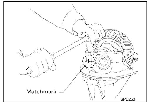
4. Remove side bearing adjuster using Tool.
