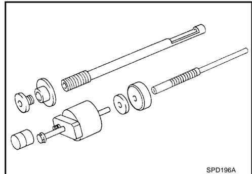
2. Assemble the pinion gear bearings into the pinion pre-load shim selector tool, J34309.
