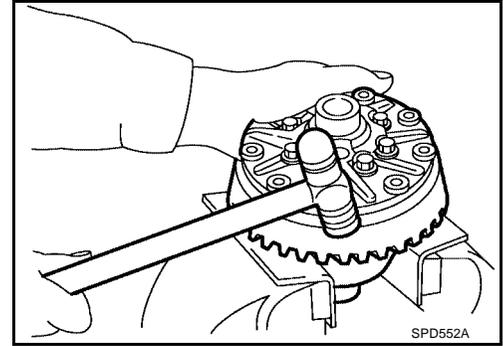
4. Remove differential case couple bolts with a press.
