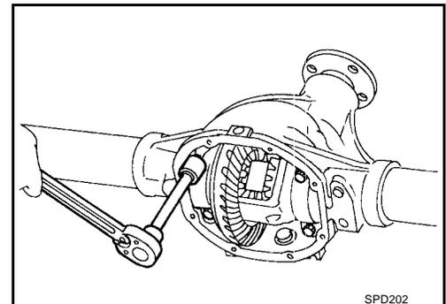
4. Remove differential case assembly with pry bar.
