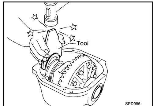
5. Install the side bearing caps in their correct locations using the matchmarks made during removal, and tighten the bearing cap bolts to specification.
