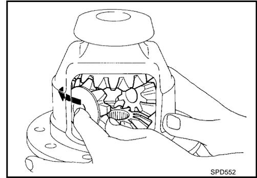
2. Fit pinion mate shaft to differential case so that it meets lock pin-holes.
