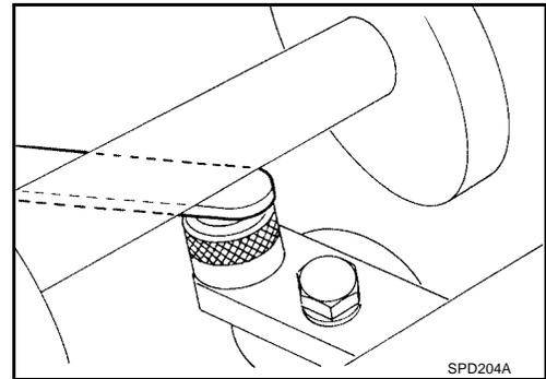
11. Write down the exact total measurement (the value of feeler gauge).
