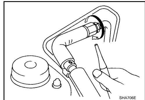
3. Move probe along component approximately 25 - 50 mm (1 - 2 in)/sec.
