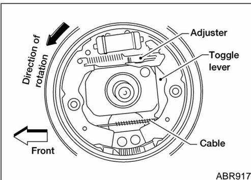
6. Check all parts are installed properly.
