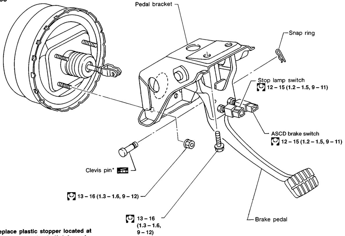
\* Replace plastic stopper located at the end of clevis pin if deformed or damaged.
