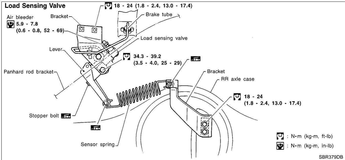
1. Tighten all flare nuts and mounting bolts.
