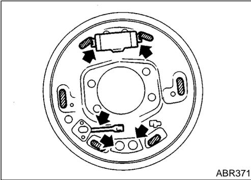
2. Apply brake grease to the contact areas shown at left.
