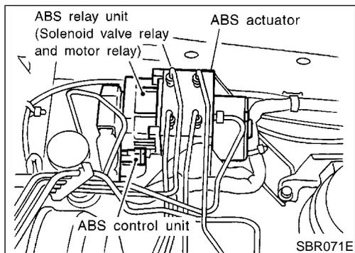
ABS ACTUATOR AND ELECTRIC UNIT (CONTROL UNIT)
