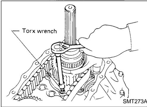
8. Remove bolts securing bearing retainer.
