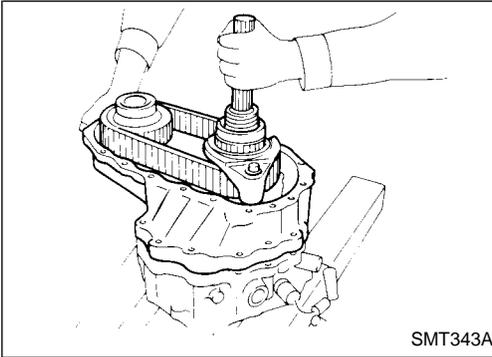
6. Apply sealant to mating surface of center case, then attach to front case and tighten bolts.
