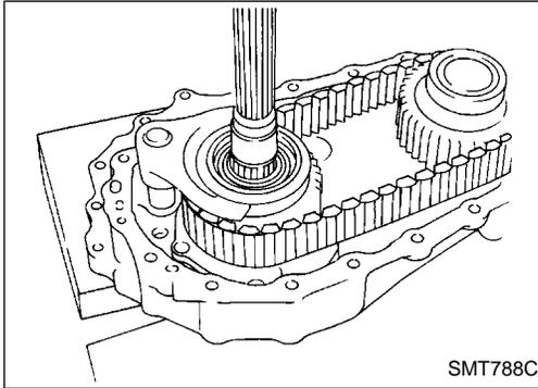
d. Make sure of the direction of the drive chain before removing it. (It must be installed in the same direction.)
