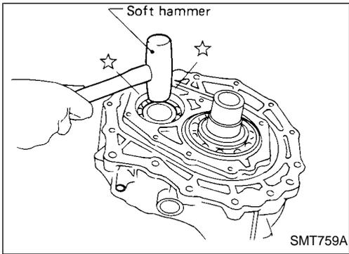
h. Remove counter gear by tapping lightly.
