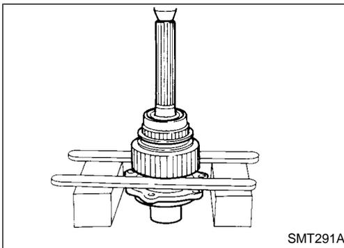
4. Use a press to remove front drive sprocket with mainshaft rear bearing and clutch gear together.
