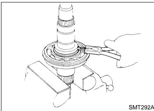
6. Remove bearing retainer, then remove snap ring.
