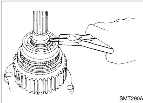
3. Remove snap ring and spacer.
