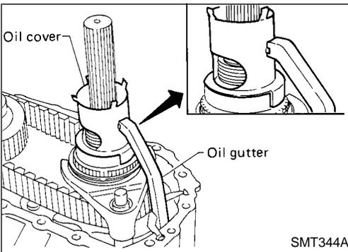
8. Install oil gutter and oil cover.
