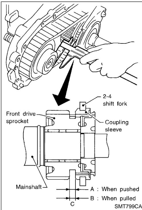
7. Using calipers, measure the difference between front drive sprocket and 2-4 coupling sleeve as outlined under Measuring method below. If it is outside specifications, check front drive sprocket, 2-4 coupling sleeve, clutch gear, 2-4 shift fork and 2-4 fork rod for abnormalities. Replace faulty part(s) as required.
