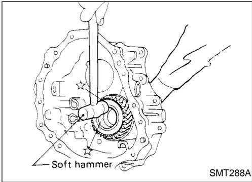
i. Remove main gear by tapping lightly.
