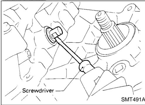
4. Remove shift shaft oil seal.
