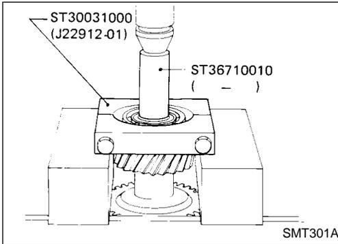
2. Press out counter gear rear bearing.
