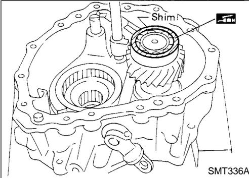
3. Place suitable shim with grease on counter gear rear bearing.
