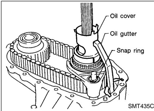
5. Remove oil cover and oil gutter.
