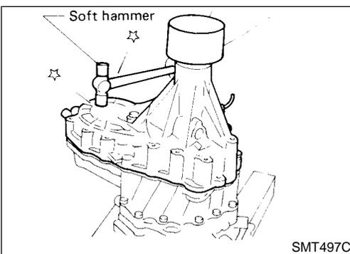
10. Apply sealant to mating surface of rear case, then attach it to center case and tighten bolts.
