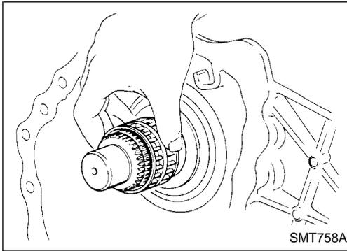
c. Remove needle bearing from main shaft.
