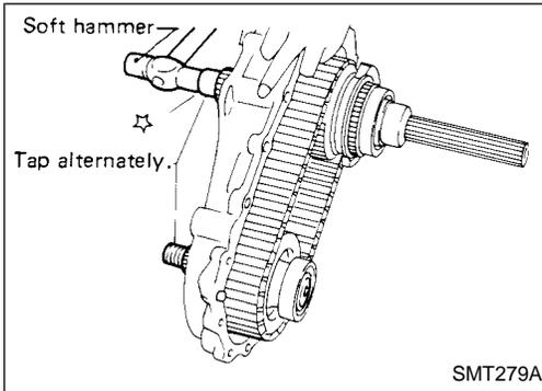
e. Remove mainshaft, front drive and drive chain as a set by tapping front end of mainshaft and front drive shaft alternately.
