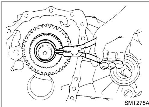
11. Disassemble center case assembly.
