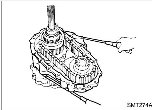
9. Remove bolts securing center case to front case, then separate center case from front case.
