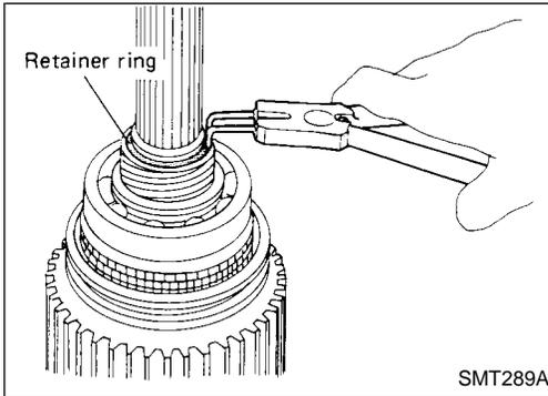
2. Remove retainer ring, speedometer drive gear and steel ball.
