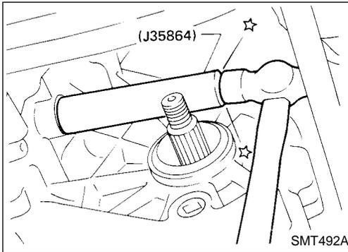
5. Install shift shaft oil seal.
