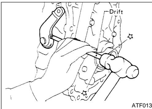
b. Remove lock pin from outer shift lever, then remove outer shift lever.
