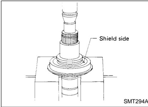
2. Select and install snap ring with proper thickness.
