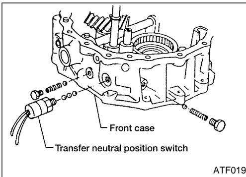
12. Disassemble front case assembly.
