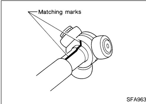
3. Move boot and slide joint housing toward wheel side, and put matching marks.
