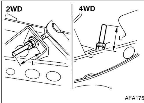
6. Tighten the adjusting nut so the torsion bar length corresponds with dimension "L" previously measured during torsion bar removal. Tighten the lock nut to specifications. If a new torsion bar spring or anchor arm is installed, tighten the adjusting nut to the dimension indicated in the figure at the left, then tighten the lock nut to specifications.
