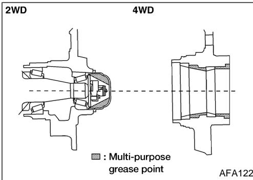
3. Pack multi-purpose grease in wheel hub and hub cap.
