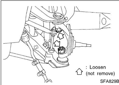
5. Separate knuckle spindle from ball joints.
