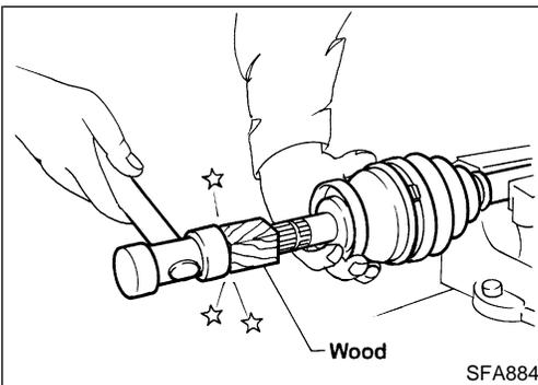
2. Set joint assembly onto drive shaft by lightly tapping it. Install joint assembly securely, ensuring that marks which were made during disassembly are properly aligned.
