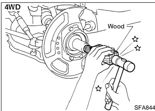
3. Separate drive shaft from knuckle spindle by slightly tapping drive shaft end. — 4WD —
