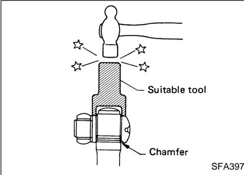
2. Install spider assembly securely, making sure marks are properly aligned.
