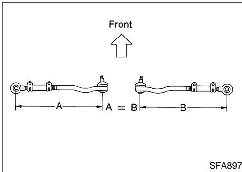
Make sure that the tie-rod bars are screwed into the tie-rod tube more than 35 mm (1.38 in).
