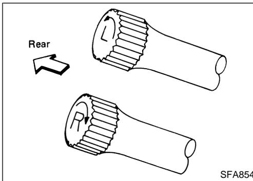
4. Install torsion bar spring. — 2WD —
