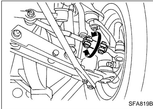
7. Adjust toe-in by varying the length of both steering tie-rods.
