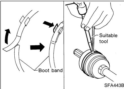
6. Lock new large boot band securely with a suitable tool, then lock new small boot band.
