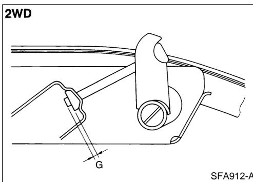
5. While aligning the anchor arm with the matching mark, install the anchor arm to the torsion bar spring.
