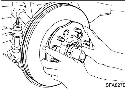
5. Remove wheel hub and wheel bearing.
