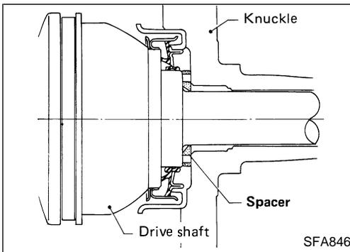
2. Install bearing spacer onto drive shaft.
