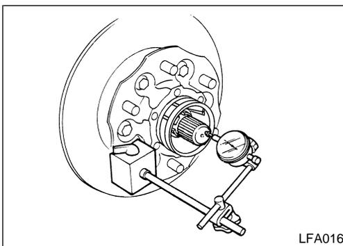
4. When installing drive shaft, adjust drive shaft axial end play by selecting a suitable snap ring.
