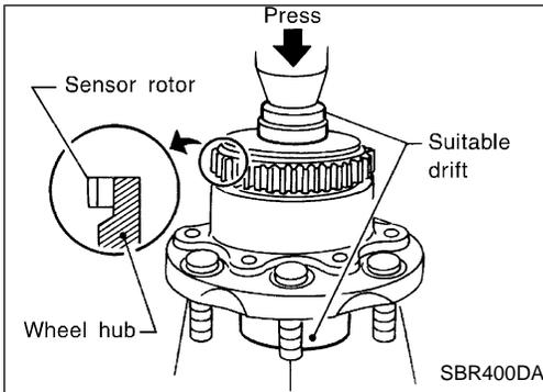
2. Install the sensor rotor using suitable drift and press. (Models with ABS)
