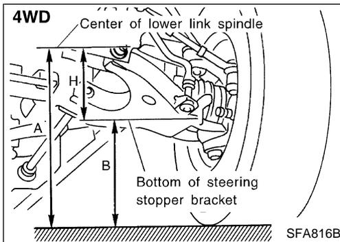
9. If height of the vehicle is not within allowable limit, adjust vehicle posture.
