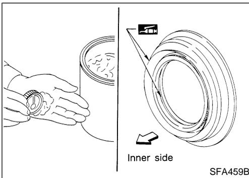
4. Apply multi-purpose grease to each bearing cone.
