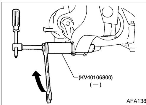
6. Remove front lower link fixing nut.
