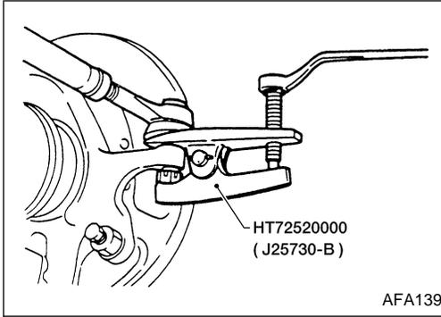
4. Separate tie-rod from knuckle spindle with Tool.
