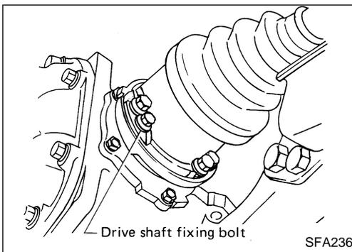
5. Remove bolts fixing drive shaft to final drive.
