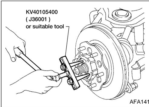
4. Remove wheel bearing lock nut.
