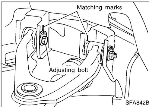
3. Put matching marks on adjusting bolts and remove adjusting bolts.
