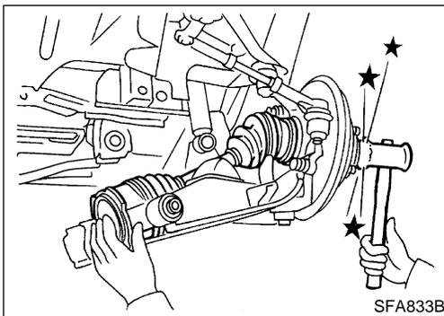
6. Separate drive shaft from knuckle spindle by slightly tapping end of drive shaft.
