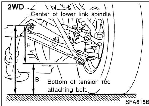
7. Bounce vehicle with tires on ground (Unladen) to eliminate friction of suspension.
