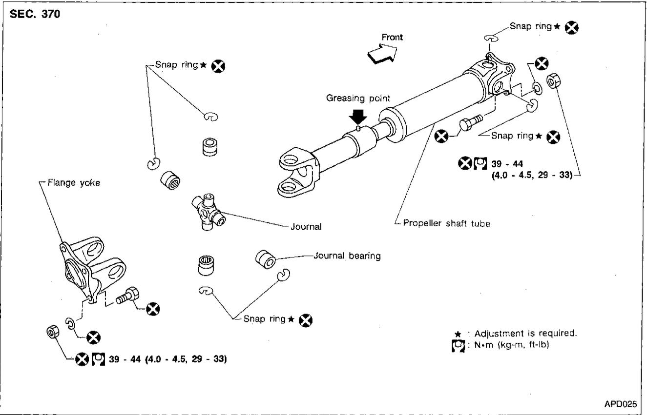
Rear propeller shaft (Model 3S1310)
