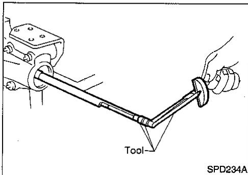
6. Measure the turning torque at the end of the J34309-2 gauge anvil using torque wrench J25765A.
