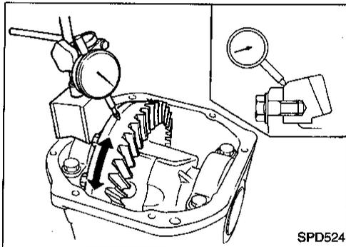
19. Check runout of ring gear with a dial indicator.
