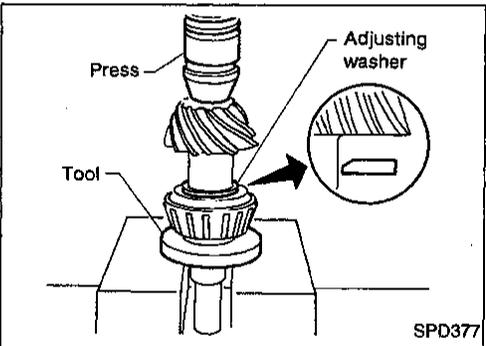
2. Select drive pinion height adjusting washer and pinion bearing adjusting washer. Refer to ADJUSTMENT (PD-24).
