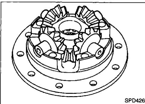
6. Install pinion mate gears and pinion shaft to differential case B.
