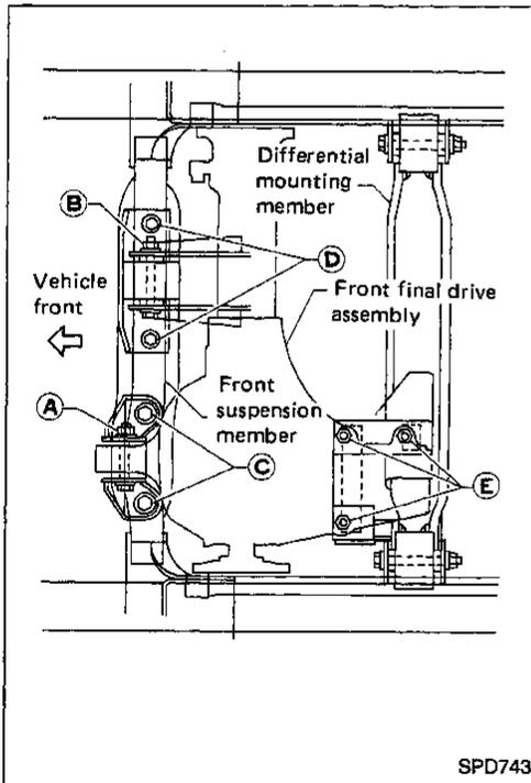
2. Tighten front final drive securing bolts and nuts by following the procedure to prevent drive train vibration.
