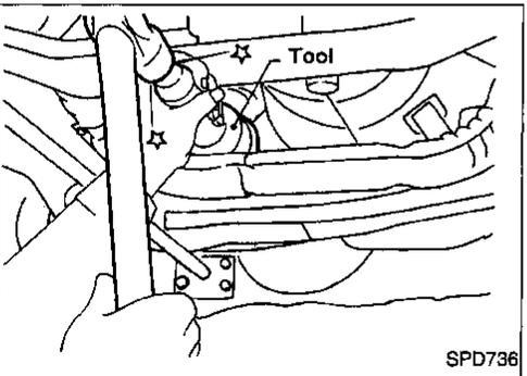
5. Apply multi-purpose grease to cavity at sealing lips of oil seal.
