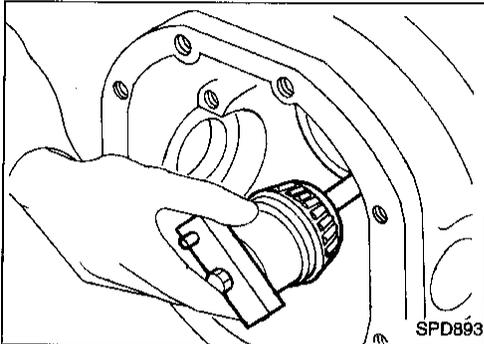
3. Place the pinion preload shim selector Tool, J34309-1, gauge screw assembly with the pinion rear bearing inner cone installed into the final drive housing.
