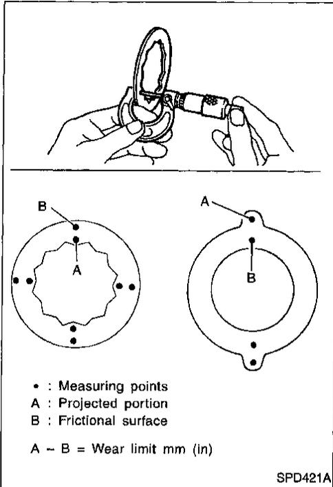
4. Measure frictional surfaces and projected portions of friction discs, plates, spring disc and plate.
