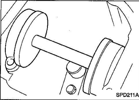
11. Now, position the side bearing discs, J25269-4, and arbor firmly into the side bearing bores.
