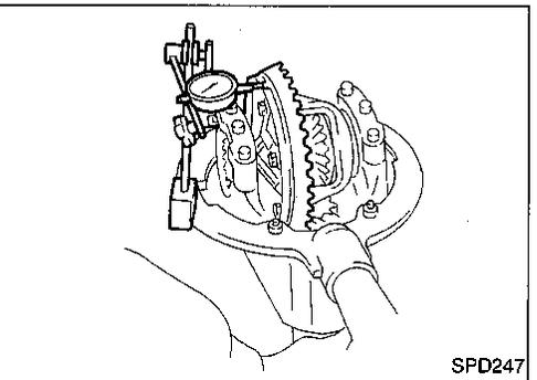
16. Check runout of ring gear with a dial indicator.
