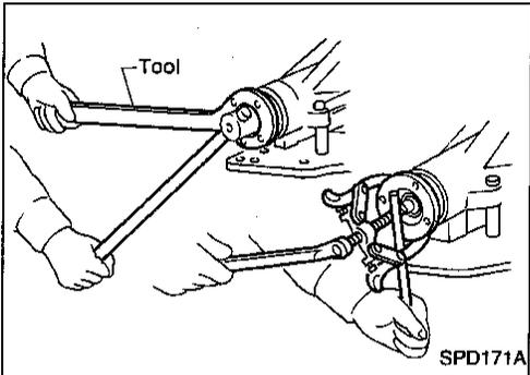
7. Loosen drive pinion nut.
