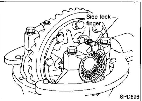
14. Tighten side bearing cap bolts.
