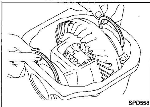
12. Insert left and right side bearing adjusting washers in place between side bearings and final drive housing.
