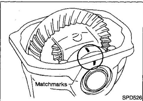
14. Align mark on bearing cap with that on final drive housing and install bearing cap on final drive housing.
