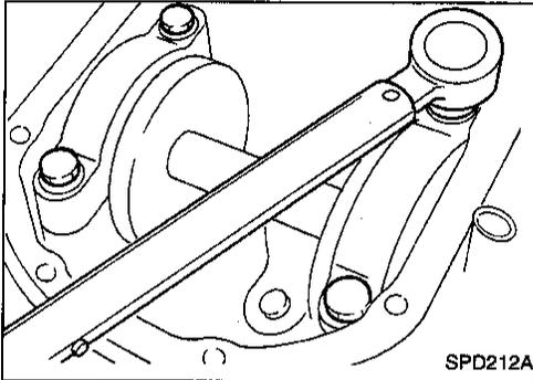
12. Install the side bearing caps and tighten the cap bolts.
