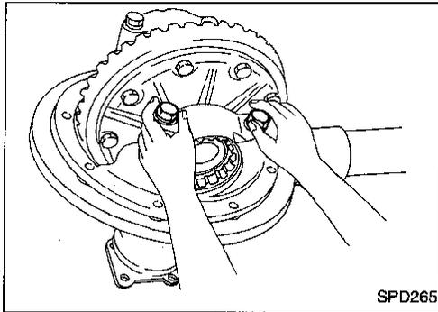
12. Align mark on bearing cap with that on gear carrier and install bearing cap on gear carrier.
