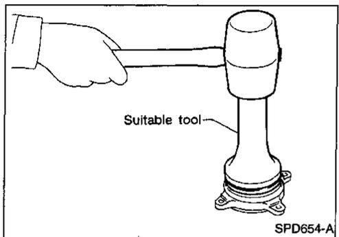
2. Install extension tube retainer, rear axle bearing and rear axle shaft bearing collar on differential side shaft.
