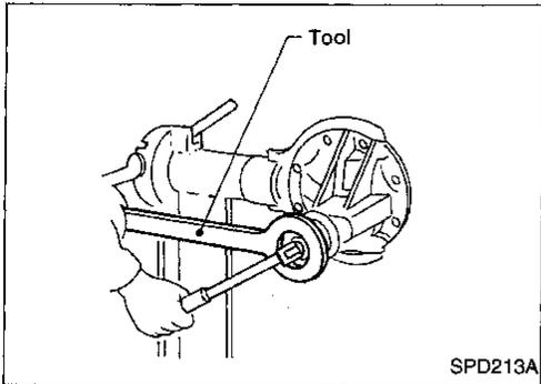
6. Remove drive pinion nut with Tool.
