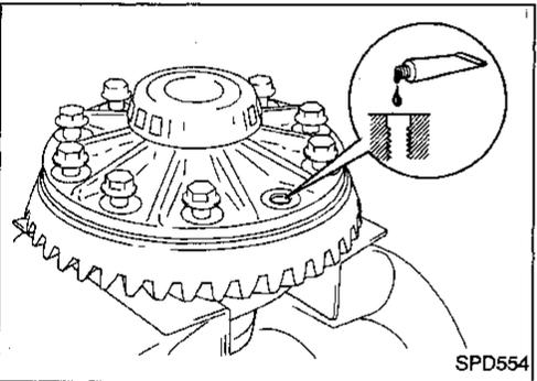
6. Install differential case assembly on ring gear.
