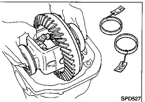
10. Select side bearing adjusting washer. Refer to ADJUSTMENT (PD-23).
