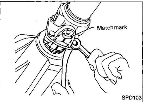
2. Remove propeller shaft.
