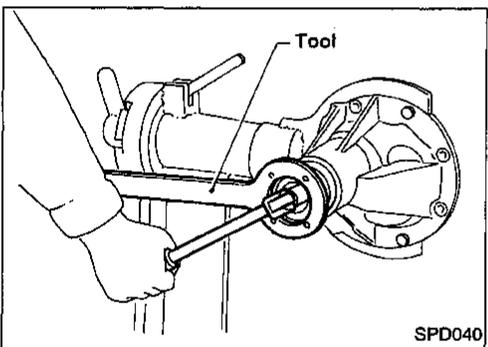
8. Tighten pinion nut to the specified torque.
