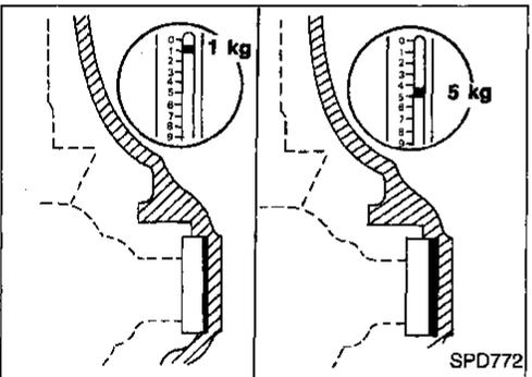
8. If the carrier turning torque is not within the specification range, increase or decrease the total thickness of the side bearing adjusting washers until the turning torque is correct. If the turning torque is less than the specified range, install washers of greater thickness; if the turning torque is greater than the specification, install thinner washers. See the SDS section for washer dimensions and part numbers.
