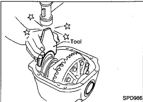
1. Make sure all parts are clean and that the bearings are well lubricated with light oil or "DEXRON™" type automatic transmission fluid.
