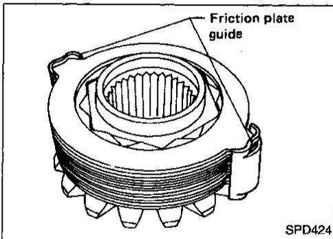
4. Install friction plate guides.
