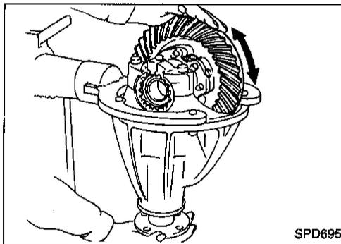
3. Hold companion flange steady and rotate the ring gear in both directions.
