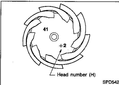
15. Correct the pinion height washer size by referring to the "pinion head number".
