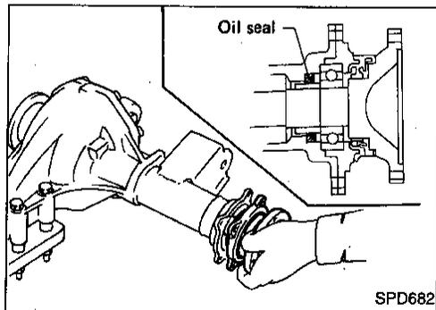
22. Install differential side shaft assembly.
