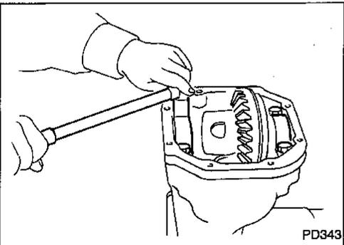
6. Remove differential case assembly with a pry bar.
